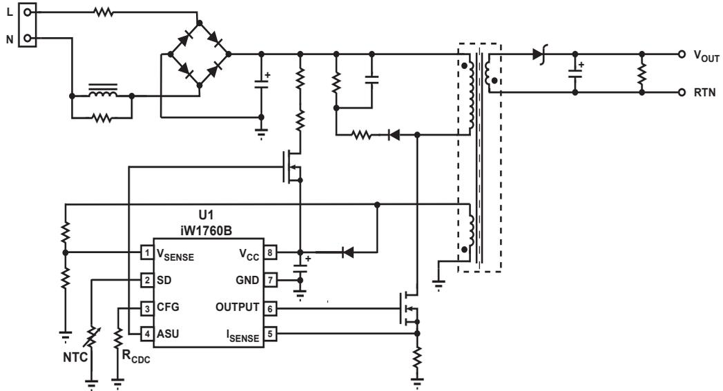
**Figure 3.1 : iW1760B Typical Application Circuit
