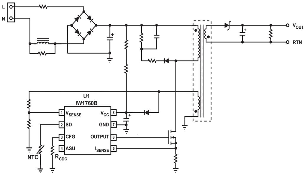
**Figure 3.2 : iW1760B Typical Application Circuit
