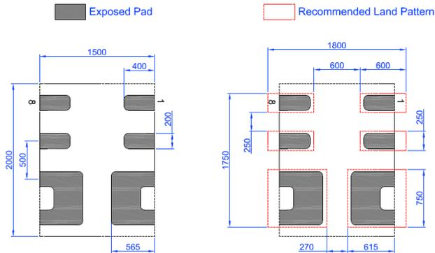
**Figure 2. SLG59M1456V Package Dimensions and Recommended Land Pattern**
