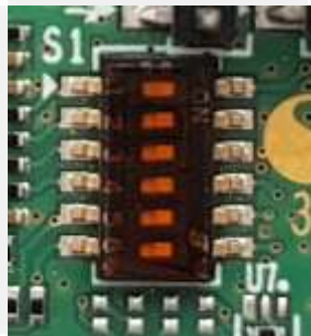
Figure 16: Debugging DIP switch
