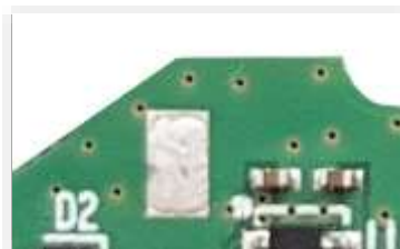
Figure 24: GND Support Point (Must Be Placed by Users)
