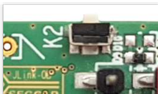
Figure 12: RESET Push Button (K2)
