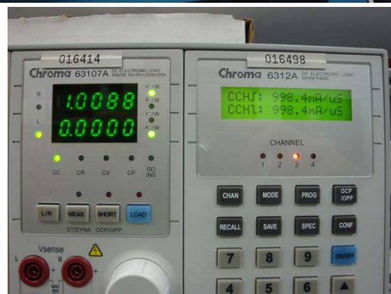
FIGURE 1. TYPICAL ELECTRONIC LOAD SETUP
