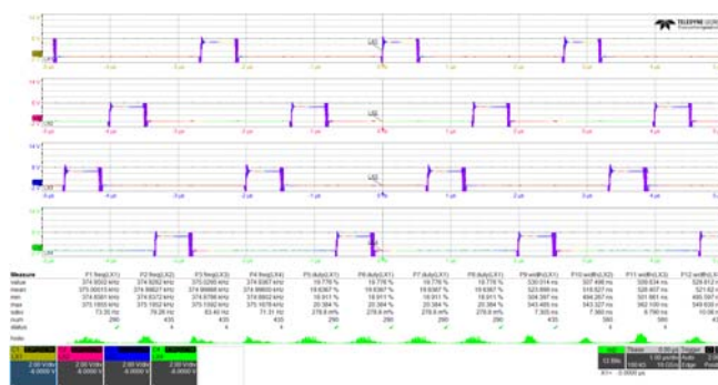
Figure 61. Phase Node Steady-State Jitter ( V_{DD} = 5V , P_{VIN} = 5V , I_{LOAD} = 150A )
