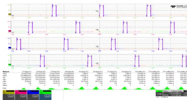
Figure 63. Phase Node Steady State Jitter (VDD = 12V, PVIN = 12V, I LOAD = 150A)
