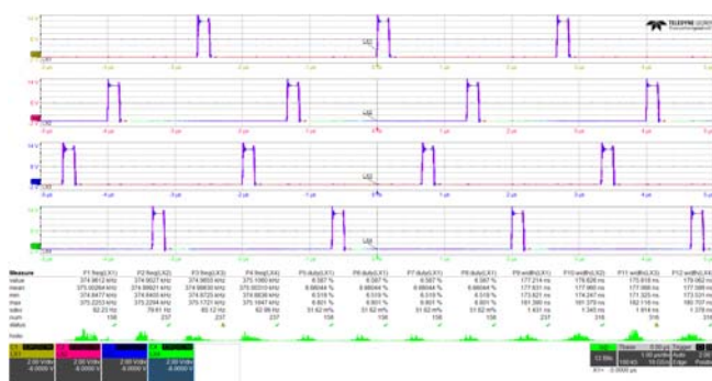
Figure 62. Phase Node Steady State Jitter (VDD = 12V, PVIN = 12V, I LOAD = 0A)
