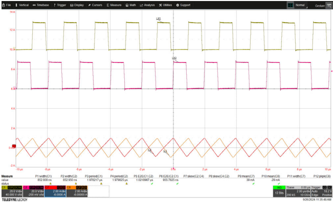
Figure 12. No Load LX Voltages and Inductor Currents
