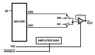
FIGURE 1. ISL59420, ISL59421 FUNCTIONAL BLOCK
