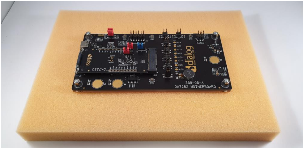
Figure 12. Placement of DA728x motherboard for optimal haptic feedback measurements
