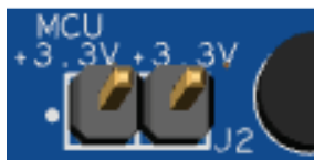
Figure 20. RX MCU Current Measurement
