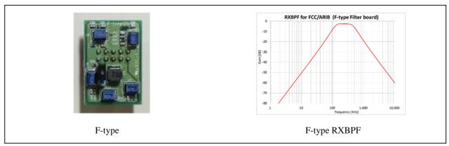
Figure 1-7: RX band pass filter (Filter board)
