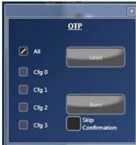
Figure 16. OTP Programming within Timing Commander GUI
