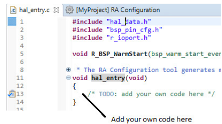
Figure 43: Adding user code to hal_entry.c
