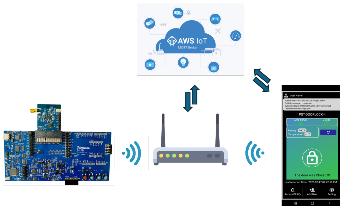
Figure 1. Architecture of AWS IoT reference application
