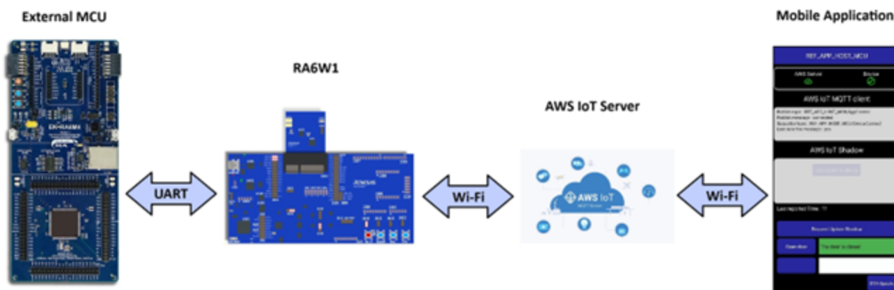
Figure 13. Architecture of AWS IoT reference application using AT commands
