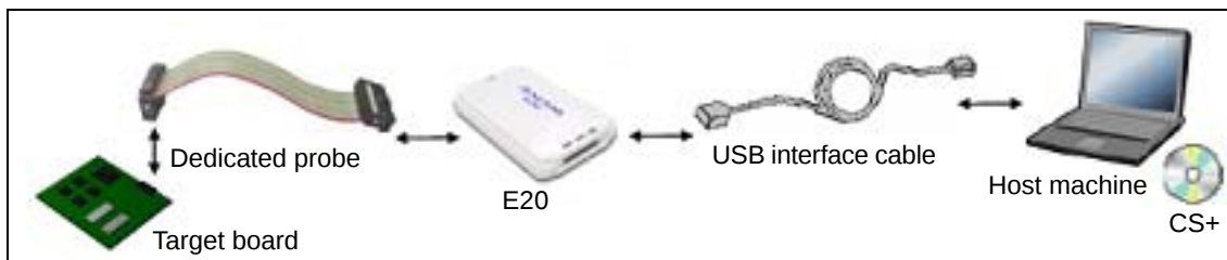
Figure 2.3 Connection Example [E20]
