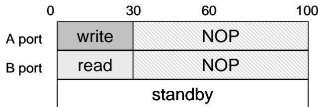
$$P_{DD} = P_{DDW} \times 0.3 + P_{DDR} \times 0.3 + P_{DDW} \times 0.7 + P_{DDR} \times 0.7 + \text{standby} \quad [\mu\text{W}]$$
