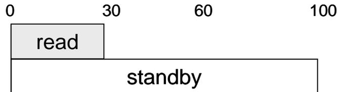
$$P_{DD} = P_{DDR} \times 0.3 + \text{standby} \quad [\mu\text{W}]$$
