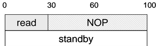
$$P_{DD} = P_{DDR} \times 0.3 + \text{NOP} \times 0.7 + \text{standby} \quad [\mu\text{W}]$$
