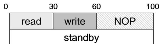
$$P_{DD} = P_{DDR} \times 0.3 + P_{DDW} \times 0.3 + \text{NOP} \times 0.4 + \text{standby} [\text{uW}]$$
