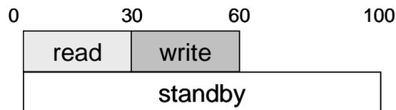
$$P_{DD} = P_{DDR} \times 0.3 + P_{DDW} \times 0.3 + \text{standby} [\text{uW}]$$
