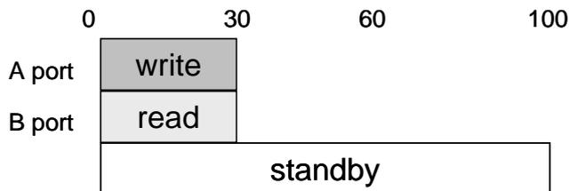
$$P_{DD} = P_{DDRA} \times 0.3 + P_{DDWA} \times 0.3 + \text{standby} \quad [\mu\text{W}]$$
