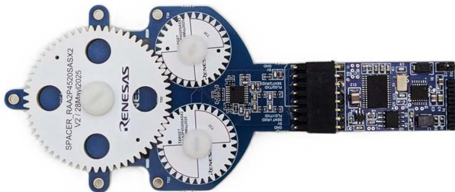
Figure 22: Assembled Board MCU and IPS Sensor
