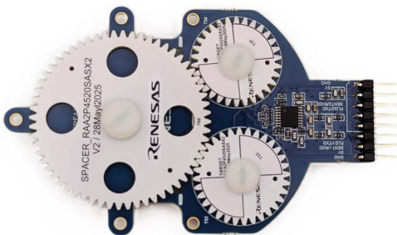
Figure 20: IPS Board Top View
