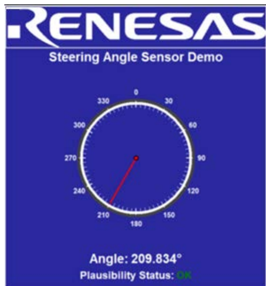
Figure 14: GUI Interface after Rotating the Gears on Sensor Board
