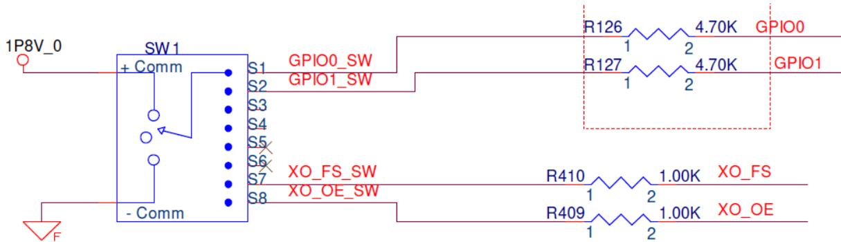
Figure 12. XO\_OE and XO\_FS Pins DIP Switch Schematic
