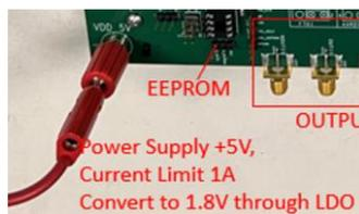
Figure 4. External 5V Board Input
