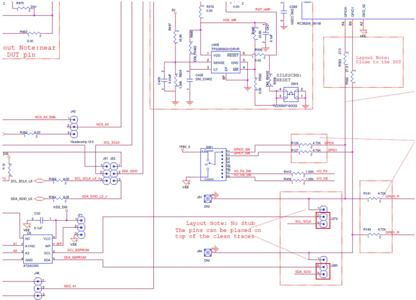
Figure 20. EEPROM Connection Jumpers for RC38208A SCL\_SCLK and SDA\_SDIO
