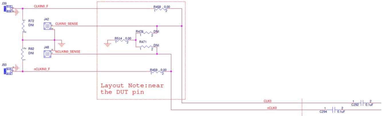
Figure 13. Input Clock with Sense Schematic
