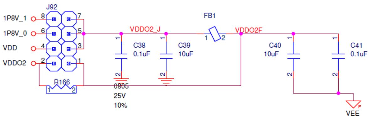
Figure 7. V<sub>DD</sub> Jumper Bypass Schematic
