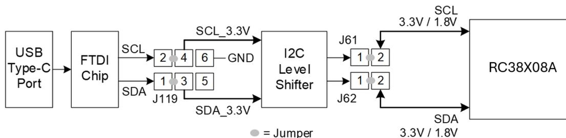
Figure 16. Communication Setup for I<sup>2</sup>C Mode
