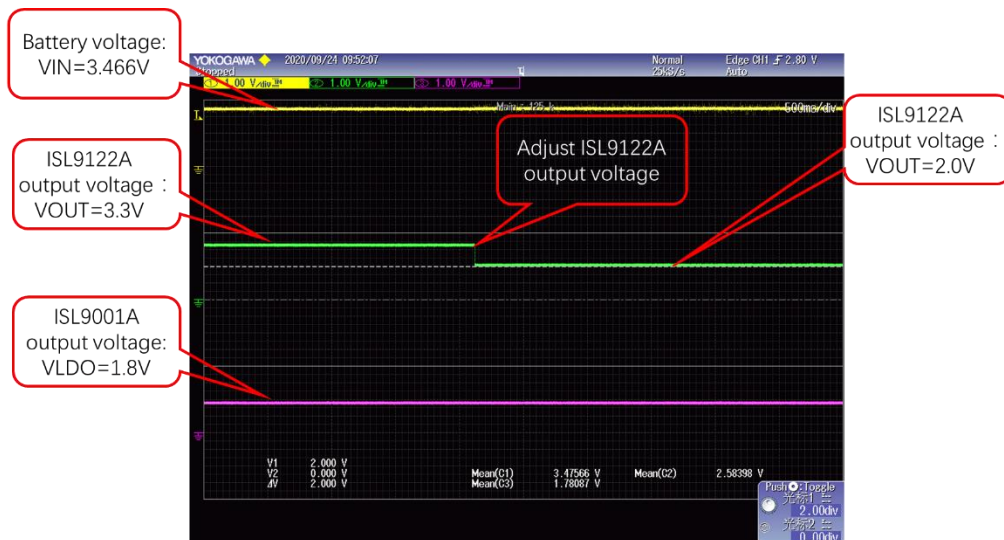
Figure 9 Test of Adjust the Output by PC
