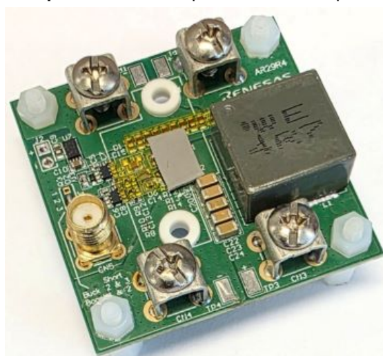
Step 2: Install SMD spacer, TIM and tapes
