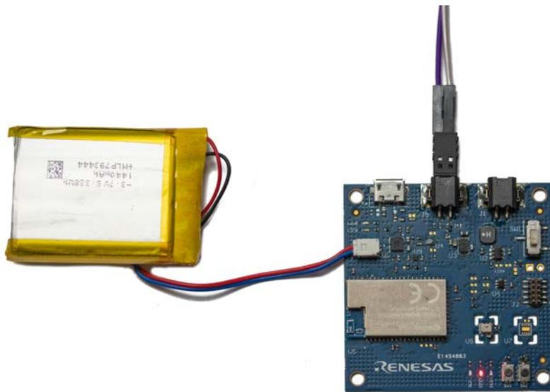
Figure 4: EU153-1 with battery and water leakage sensor
