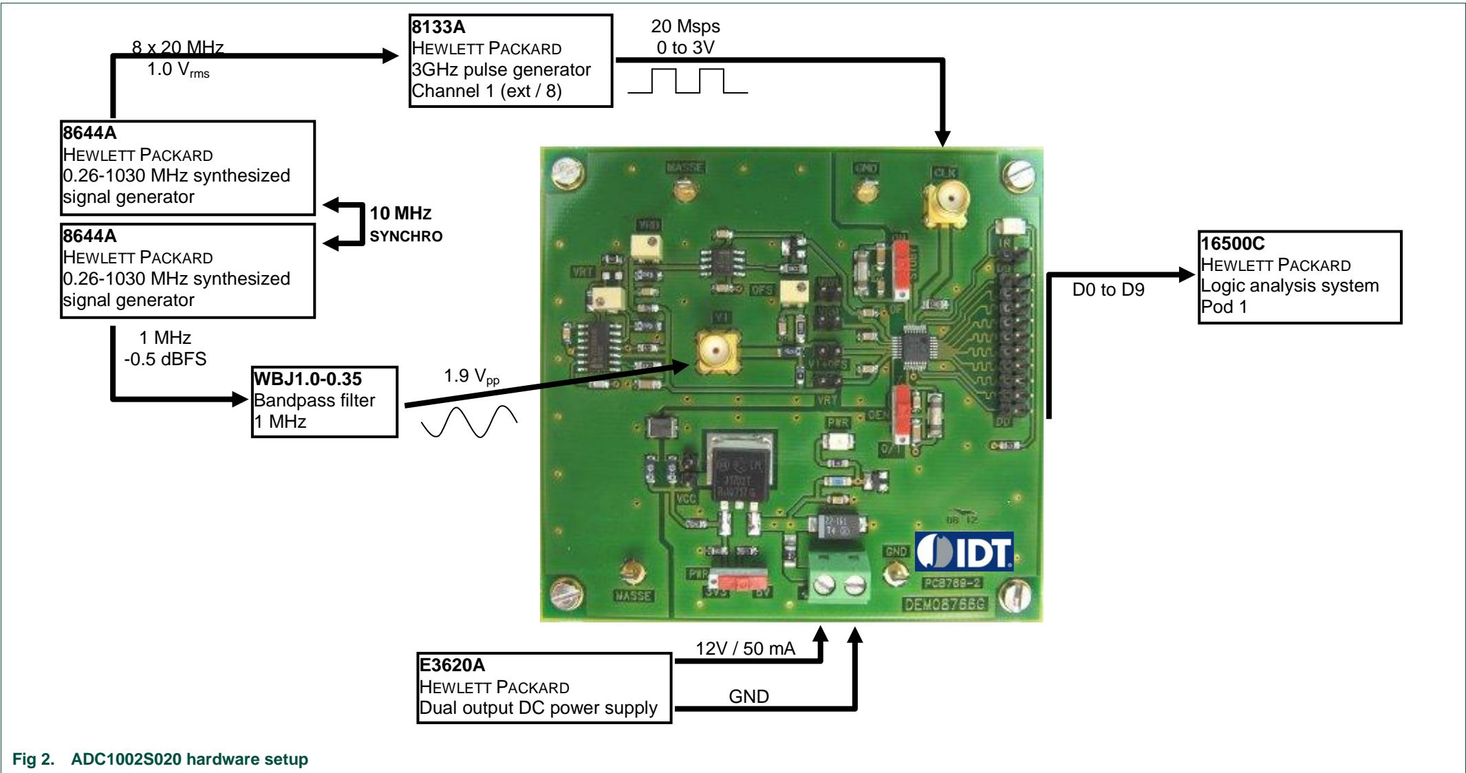
Fig 2. ADC1002S020 hardware setup
