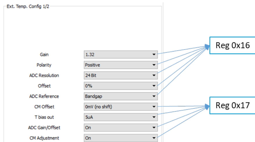
Figure 29. Ext Temp. 1/2 Sub-Tab
