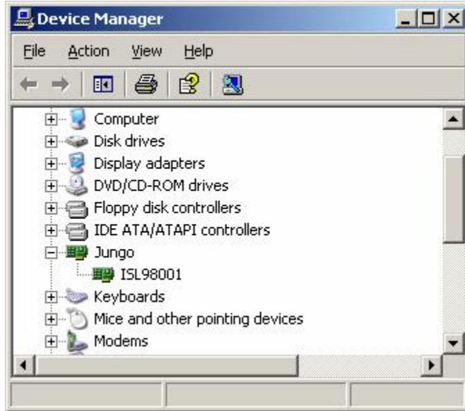
There should be a "Jungo" entry, with an ISL98001 sub category. This indicates the driver is properly installed and is communicating with the evaluation board. If this is not visible, or there are any error messages, take the following actions until the problem is resolved:
