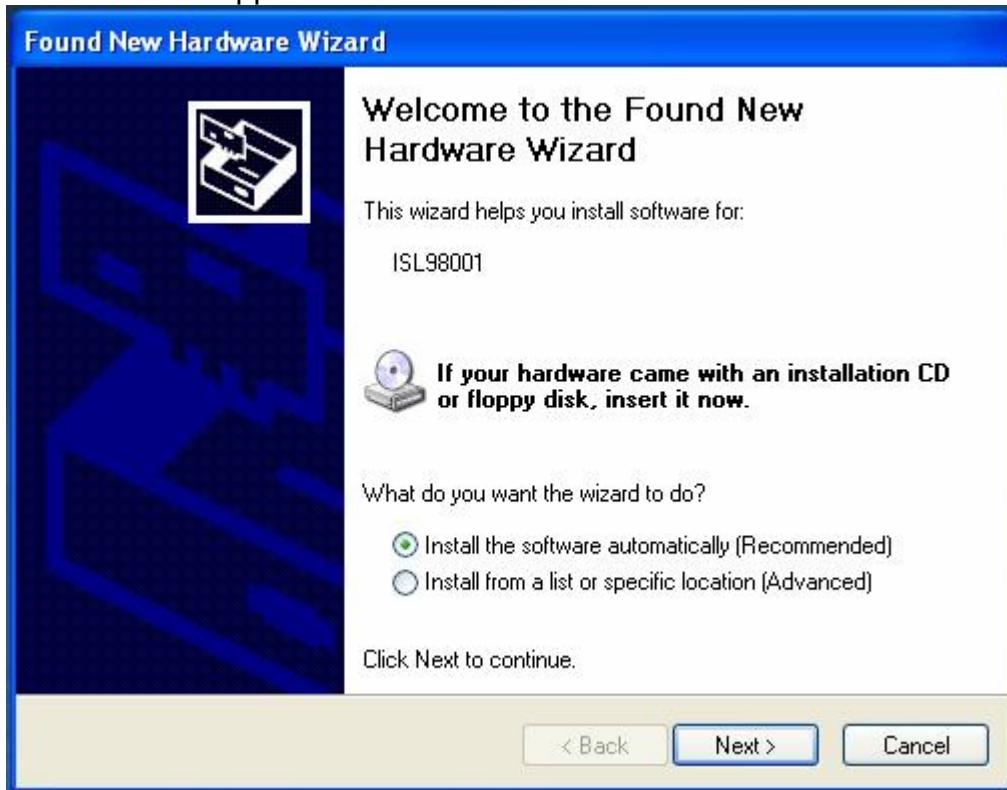
Press Next ("Install the software automatically").
