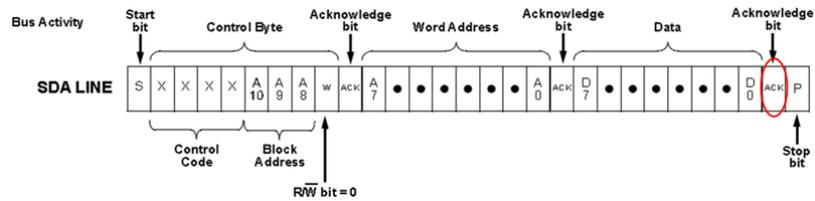
Figure 2: GreenPAK I<sup>2</sup>C Write Frame for Page Erase
