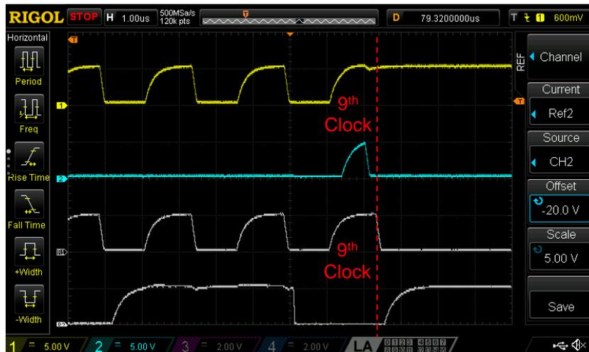
Figure 3: Non-I<sup>2</sup>C Compliant Behavior Oscilloscope
