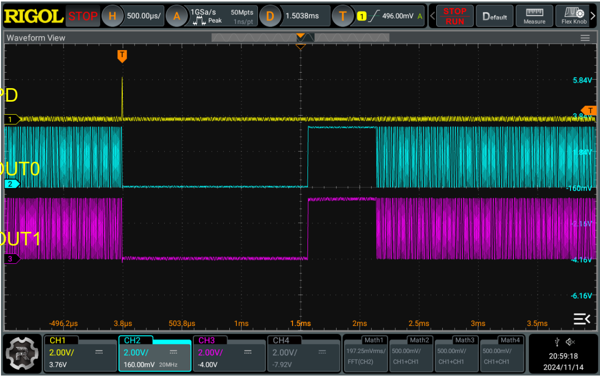
Figure 23. 2 MHz OSC Long Start-Up Timing Diagram
