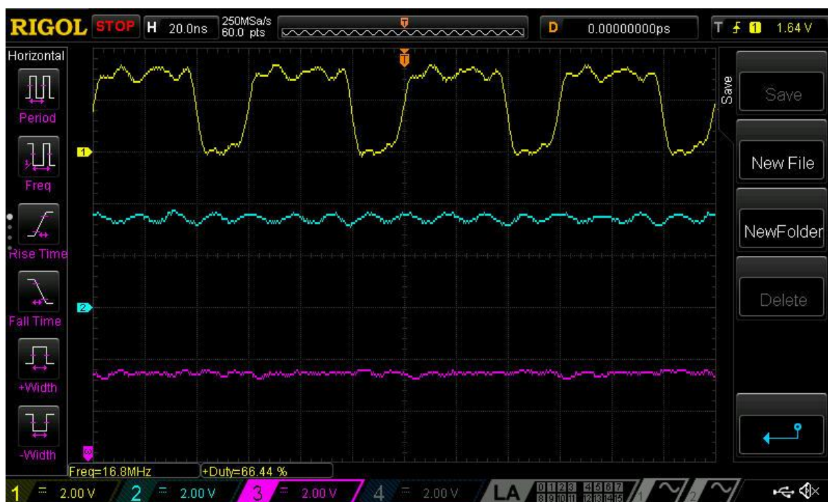
Figure 16. Waveforms at 60 ns Period and 40 ns Pulse Width (Correct Functionality)
