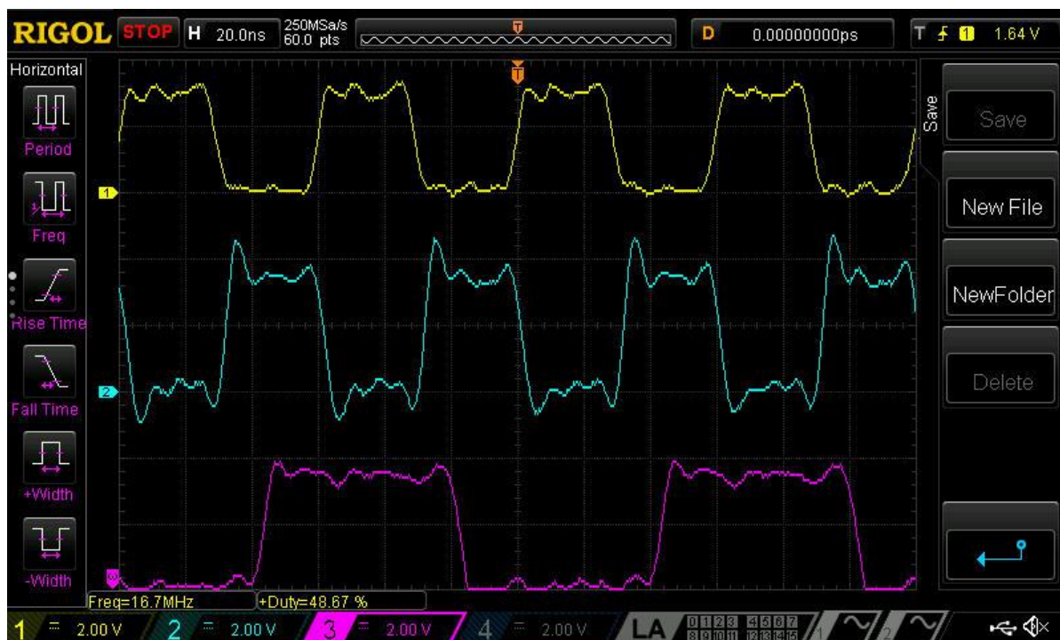
Figure 15. Waveforms at 60 ns Period and 30 ns Pulse Width (Incorrect Functionality)
