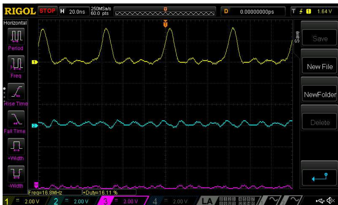
Figure 13. Waveforms at 60 ns Period and 10 ns Pulse Width (Correct Functionality)
