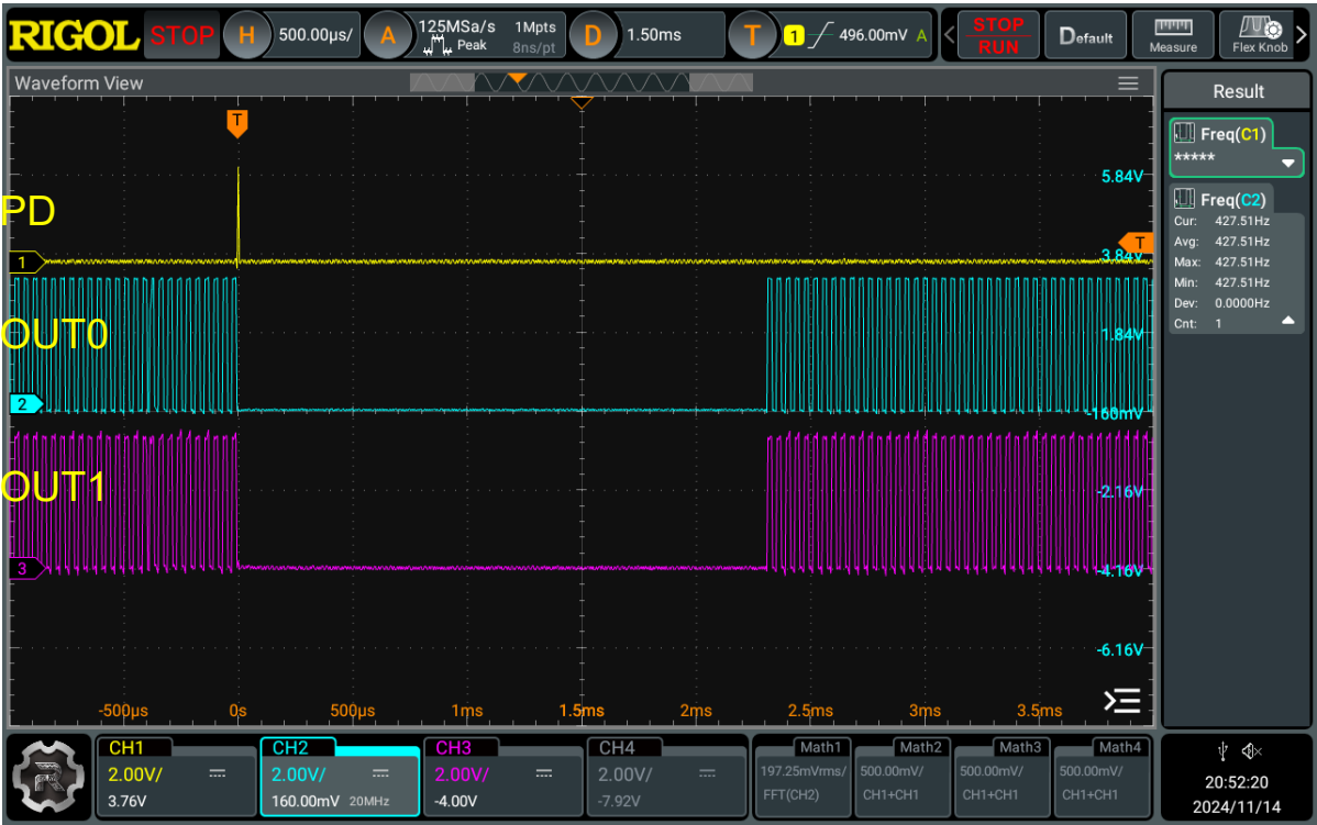
Figure 22. 25 kHz OSC Long Start-Up Timing Diagram
