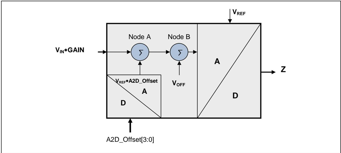
Digital representation of the input voltage as a signed number requires calculating the difference  $Z_{SENSOR} - Z_{AUTOZERO}$ .
