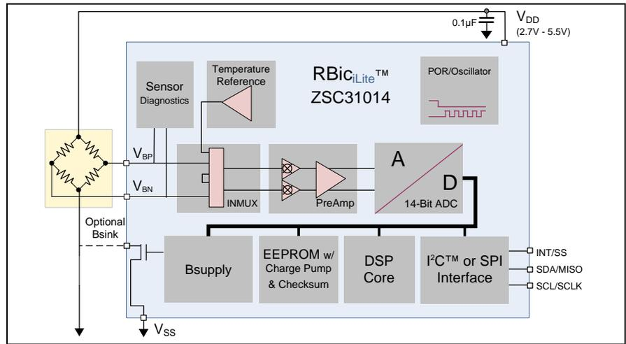
**Application: Half-Bridge Voltage Measurement**
