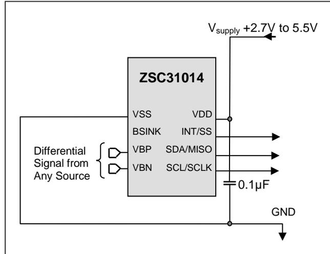
Figure 4.2 Example 2 Circuit Diagram: Generic Differential A2D Converter
