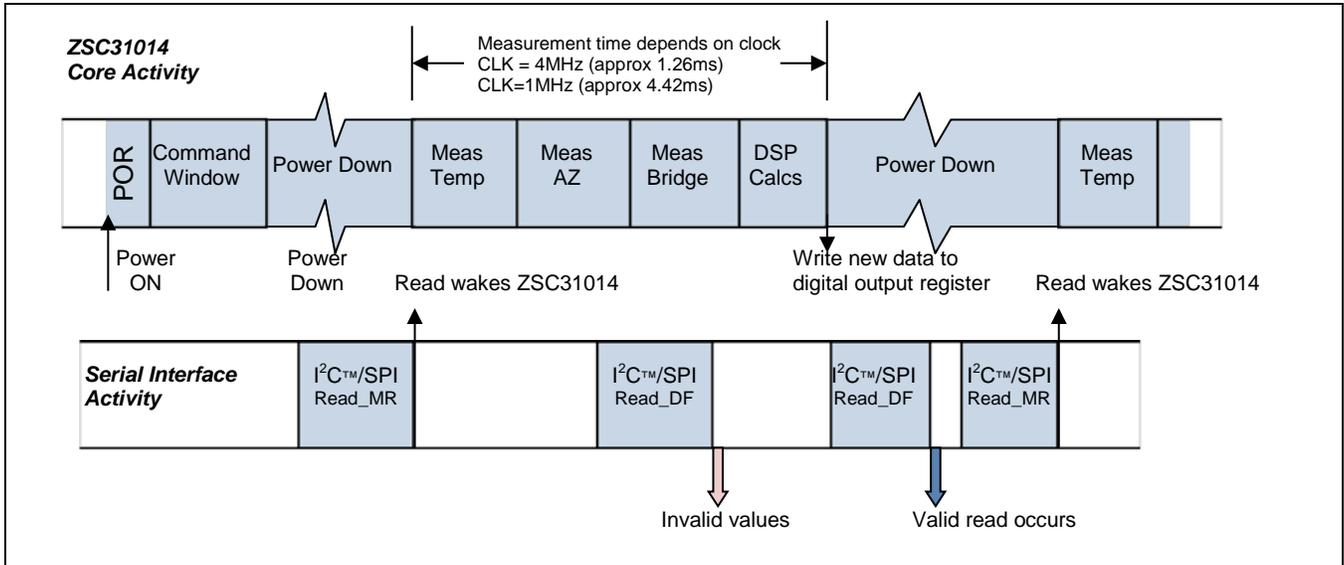
**Figure 3.5 Sequence during Sleep Mode Using an I<sup>2</sup>C™ Write\_MR to Wake Up (Typical Timing Values\*\*)**
