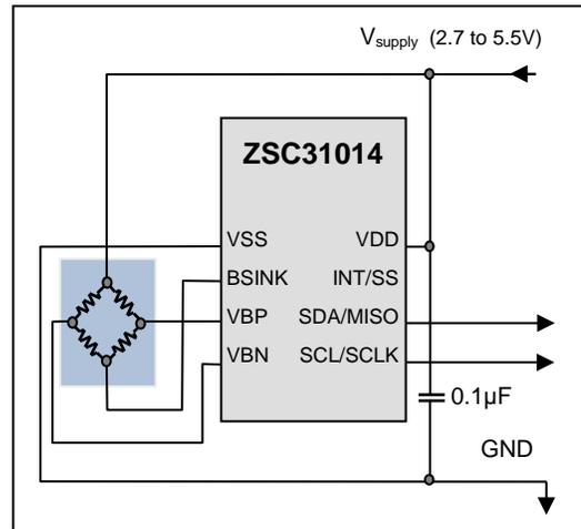
**Figure 4.1** Example 1 Circuit Diagram: Bsink Option and Internal Temperature Correction and I<sup>2</sup>C™ Output
