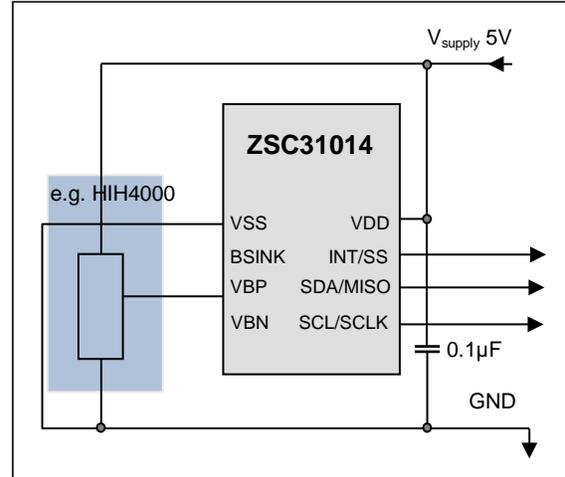
**Figure 4.3** Half-Bridge Voltage Measurement with Internal Temperature Correction
