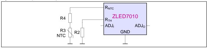
As shown in Figure 4.1, the temperature compensation curve is determined by R2, R3 (NTC) and R4. When the LED temperature increases, the resistance of R3 decreases. As R3 reaches the point that R3 plus R4 equal R2, the temperature compensation function starts to work by reducing I<sub>OUT</sub>.
