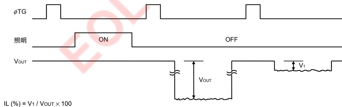
$$\text{IL (\%)} = V_1 / V_{\text{out}} \times 100$$
