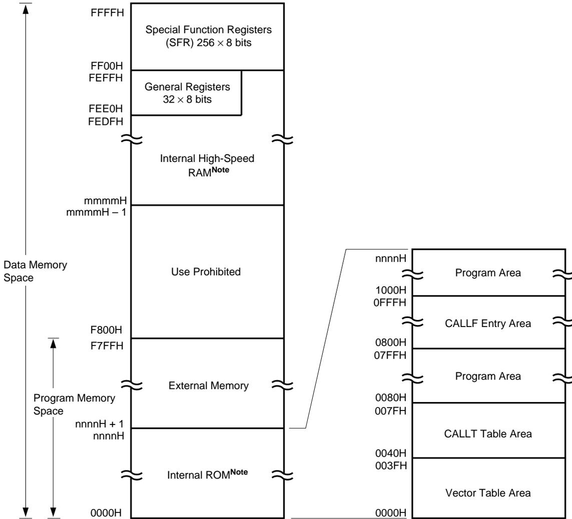
**Note** The internal ROM capacity and internal high-speed RAM capacity depend on the products (see the following table).
