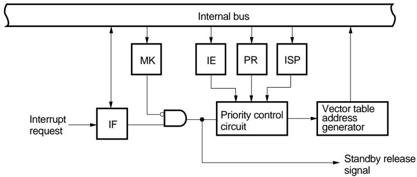
(C) External maskable interrupt (INTP0 to INTP3)
