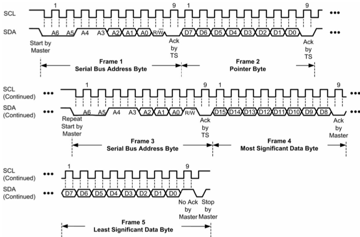
SMBus/I<sup>2</sup>C write to the Configuration Register to Enable Shutdown ((SHDN) <0000 0001 0000 0000>b)
