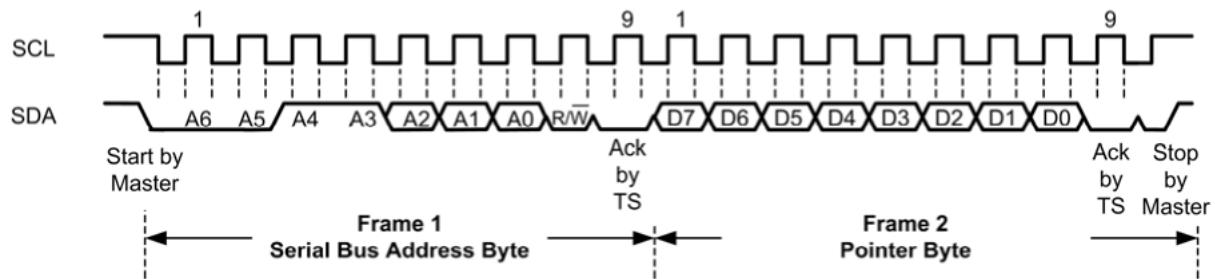
SMBus/I<sup>2</sup>C write to the pointer register followed by a write data word
