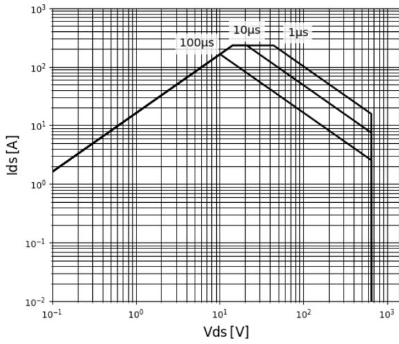
Figure 15. Safe Operating Area T<sub>c</sub> = 25°C
