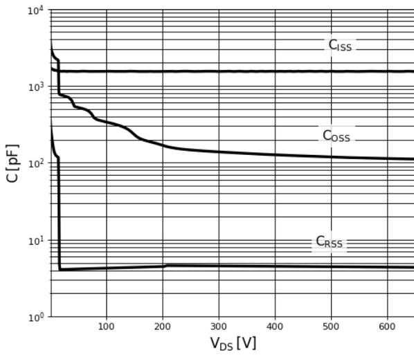
**Figure 7. Typical Capacitance**
