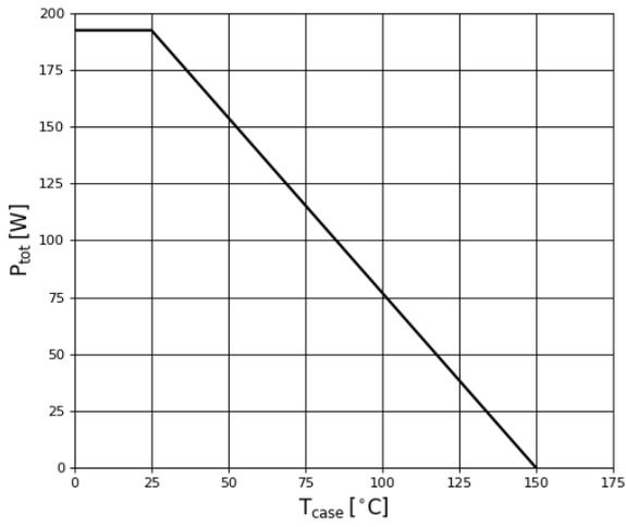
Figure 11. Power Dissipation
