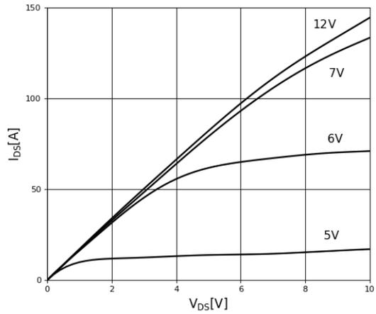
**Figure 4. Typical Output Characteristics,  $T_J = 150^\circ\text{C}$**
