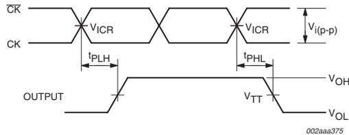
$V_{TT} = V_{DD}/2$
