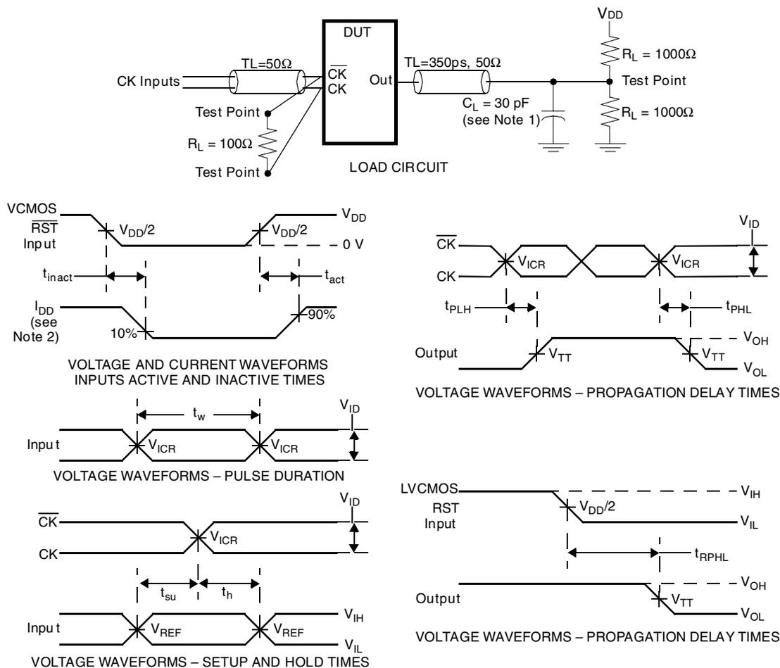
Figure 6 — Parameter Measurement Information ( $V_{DD} = 1.8V \pm 0.1V$ )
