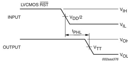
$V_{TT} = V_{DD}/2$
