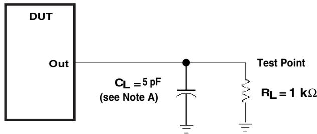
(1)  $C_L$  includes probe and jig capacitance.
