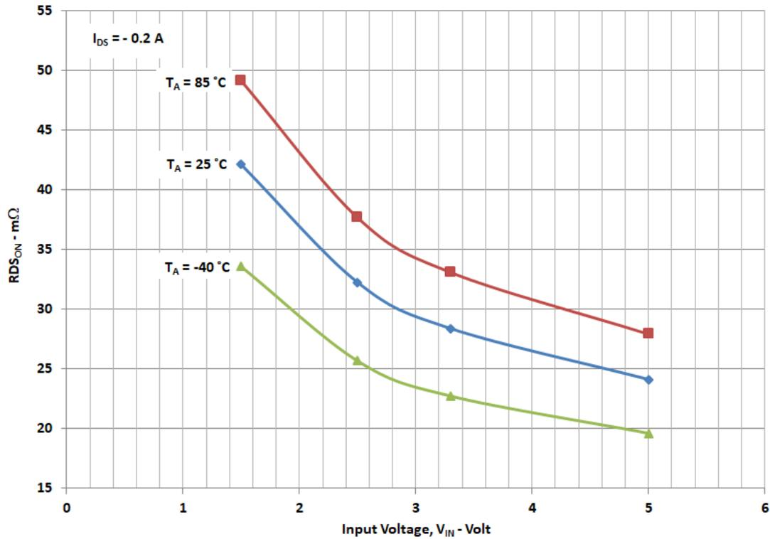
RDS<sub>ON</sub> vs. Temperature and V<sub>IN</sub>
