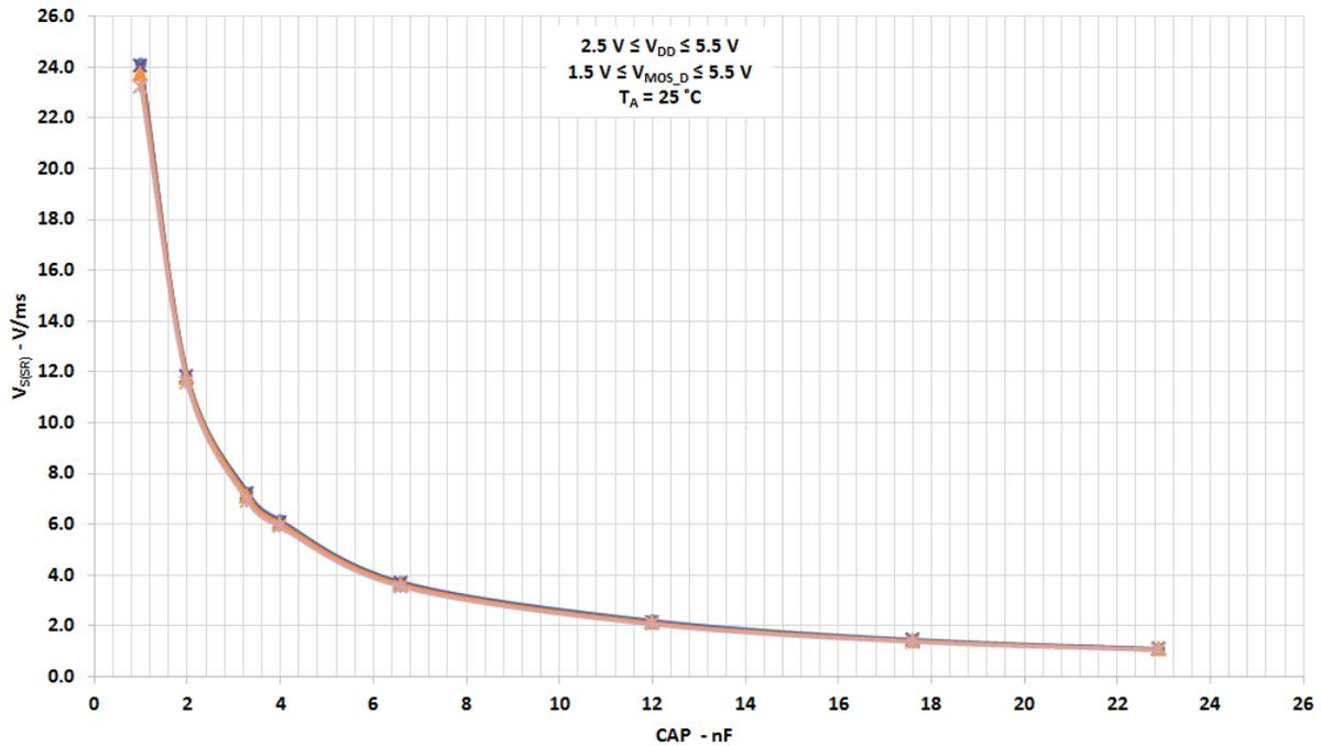
$T_{Total\_ON}$  vs. CAP,  $V_{MOS\_D}$ , and  $V_{DD}$
