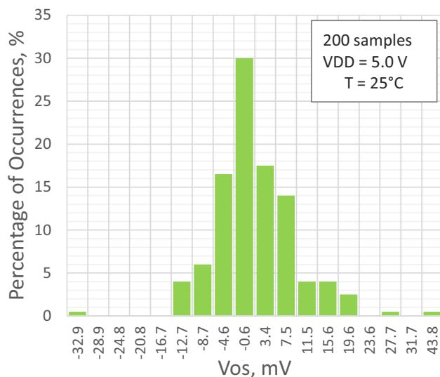
Figure 17: PGA Input Offset Distribution, Single-Ended Mode, G = 0.25
