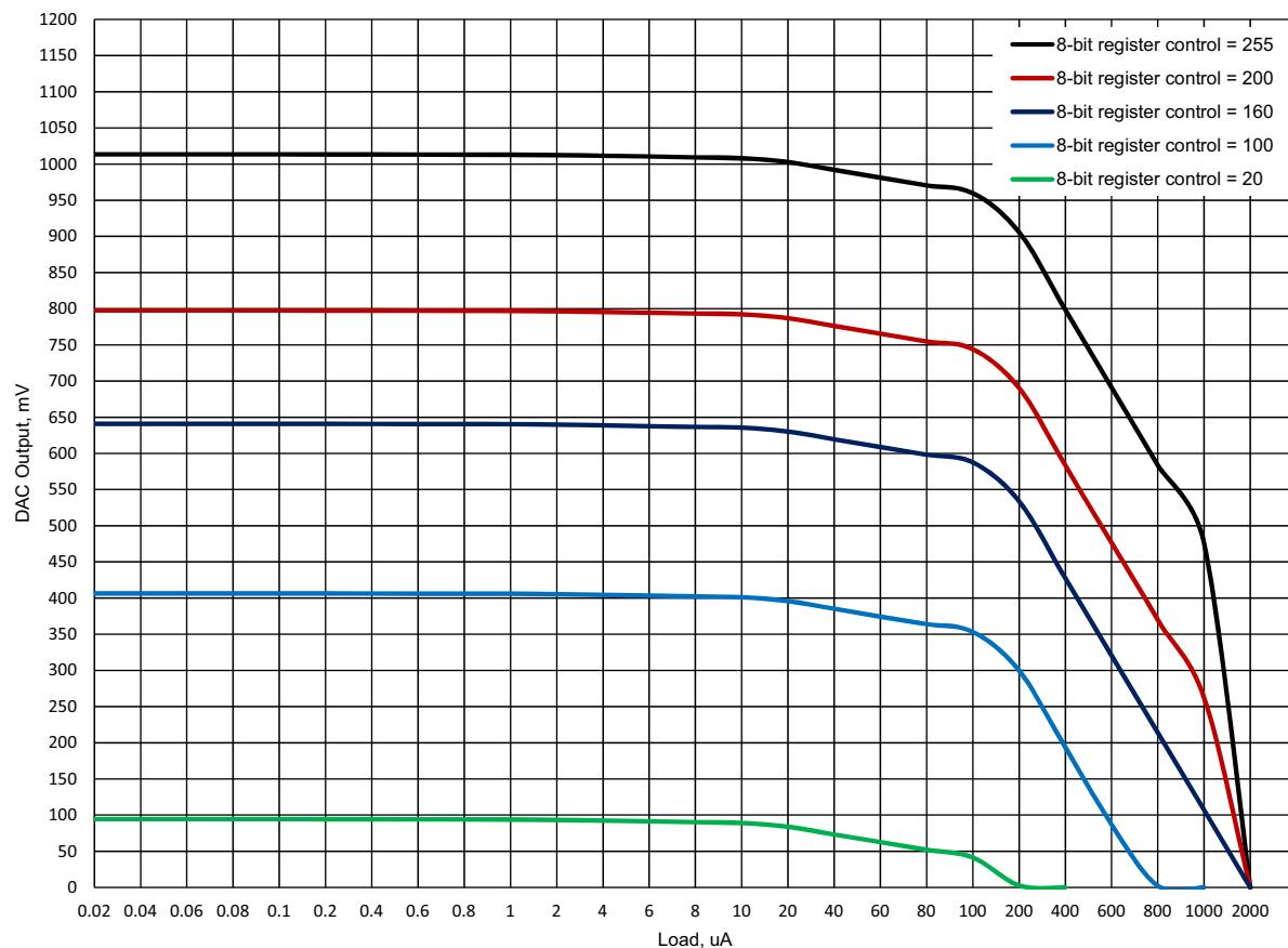
Figure 31: DAC Typical Load Regulation,  $T_A = 25^\circ\text{C}$ ,  $V_{DD} = 3.3\text{ V}$
