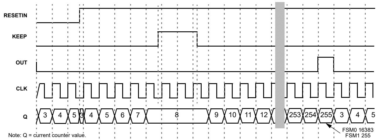
Figure 82: CNT/FSM Timing Diagram (Set Rising Edge Mode, Oscillator is Forced on, UP = 1) for Counter Data = 3
