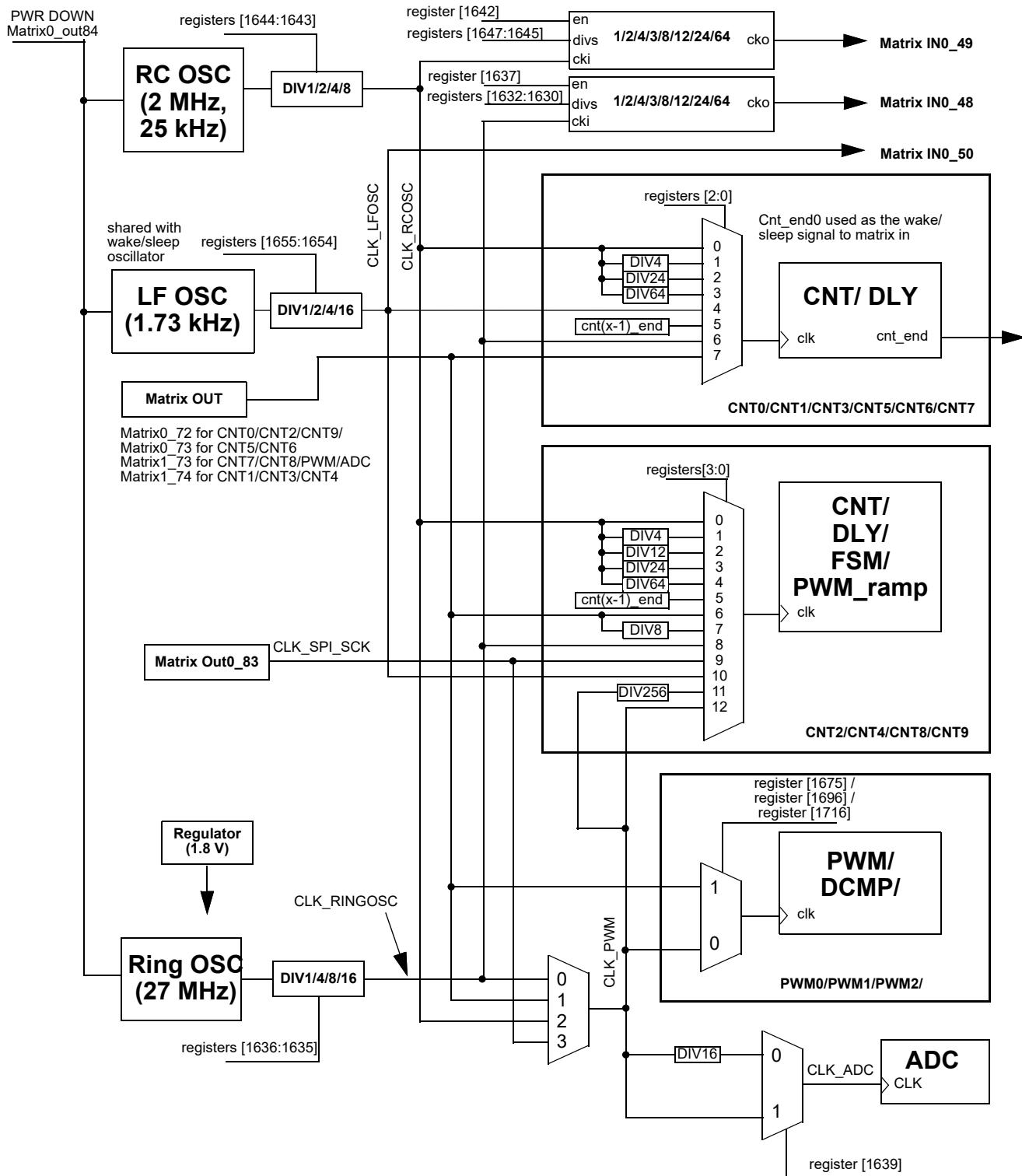
Figure 102: Oscillator Block Diagram
