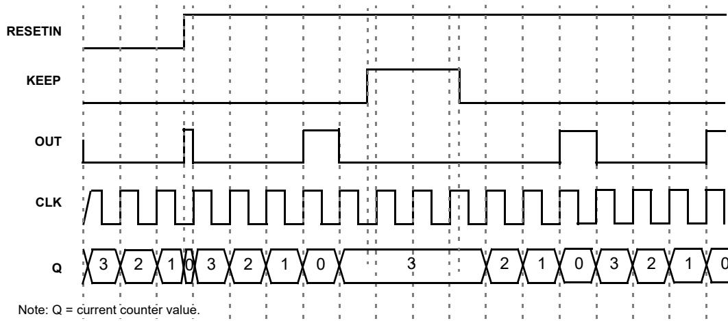
Figure 79: CNT/FSM Timing Diagram (Reset Rising Edge Mode, Oscillator is Forced On, UP = 0) for Counter Data = 3
