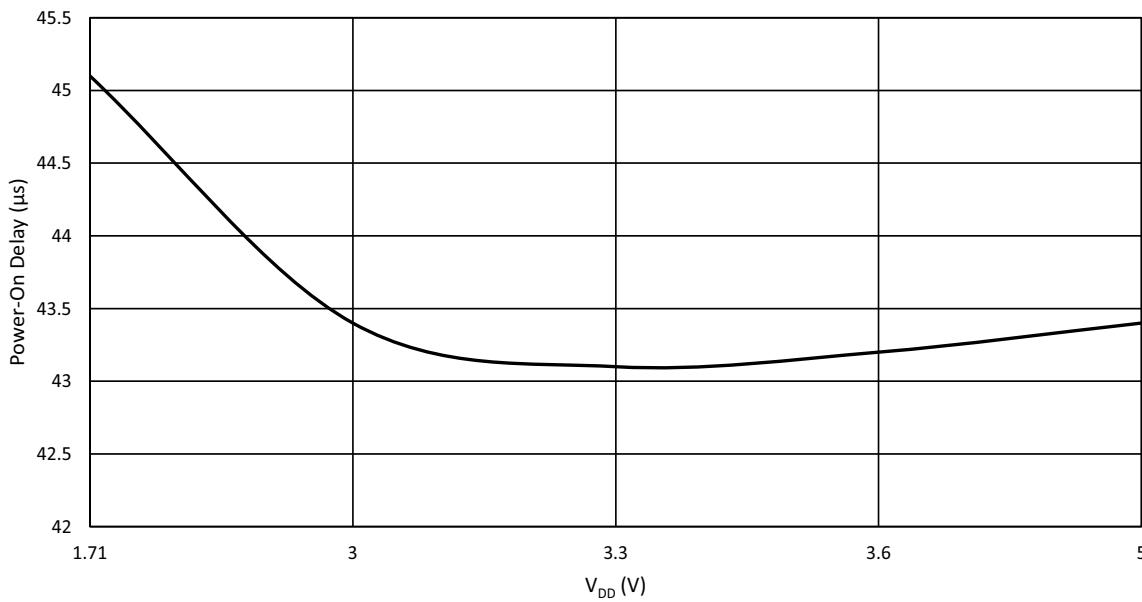
Figure 106: RC Oscillator Maximum Power-On Delay vs.  $V_{DD}$  at  $T_A = 25^\circ\text{C}$ , RC OSC = 25 kHz
