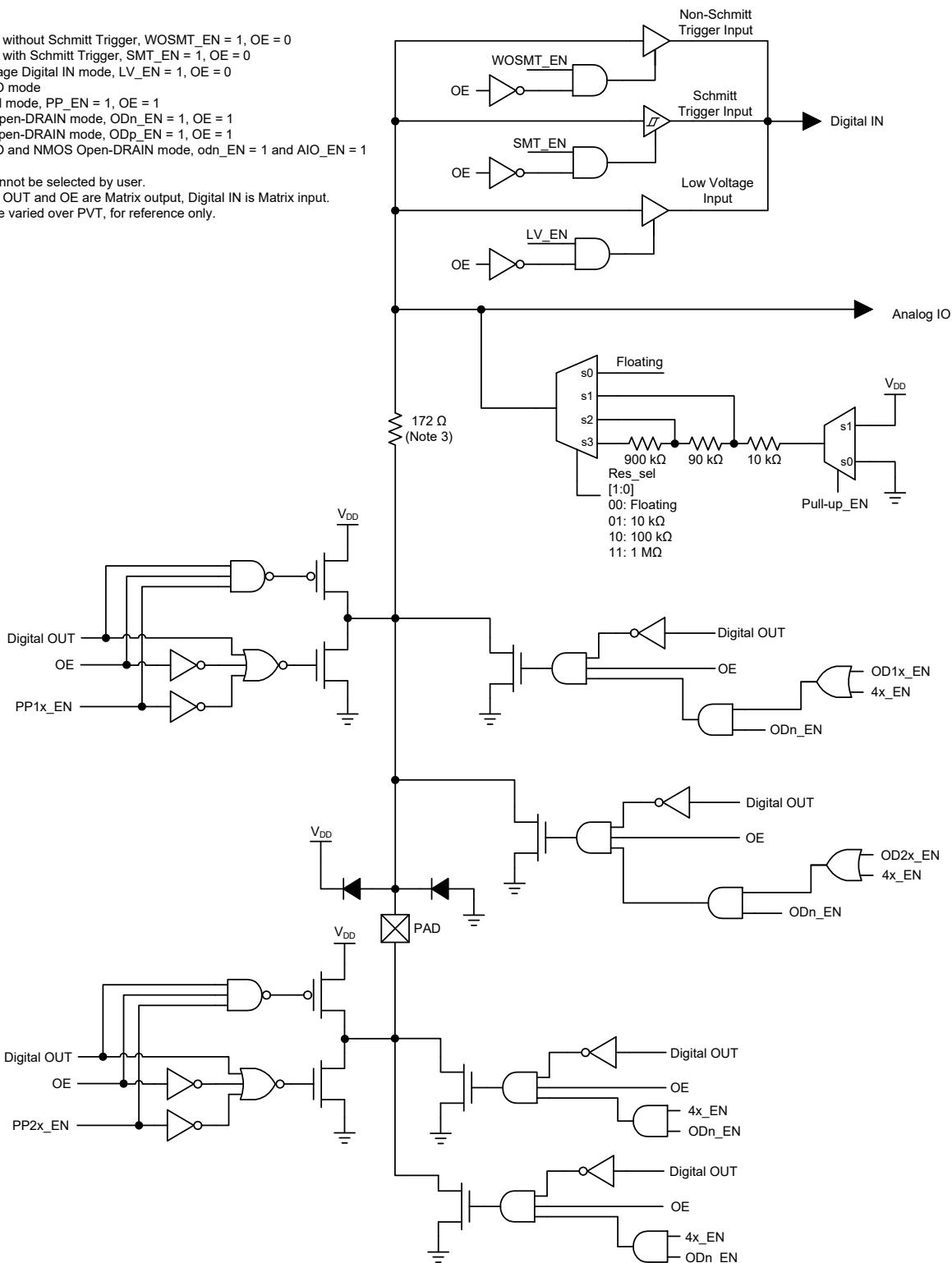
Figure 6: Register OE 4x Drive Structure Diagram
