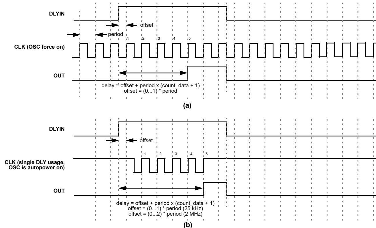
Figure 74: Timing (Rising Edge) for Count Data = 3: (a) Oscillator is in Force Power On Mode or an External Oscillator is Used, (b) Oscillator is in Auto Power On Mode
