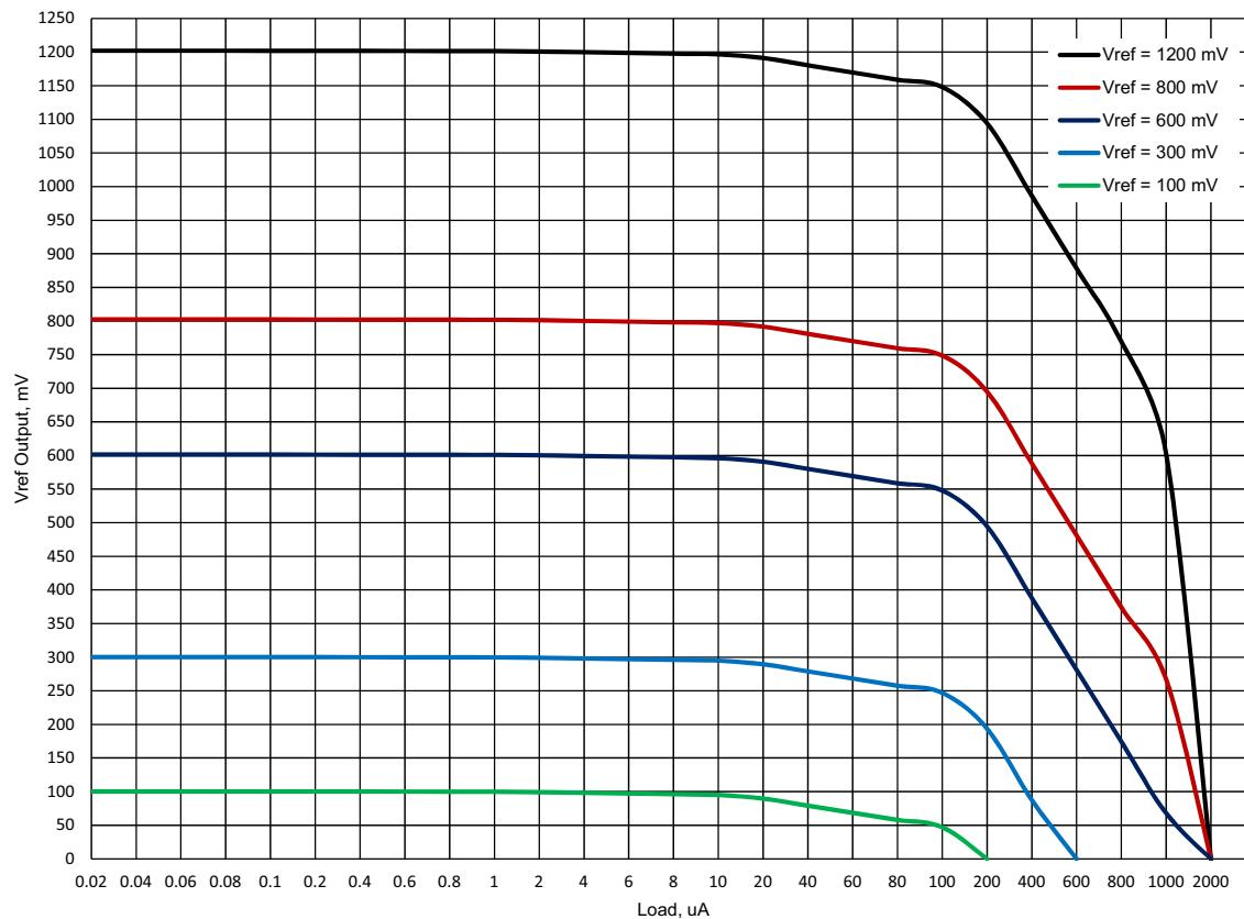
Figure 101: Typical Load Regulation,  $T_A = 25^\circ\text{C}$ ,  $V_{DD} = 3.3\text{ V}$
