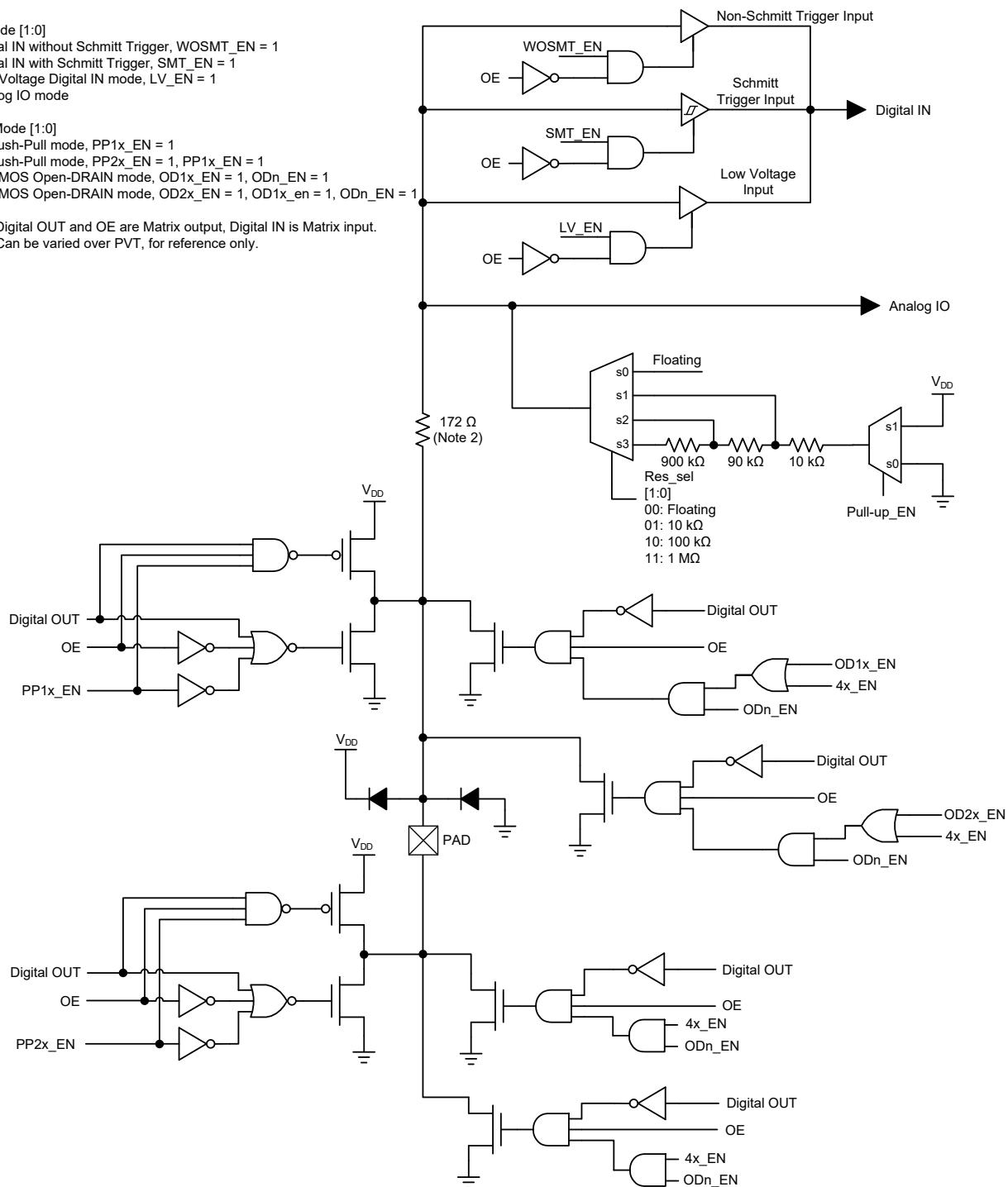
Figure 4: Matrix OE IO 4x Drive Structure Diagram
