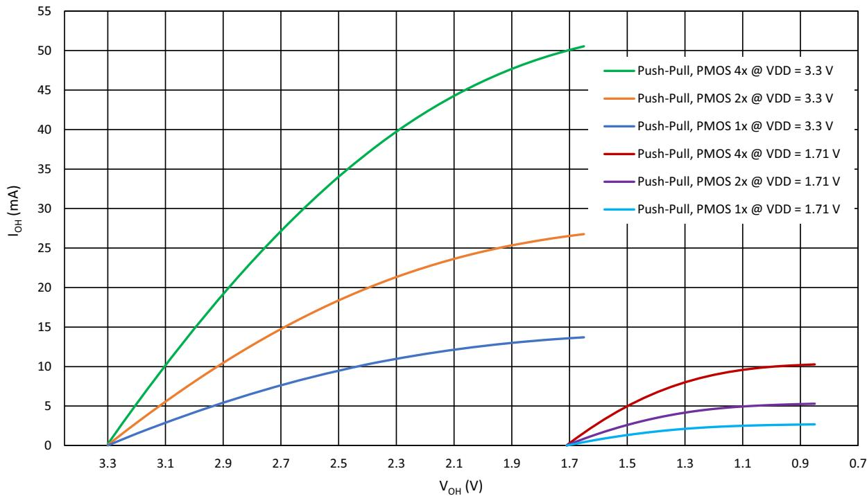
Figure 7: Typical High Level Output Current vs. High Level Output Voltage at  $T_A = 25^\circ\text{C}$
