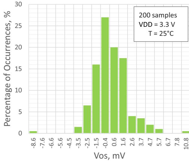
Figure 19: PGA Input Offset Distribution, Single-Ended Mode, G = 1
