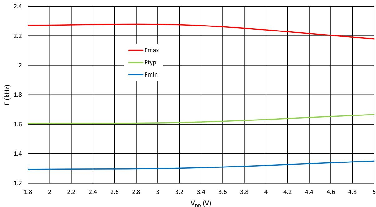
Figure 109: LF Oscillator Frequency vs. V<sub>DD</sub>, OSC = 1.73 kHz, T<sub>A</sub> = -40 °C to 125 °C
