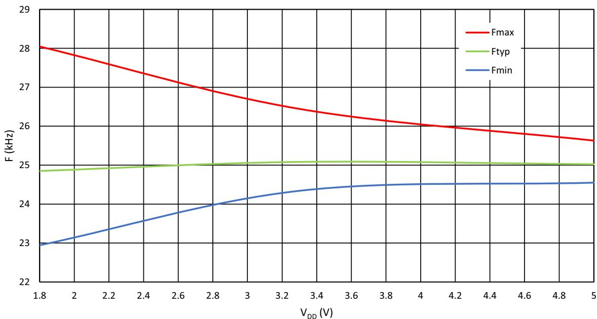
Figure 112: RC Oscillator Frequency vs. V<sub>DD</sub>, RC OSC = 25 kHz, T<sub>A</sub> = 25 °C
