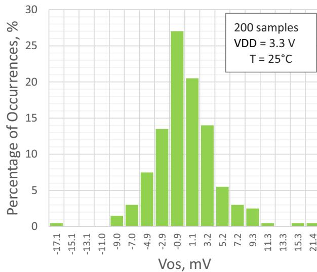
Figure 18: PGA Input Offset Distribution, Single-Ended Mode, G = 0.5
