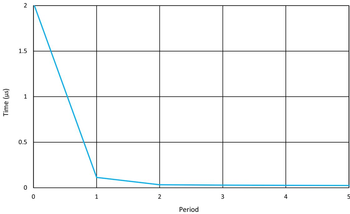
Figure 119: Ring Oscillator Settling Time,  $V_{DD} = 3.3$  V,  $T_A = 25$  °C, OSC = 27 MHz
