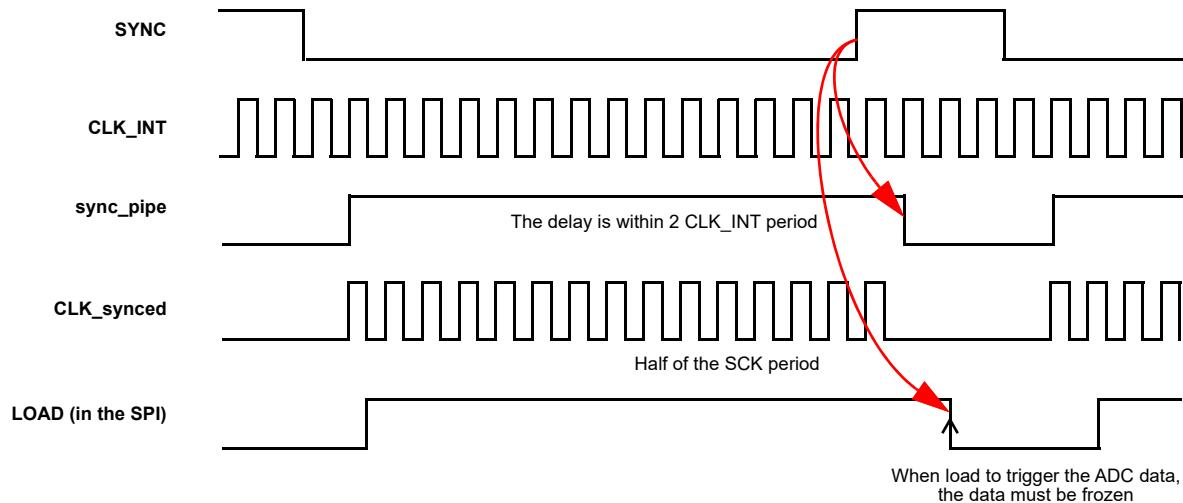
Figure 91: Timing Diagram Showing SPI Clock Synchronization
