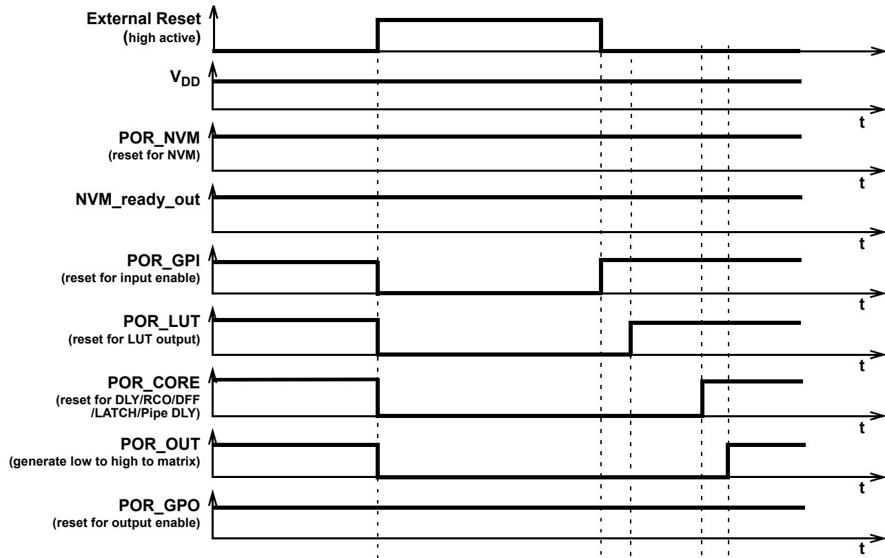
Figure 123: External Reset Sequence (High Active)
