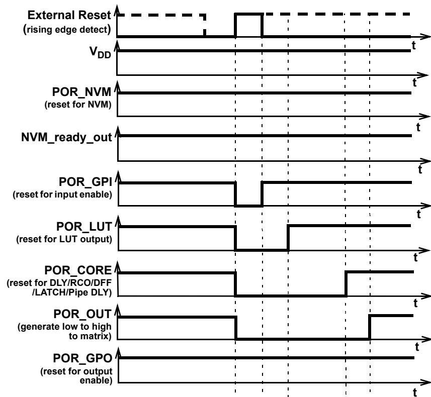
Figure 124: External Reset Sequence (Rising Edge Detect)
