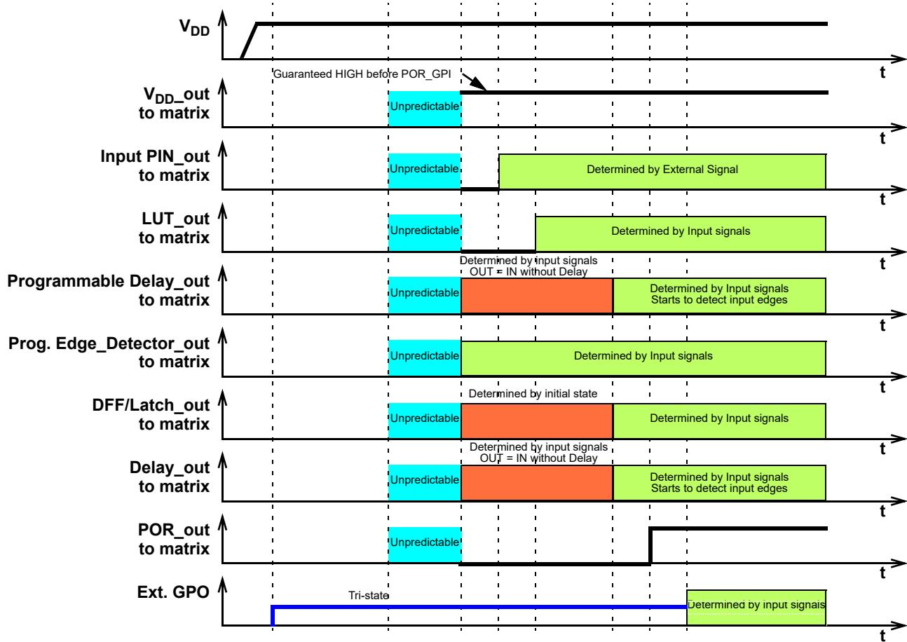
Figure 121: Internal Macrocell States during POR Sequence
