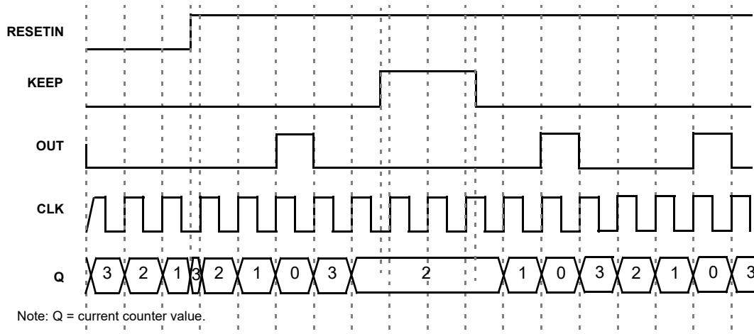
Figure 80: CNT/FSM Timing Diagram (Set Rising Edge Mode, Oscillator is Forced on, UP = 0) for Counter Data = 3
