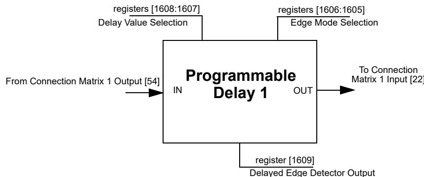
Figure 96: Programmable Delay
