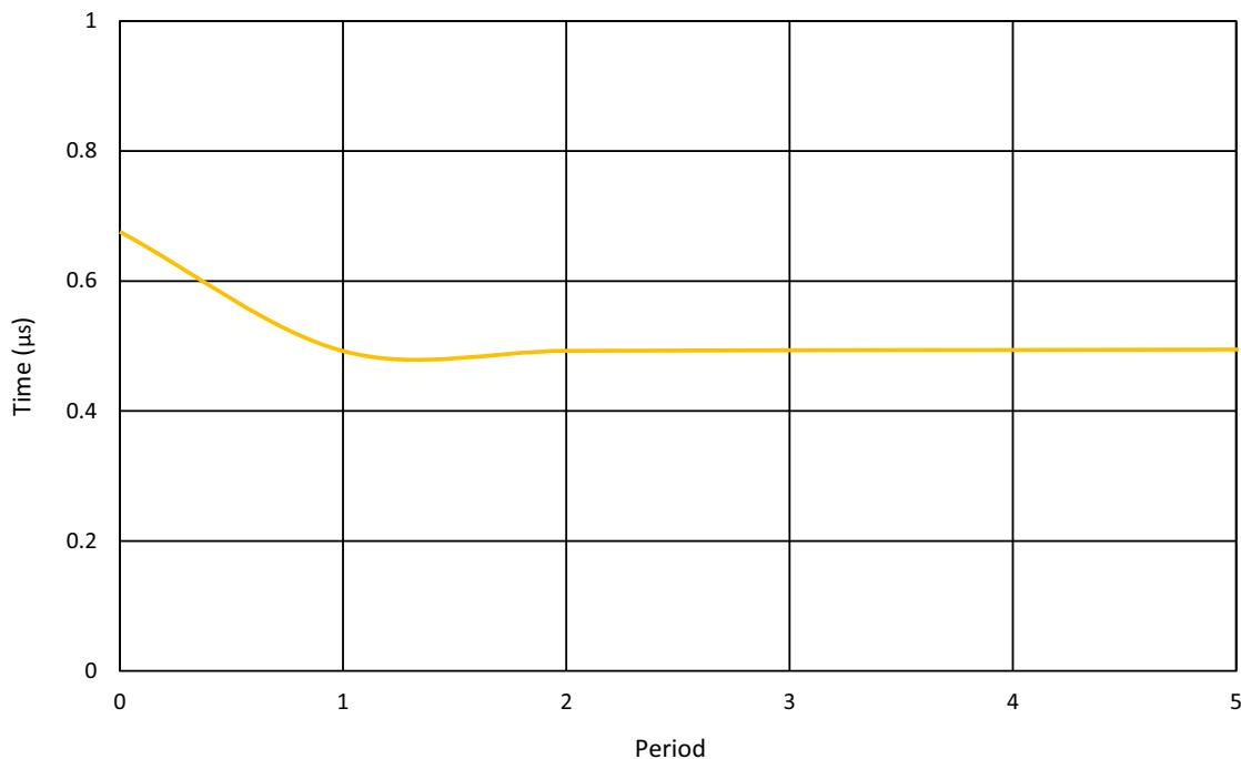
Figure 117: RC Oscillator Settling Time,  $V_{DD} = 3.3$  V,  $T_A = 25$  °C, OSC = 2 MHz
