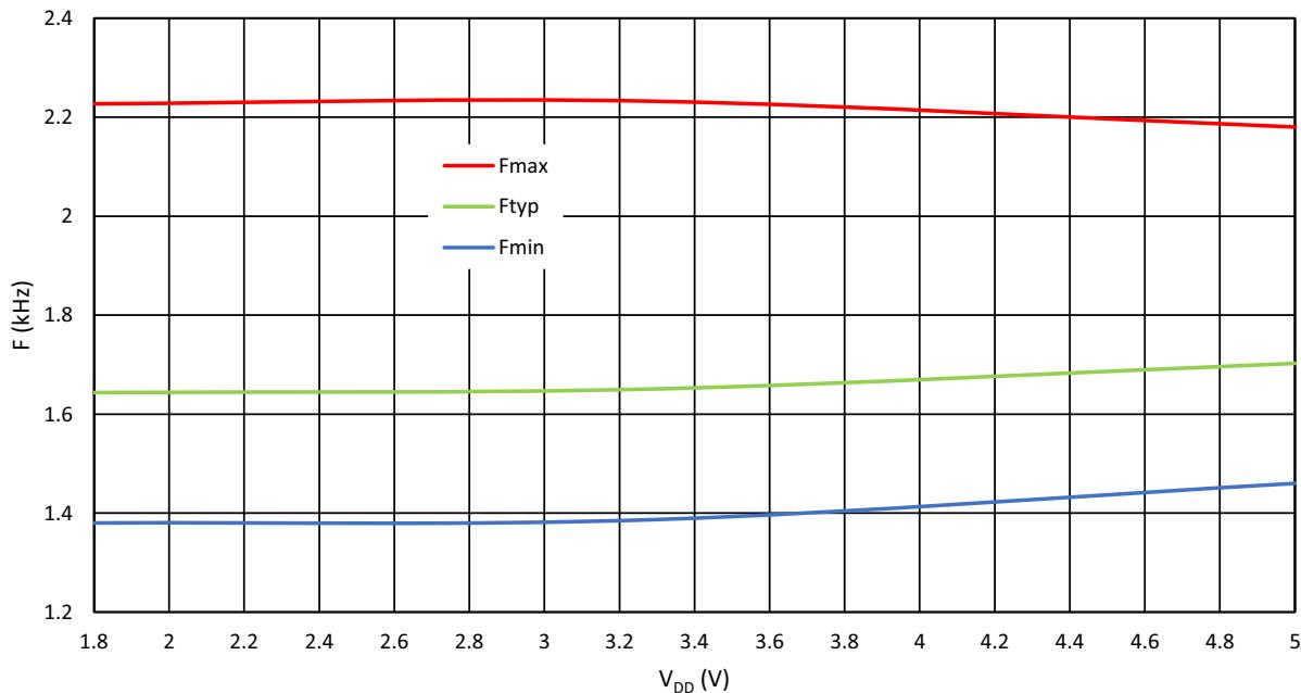
Figure 108: LF Oscillator Frequency vs.  $V_{DD}$ , OSC = 1.73 kHz,  $T_A = 25^\circ\text{C}$
