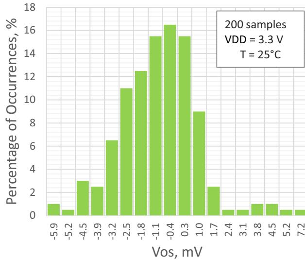
Figure 20: PGA Input Offset Distribution, Single-Ended Mode, G = 2
