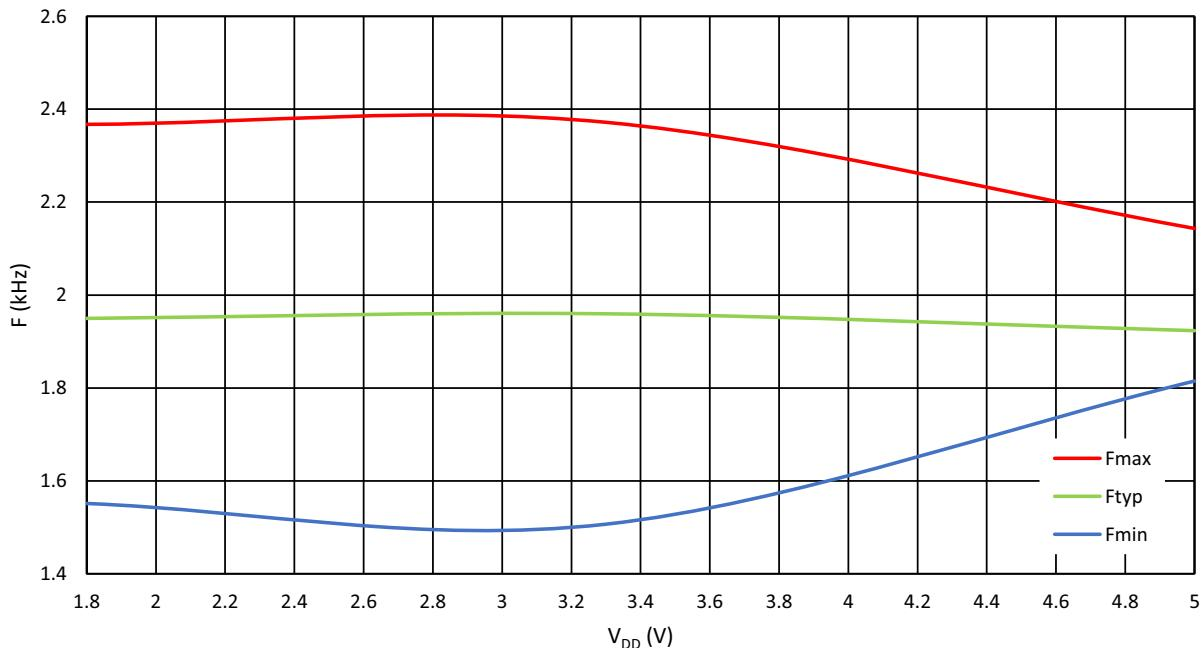
Figure 111: RC Oscillator Frequency vs. V<sub>DD</sub>, OSC = 2 MHz, T<sub>A</sub> = -40 °C to 125 °C
