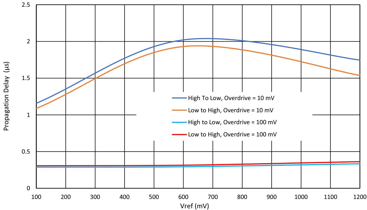
Figure 47: Propagation Delay vs. Vref for ACMPx at  $T_A = 25^\circ\text{C}$ , at  $V_{DD} = 1.71\text{ V to }5\text{ V}$ , Gain = 1, Hysteresis = 0
