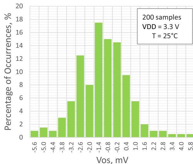
Figure 21: PGA Input Offset Distribution, Single-Ended Mode, G = 4
