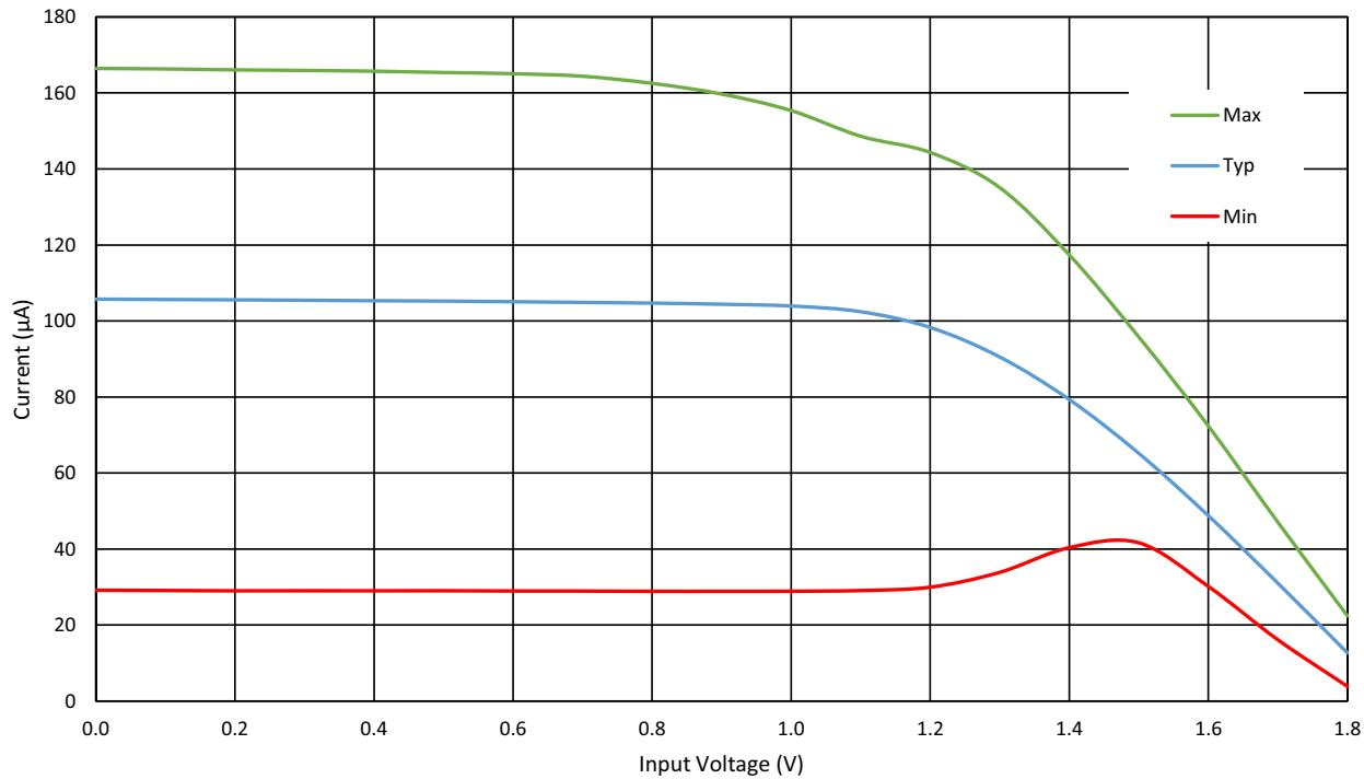
Figure 48: ACMP Input Current Source vs. Input Voltage at  $T_A = -40^\circ\text{C to }125^\circ\text{C}$ ,  $V_{DD} = 3.3\text{ V}$
