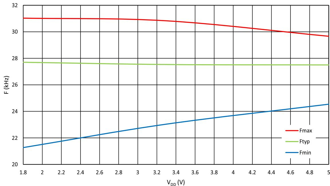
Figure 114: Ring Oscillator Frequency vs. V<sub>DD</sub>, OSC = 27 MHz, T<sub>A</sub> = 25 °C
