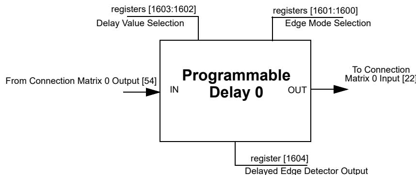
Figure 95: Programmable Delay
