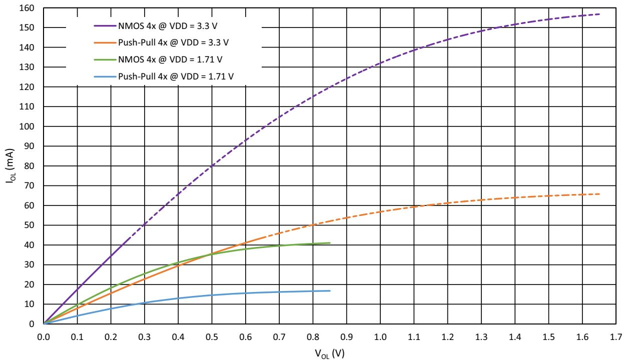
Figure 10: Typical Low Level Output Current vs. Low Level Output Voltage, 4x Drive at  $T_A = 25^\circ\text{C}$
