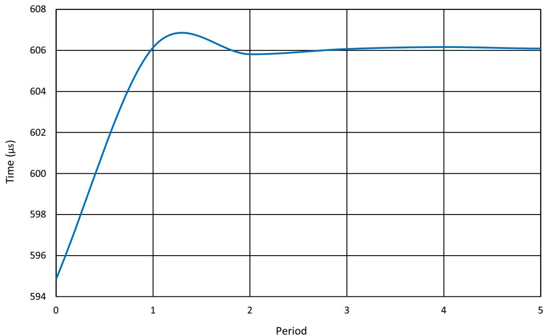
Figure 116: LF Oscillator Settling Time,  $V_{DD} = 3.3$  V,  $T_A = 25$  °C, OSC = 1.73 kHz
