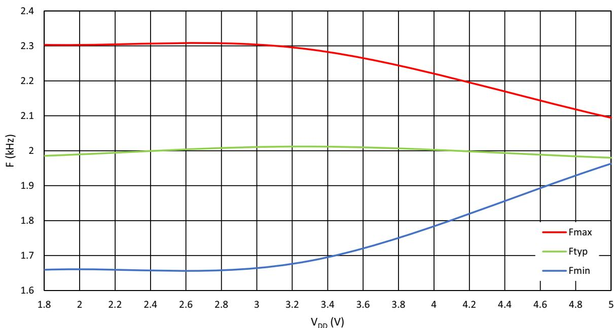
Figure 110: RC Oscillator Frequency vs. V<sub>DD</sub>, OSC = 2 MHz, T<sub>A</sub> = 25 °C
