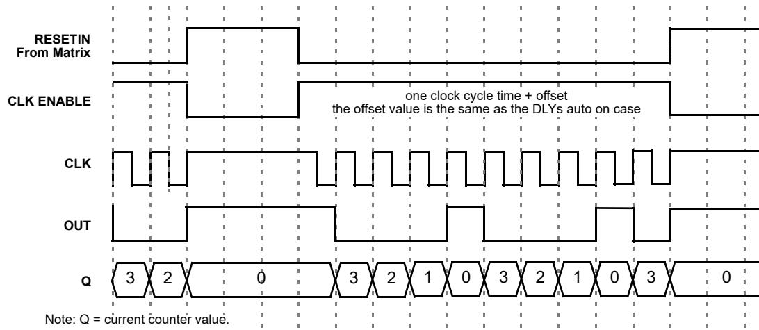
Figure 78: Timing (Reset High Level Mode, Oscillator is Autopowered on (Controlled by Reset)) for Count Data = 3
