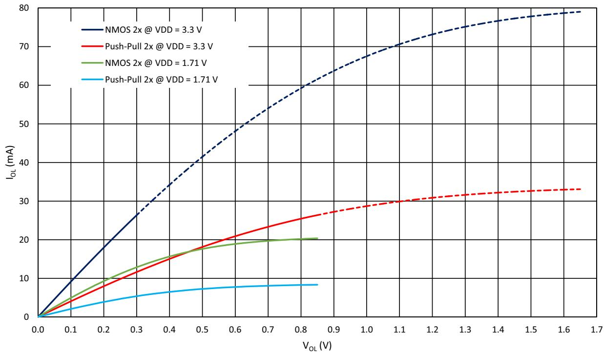
Figure 9: Typical Low Level Output Current vs. Low Level Output Voltage, 2x Drive at  $T_A = 25^\circ\text{C}$
