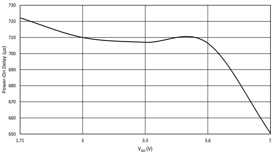
**Figure 104: LF Oscillator Maximum Power-On Delay vs. V<sub>DD</sub> at T<sub>A</sub> = 25 °C, OSC = 1.73 kHz**
