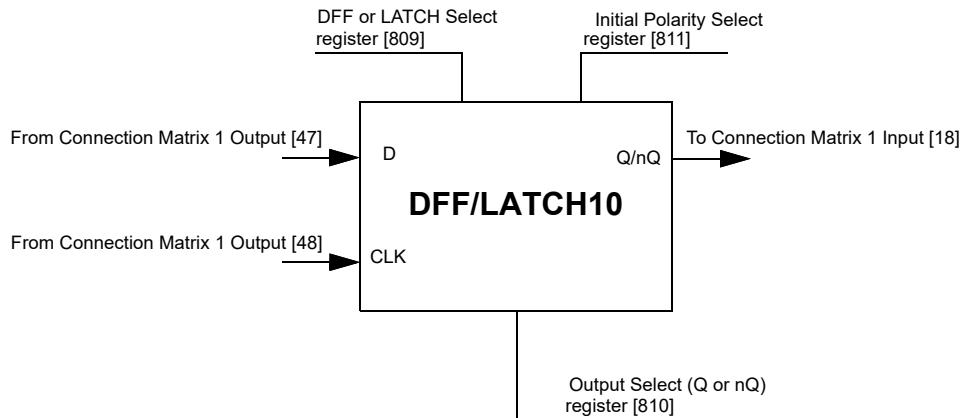
**Figure 59: DFF/LATCH10**
