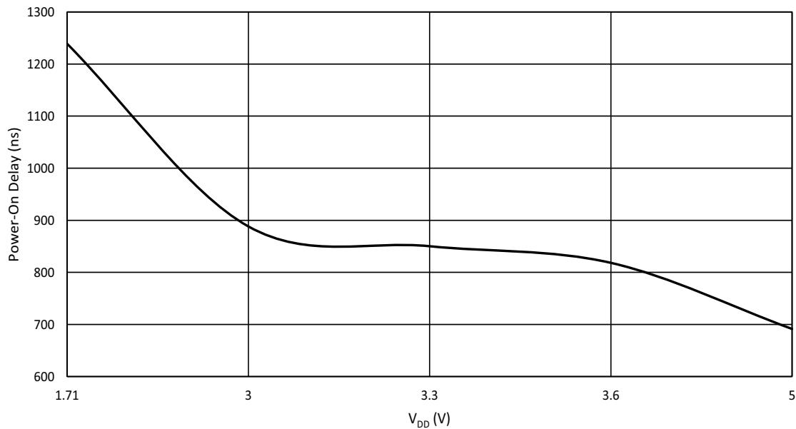
Figure 105: RC Oscillator Maximum Power-On Delay vs.  $V_{DD}$  at  $T_A = 25^\circ\text{C}$ , RC OSC = 2 MHz
