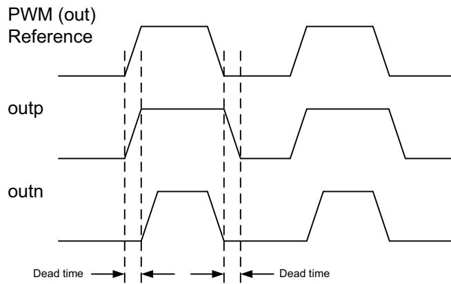
Figure 87: PWM Dead Band Control Timing Diagram
