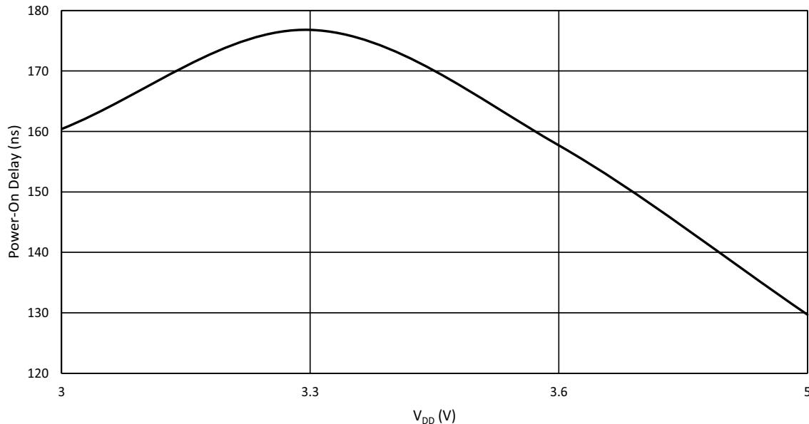
Figure 107: Ring Oscillator Maximum Power-On Delay vs.  $V_{DD}$  at  $T_A = 25^\circ\text{C}$ , OSC = 27 MHz**19.3 OSCILLATORS ACCURACY**
