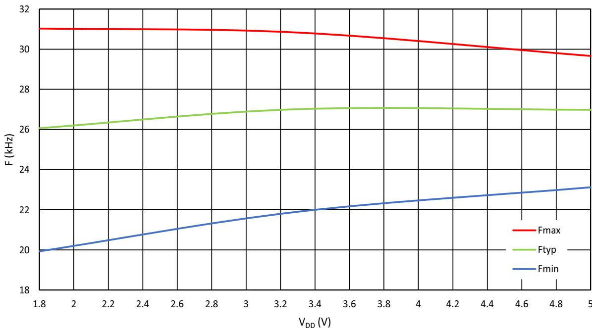
Figure 115: Ring Oscillator Frequency vs.  $V_{DD}$ , OSC = 27 MHz,  $T_A$  = -40 °C to 125 °C
