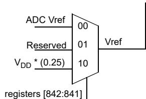
Figure 26: ADC Reference Voltage
