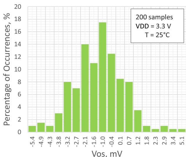
Figure 22: PGA Input Offset Distribution, Single-Ended Mode, G = 8
