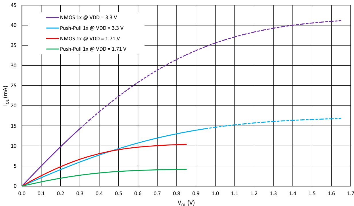
Figure 8: Typical Low Level Output Current vs. Low Level Output Voltage, 1x Drive at  $T_A = 25^\circ\text{C}$
