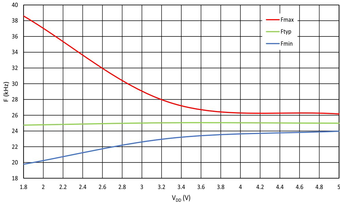
Figure 113: RC Oscillator Frequency vs. V<sub>DD</sub>, RC OSC = 25 kHz, T<sub>A</sub> = -40 °C to 125 °C
