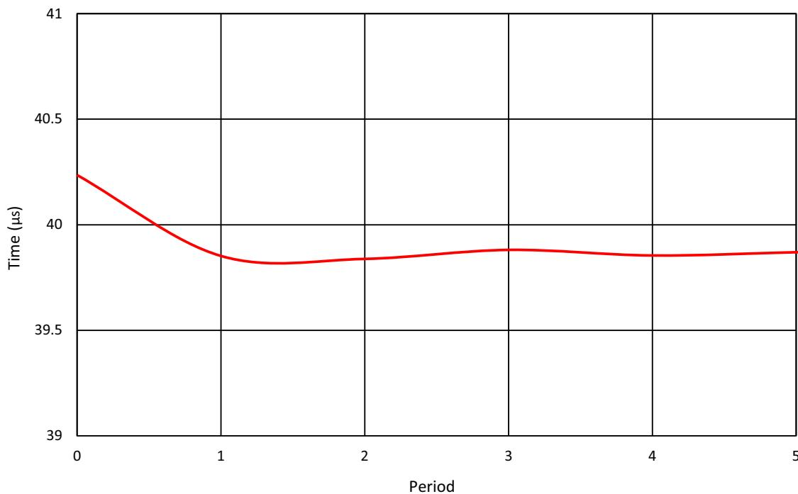
Figure 118: RC Oscillator Settling Time,  $V_{DD} = 3.3$  V,  $T_A = 25$  °C, OSC = 25 kHz
