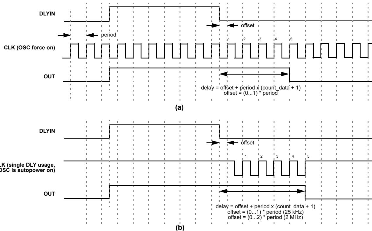
Figure 75: Timing (Falling Edge) for Count Data = 3: (a) Oscillator is in Force Power On Mode or an External Oscillator is Used, (b) Oscillator is in Auto Power On Mode
