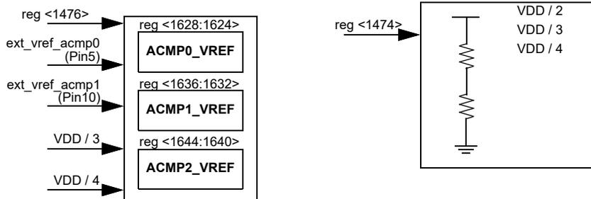
Figure 63. Voltage Reference Block Diagram
