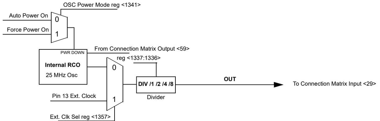
Figure 65. 25 MHz RC OSC Block Diagram
