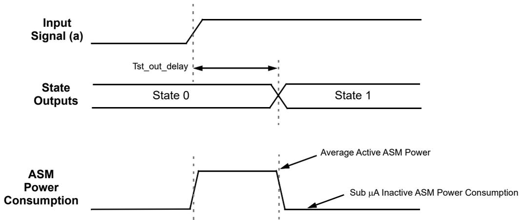
Figure 87. State Transition Timing and Power Consumption
