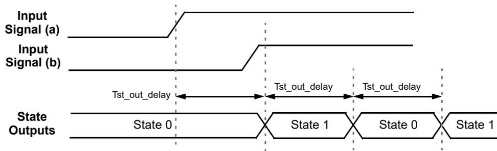
Figure 96. State Transition - Closed Cycling Timing
