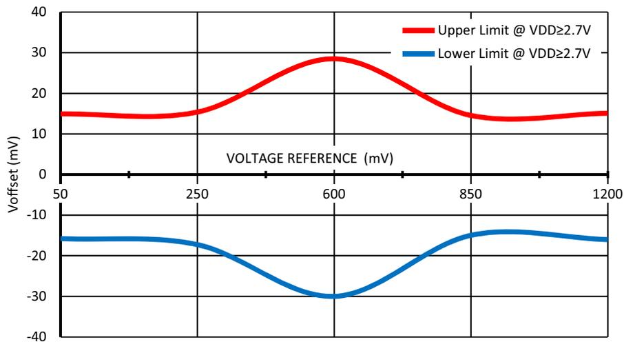
**Figure 54. Typical Buffer Input Voltage Offset vs. Voltage Reference at T = (-40... +85) °C, Buffer Bandwidth = 1 kHz, V<sub>phys</sub> = 0 mV, Gain = 1.**
