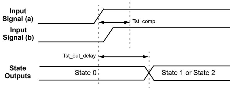
Figure 91. State Transition Timing - Competing Inputs Indeterminate
