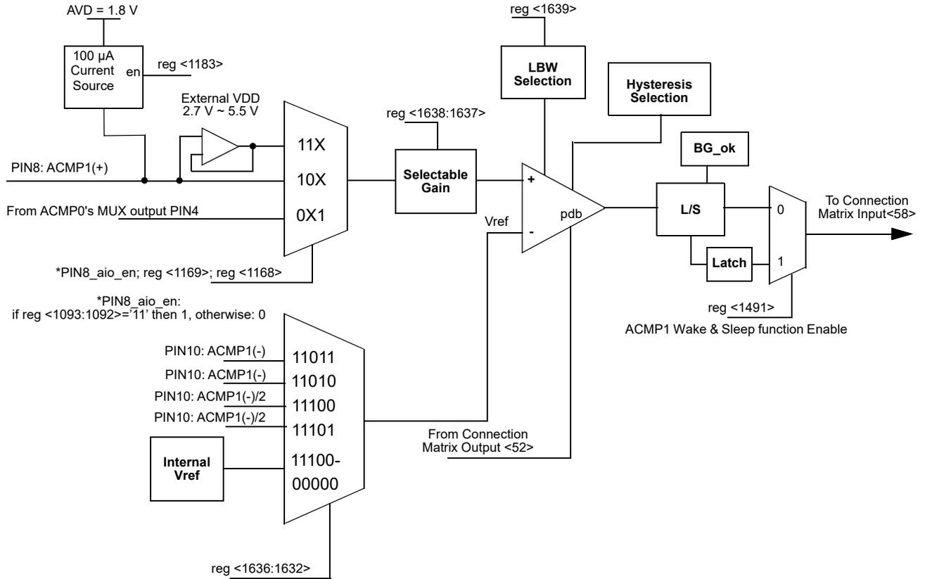
Note: when 100  $\mu$ A Current Source is enabled input voltage on Pin 8 should not exceed 1.8 V.
