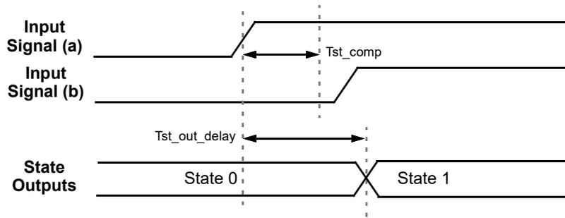
Figure 92. State Transition Timing - Competing Inputs Determinable
