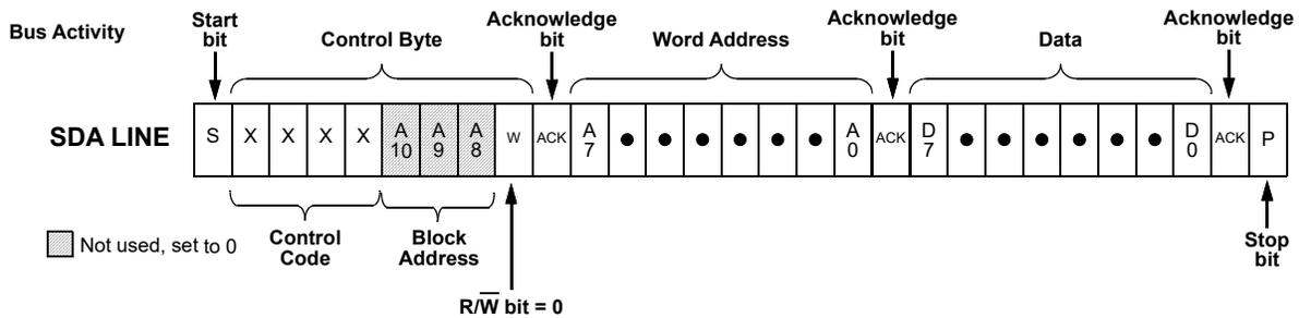
Figure 99. Byte Write Command, R/W = 0
