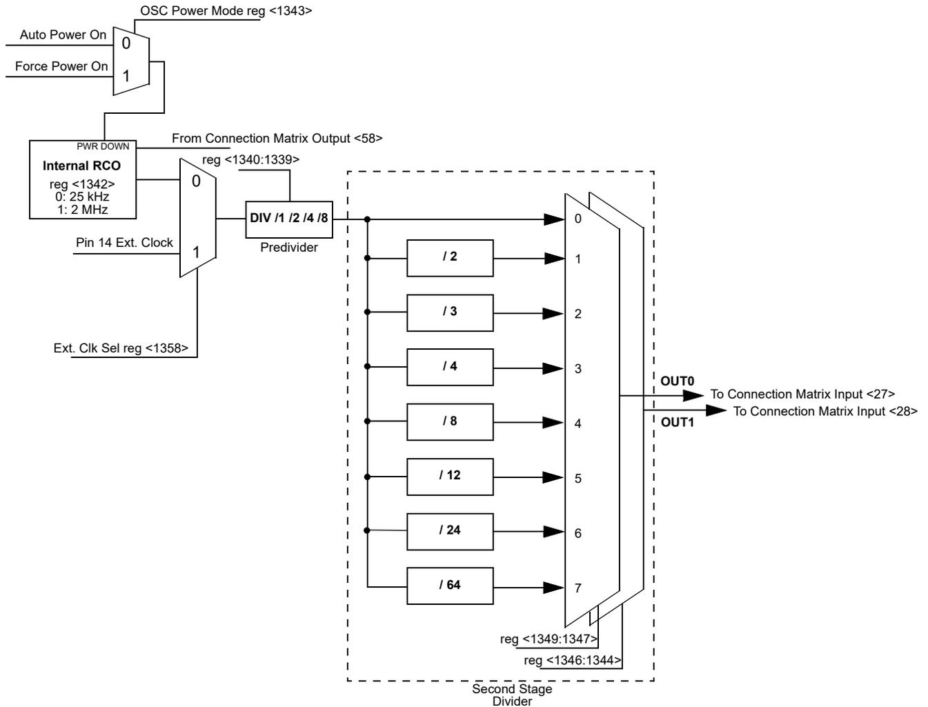
Figure 64. 25 kHz / 2MHz RC OSC Block Diagram
