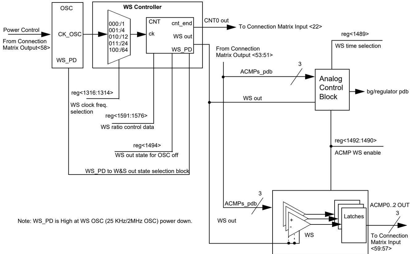
Note: WS\_PD is High at WS OSC (25 KHz/2MHz OSC) power down.
