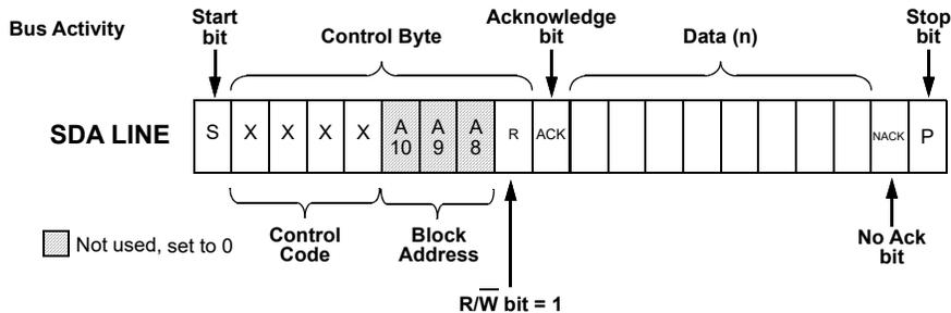
Figure 101. Current Address Read Command,  $\overline{R/W} = 1$
