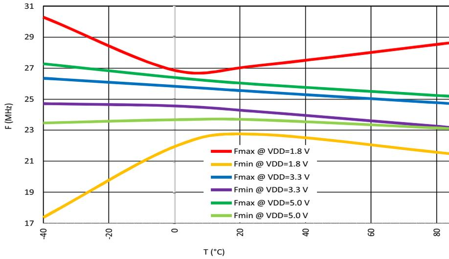
**Figure 72. OSC1 (25 MHz) Frequency vs. Temperature**
