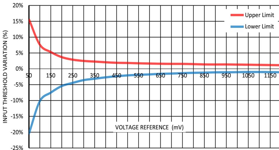
Figure 55. Typical Input Threshold Variation (including Vref variation, ACMP offset) vs. Voltage Reference at T = (-40.... +85) °C, LMB Mode - Disable, V<sub>hys</sub> = 0 mV.
