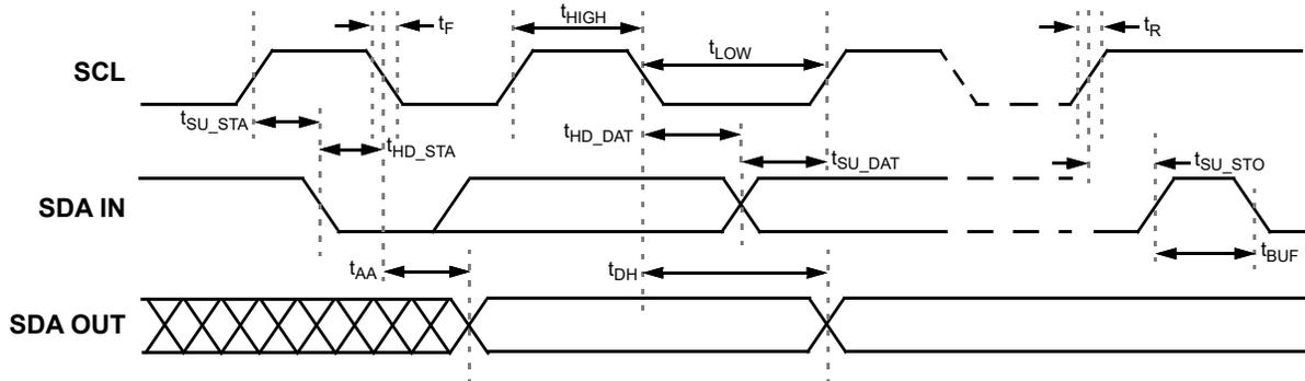
Figure 98. I<sup>2</sup>C General Timing Characteristics
