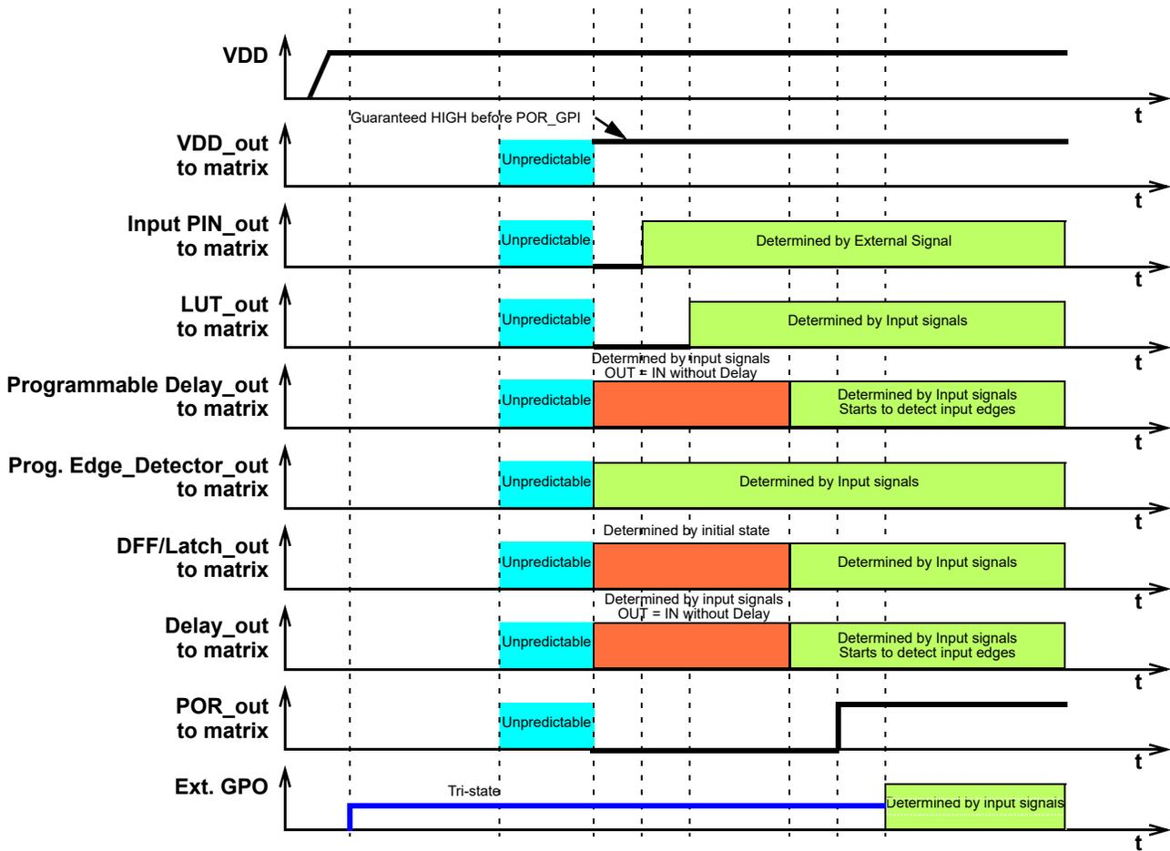
Figure 76. Internal Macrocell States during POR sequence
