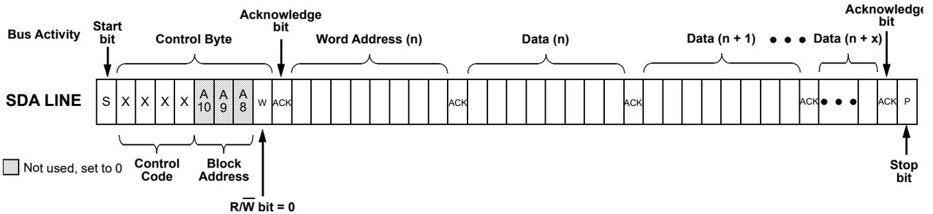
Figure 100. Sequential Write Command,  $\overline{R/W} = 0$
