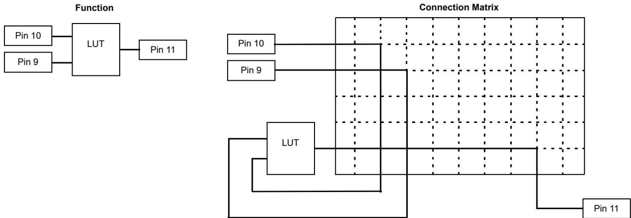
Figure 11. Connection Matrix Example
