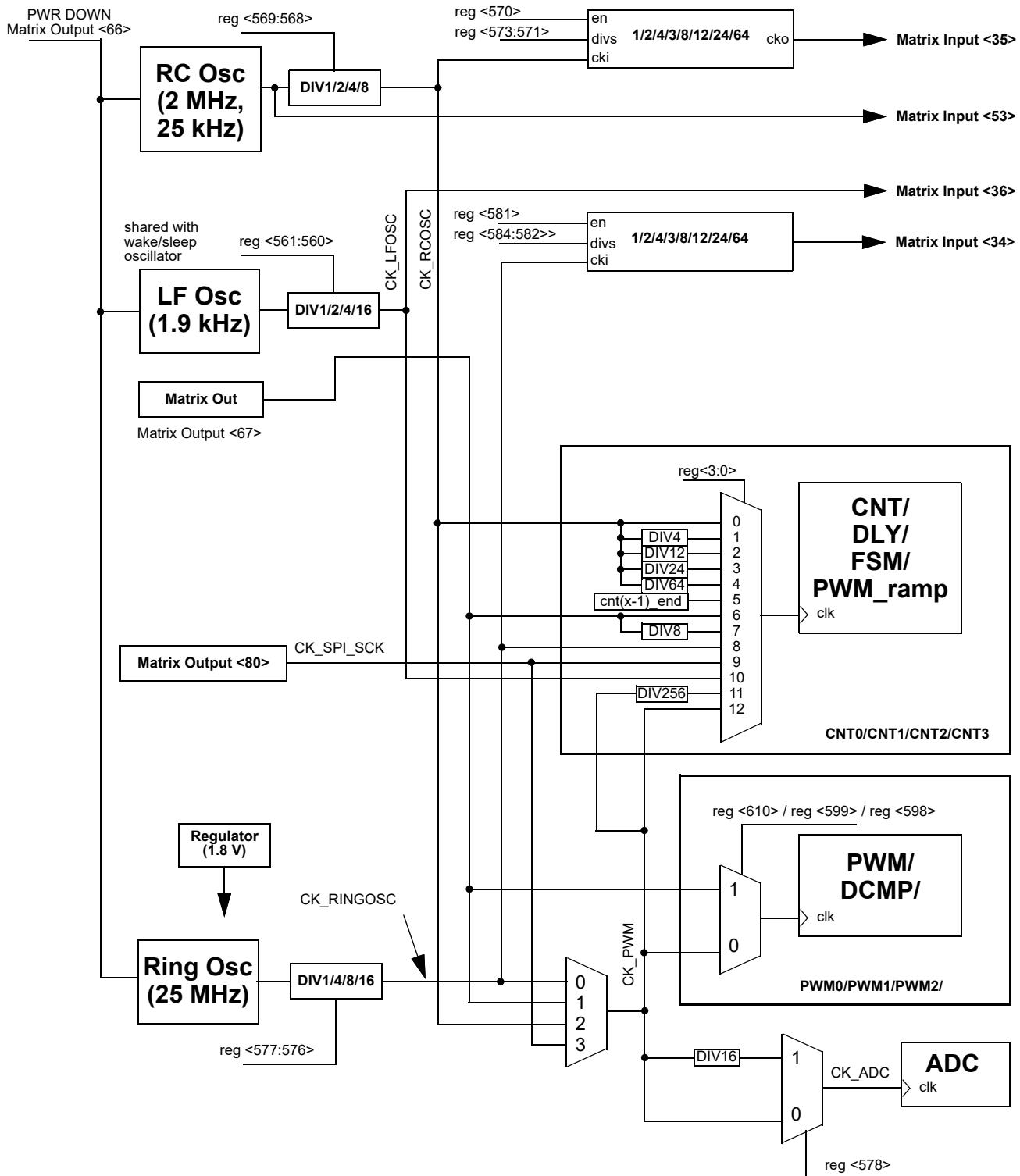
Figure 84. Oscillator Block Diagram
