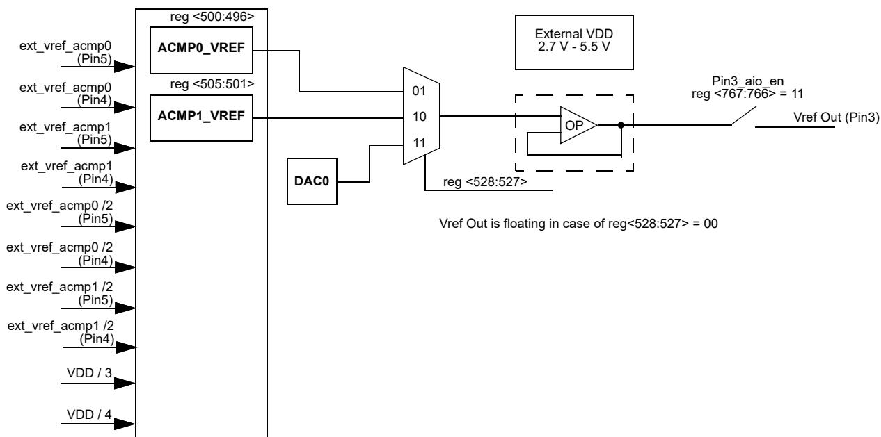
**Figure 83. Voltage Reference Block Diagram**
