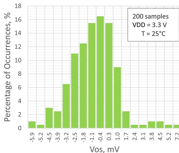
Figure 14. PGA Input Offset Distribution, Single-Ended Mode,  $G = 2$
