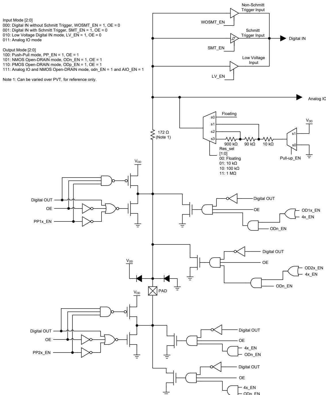
Figure 6. Register OE IO 4x Drive Structure Diagram
