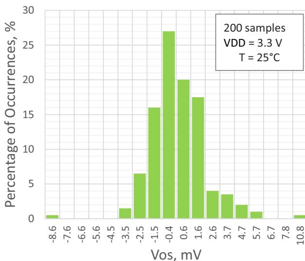
Figure 13. PGA Input Offset Distribution, Single-Ended Mode,  $G = 1$
