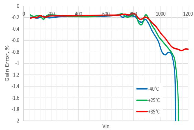
**Figure 30. Typical PGA Gain Error vs. Vin, Pseudo-Differential Mode, G = 1, VDD = 5.5 V**
