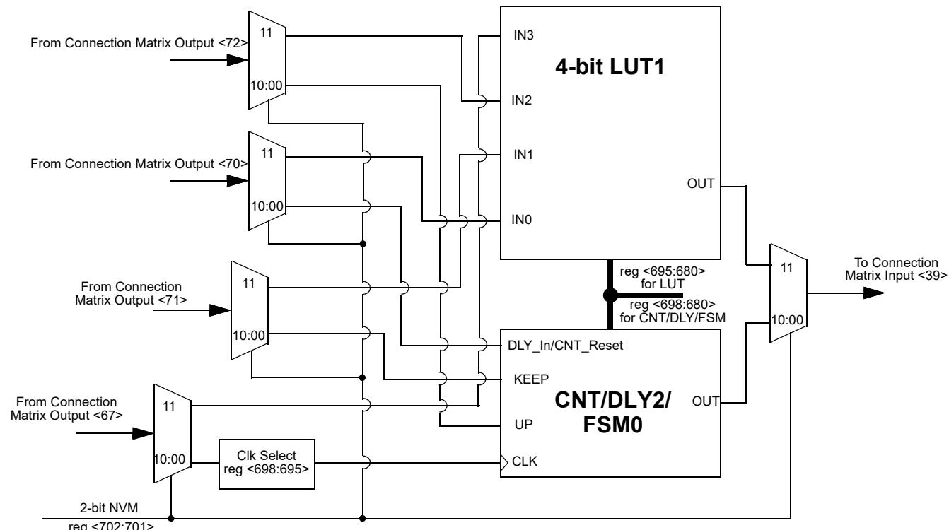
Figure 48. 4-bit LUT1 or CNT/DLY2/FSM0
