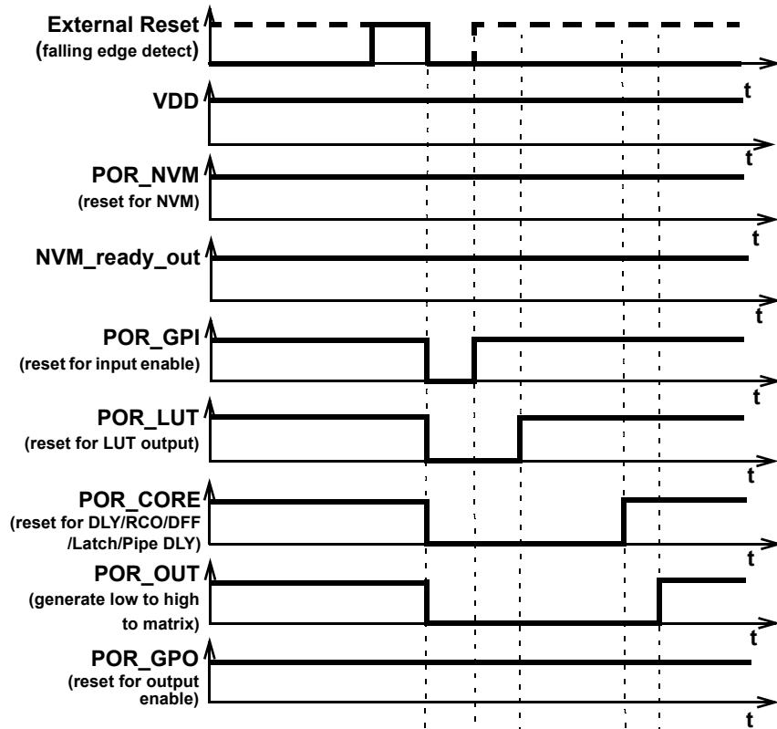
Figure 99. External reset sequence (Falling edge detect)
