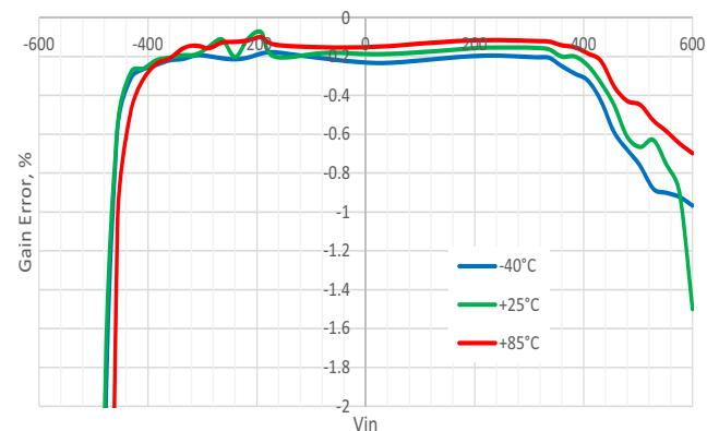
**Figure 22. Typical PGA Gain Error vs.  $V_{in}$ , Differential Mode,  $G = 1$ ,  $VDD = 1.71$  V**
