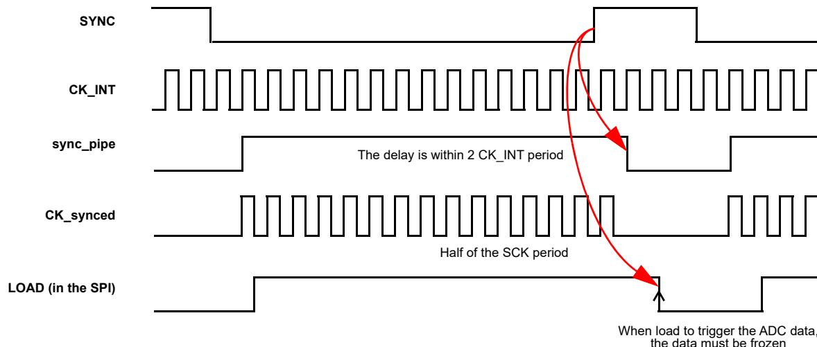
**Figure 76. Timing Diagram showing SPI Clock synchronization**
