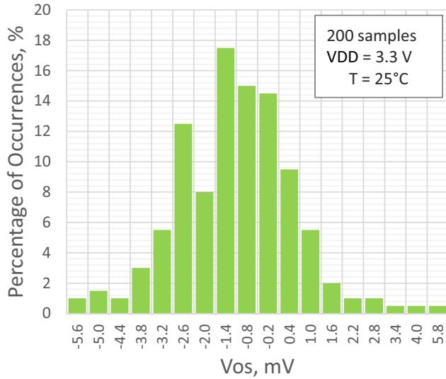
Figure 15. PGA Input Offset Distribution, Single-Ended Mode, G = 4
