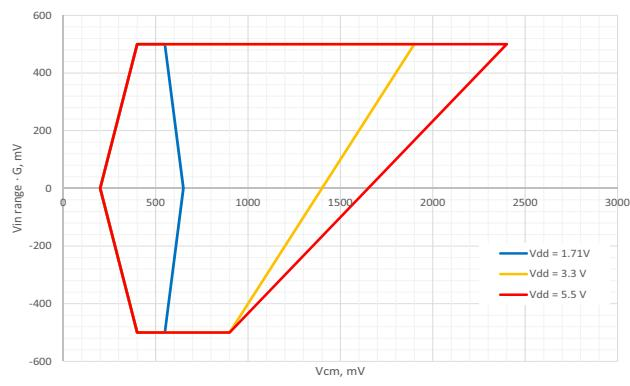
**Figure 21. PGA Input Vind Range Multiplied by Gain vs.  $V_{cm}$ , Differential Mode**
