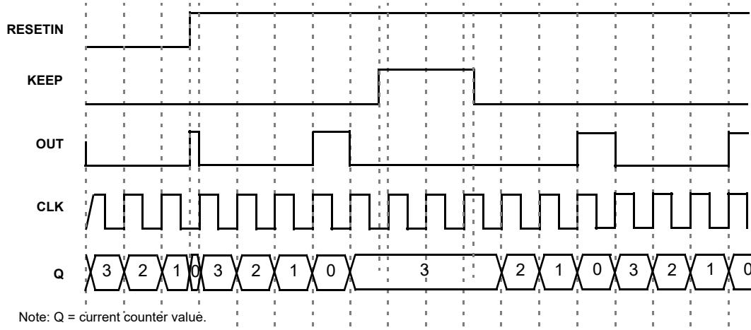
Figure 64. CNT/FSM Timing Diagram (reset rising edge mode, oscillator is forced on, UP = 0) for counter data = 3
