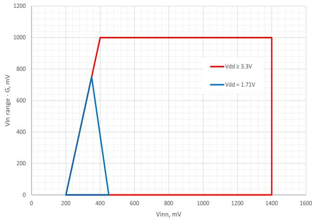
**Figure 27. PGA Input Vind Range Multiplied by Gain vs. Vinn, Pseudo-Differential Mode, G = 2**
