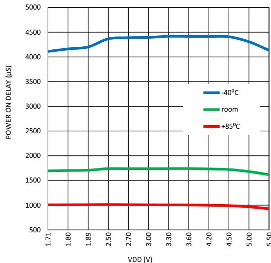
**Figure 49. Maximum Power On Delay vs. VDD,
