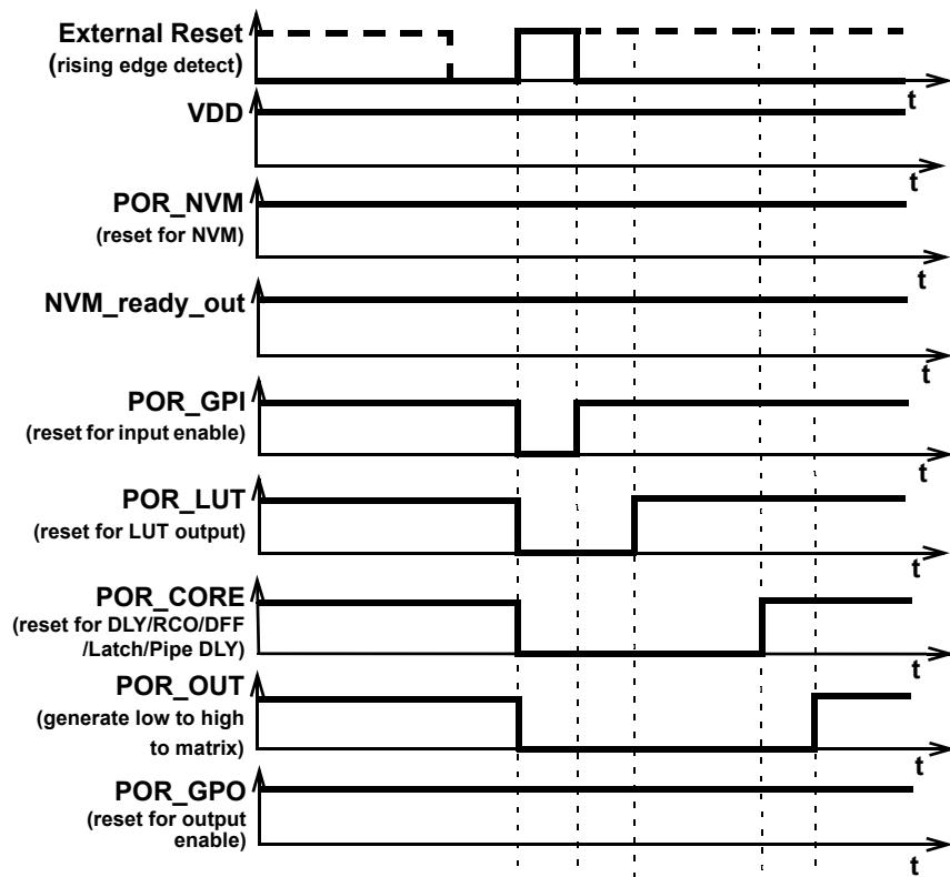
Figure 98. External reset sequence (Rising edge detect)
