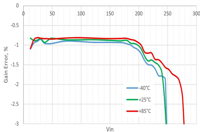
**Figure 31. Typical PGA Gain Error vs. Vin,
