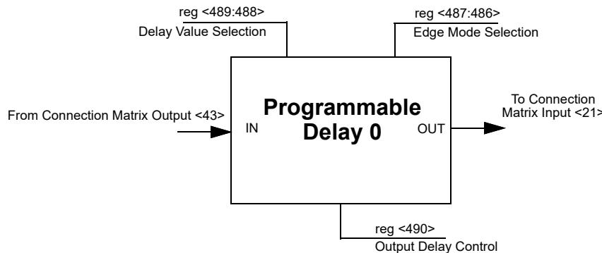
Figure 79. Programmable Delay
