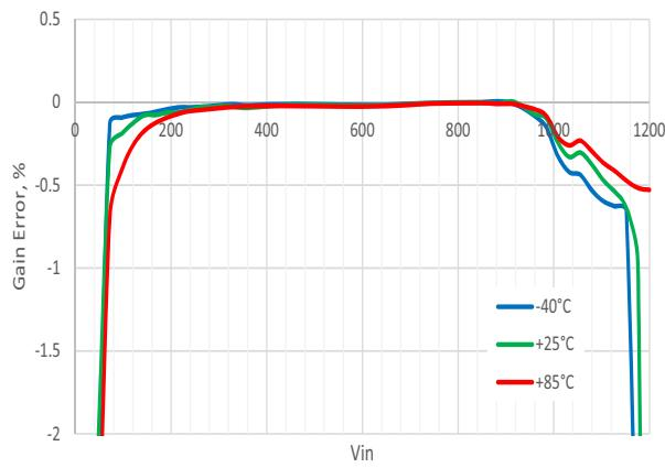
Figure 17. Typical PGA Gain Error vs. Vin, Single-Ended Mode, G = 1, VDD = 1.71 V
