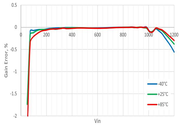
Figure 18. Typical PGA Gain Error vs. Vin, Single-Ended Mode, G = 1, VDD = 5.5 V
