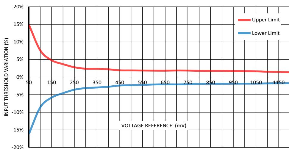
**Figure 51. Input Threshold Variation (including Vref variation, ACMP offset) vs. Voltage reference at T = (-40 ... +85)°C, LBW Mode - Disable, V<sub>hys</sub> = 0 mV**
