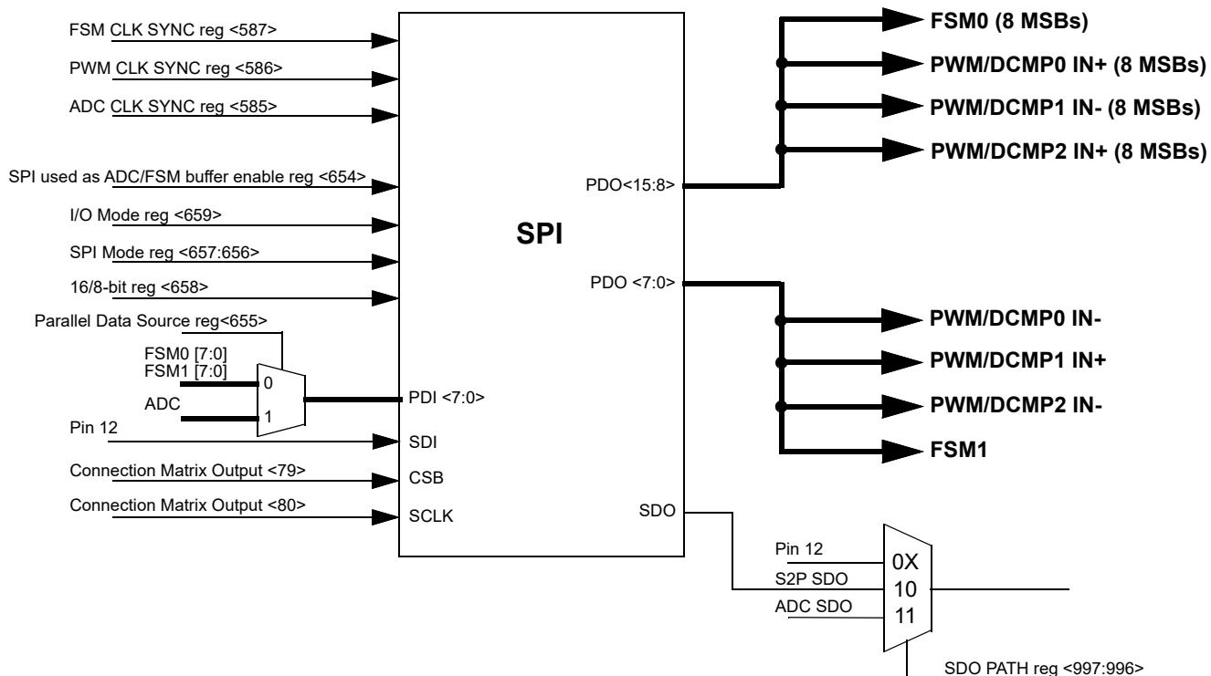
Figure 73. SPI Functional Diagram
