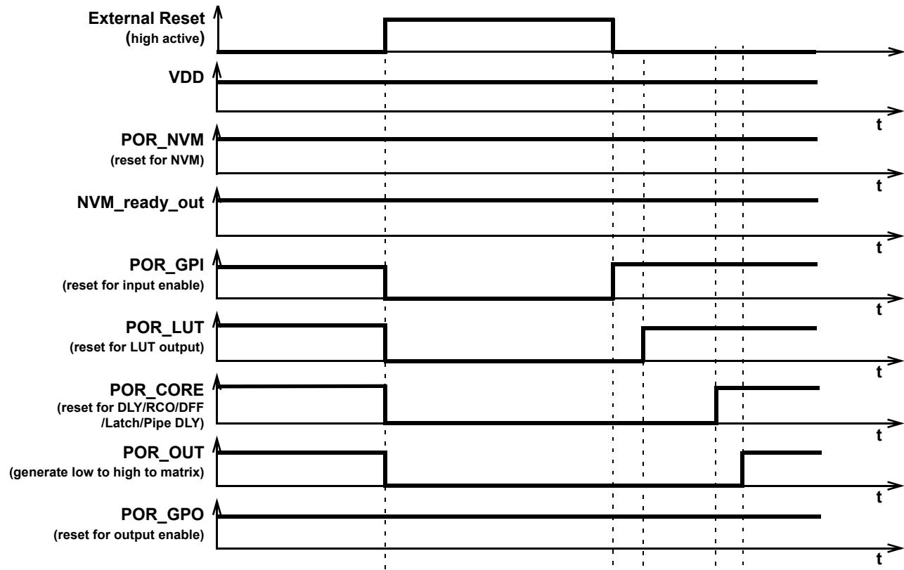
Figure 97. External reset sequence (High active)
