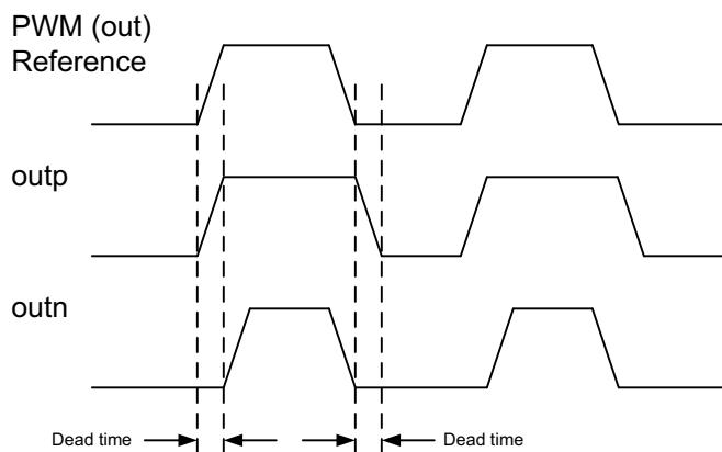
Figure 72. PWM Dead Band Control Timing Diagram
