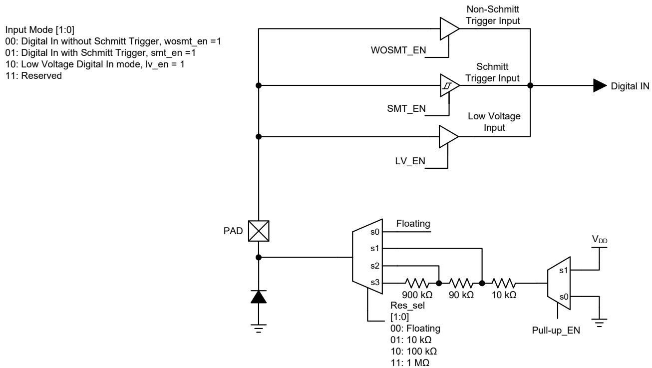
Figure 2. PIN 2 GPI IO Structure Diagram
