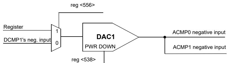
Figure 37. DAC1 Functional Diagram
