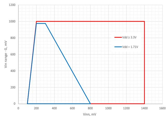
**Figure 26. PGA Input Vin Range Multiplied by Gain vs. Vinn, Pseudo-Differential Mode,  $G = 1$**
