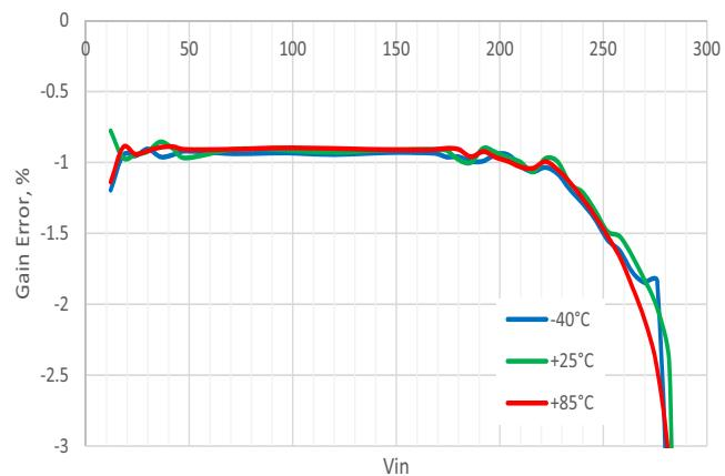
**Figure 32. Typical PGA Gain Error vs. Vin,
