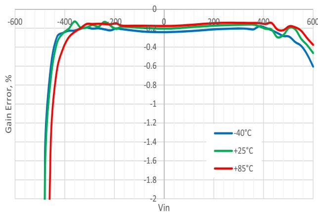
**Figure 23. Typical PGA Gain Error vs. Vin, Differential Mode,  $G = 1$ ,  $VDD = 5.5$  V**
