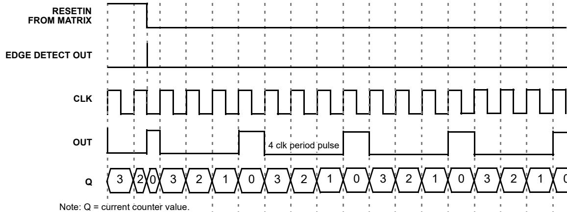
Figure 62. Timing (reset falling edge mode, oscillator is forced on) for count data = 3
