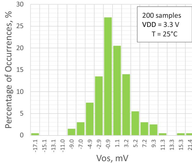
Figure 12. PGA Input Offset Distribution, Single-Ended Mode,  $G = 0.5$
