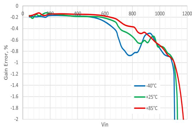
**Figure 29. Typical PGA Gain Error vs. Vin, Pseudo-Differential Mode, G = 1, VDD = 2.0 V**
