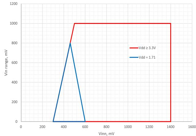
**Figure 28. PGA Input Vind Range Multiplied by Gain vs. Vinn, Pseudo-Differential Mode, G = 4**
