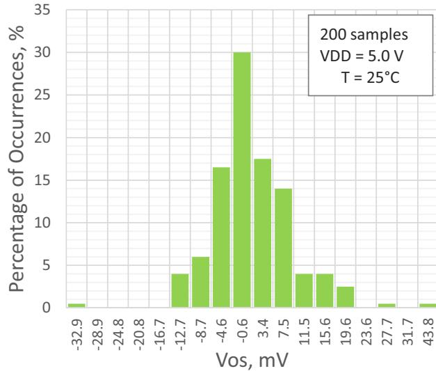
Figure 11. PGA Input Offset Distribution, Single-Ended Mode,  $G = 0.25$
