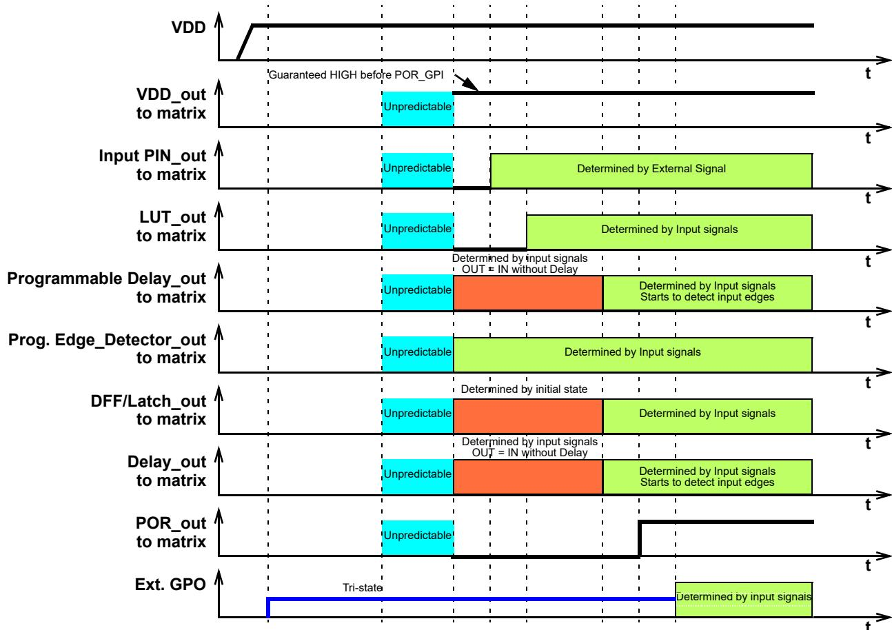
Figure 95. Internal Macrocell States during POR sequence
