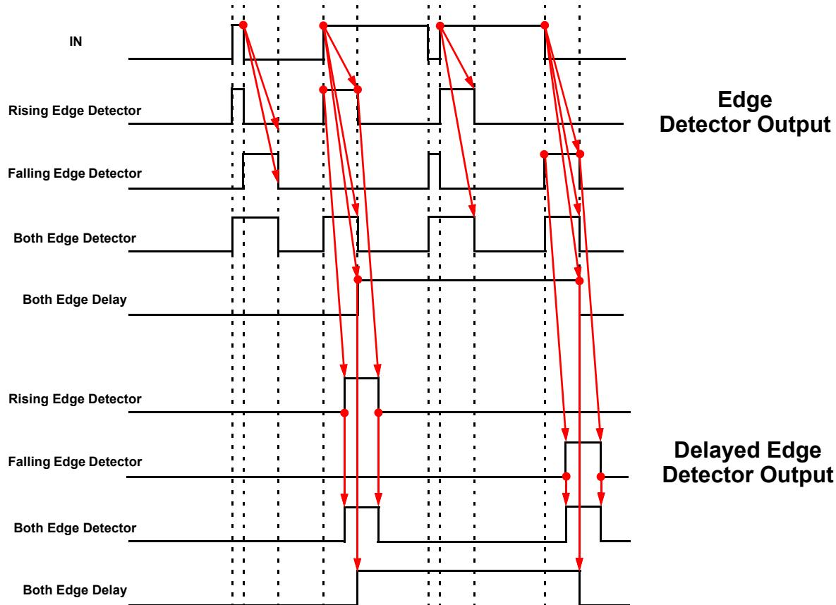
Figure 82. Glitch Filtering for Edge Detector Output
