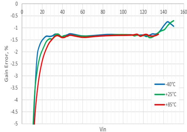
**Figure 20. Typical PGA Gain Error vs.  $V_{in}$ , Single-Ended Mode,  $G = 8$ ,  $VDD = 5.5$  V**
