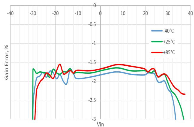
**Figure 24. Typical PGA Gain Error vs. Vin, Differential Mode,  $G = 16$ ,  $VDD = 1.71$  V**
