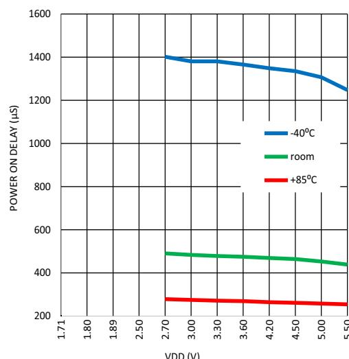
**Figure 50. Maximum Power On Delay vs. VDD,
