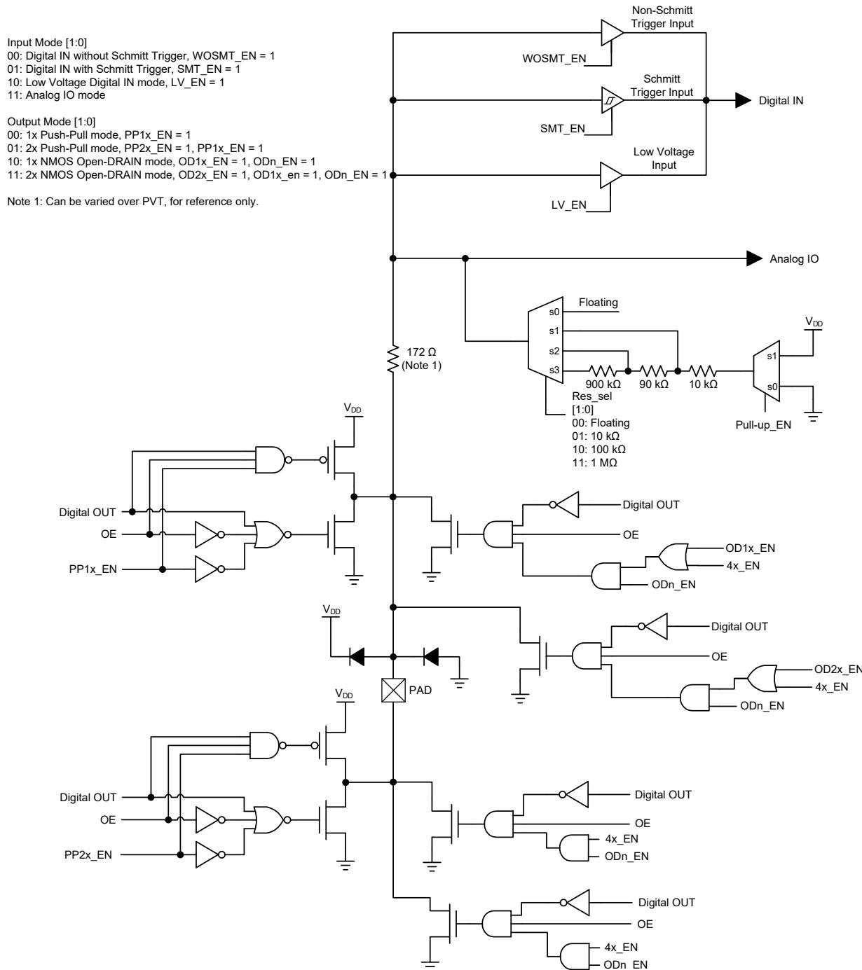
Figure 4. Matrix OE IO 4x Drive Structure Diagram
