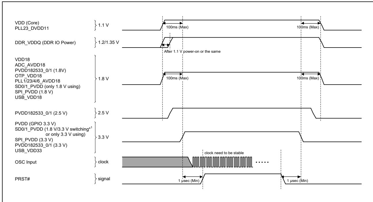
Figure 3.1 Power-On/Power-Off Sequence
