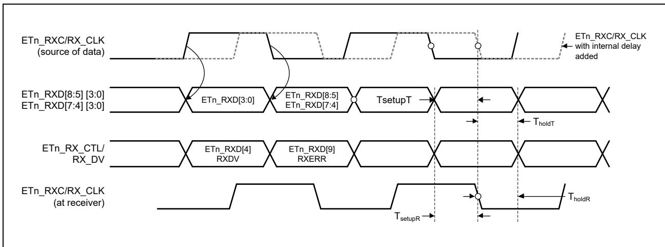
Figure 3.20 Multiplexing &amp; Timing Diagram — RGMII-ID (Receiver)
