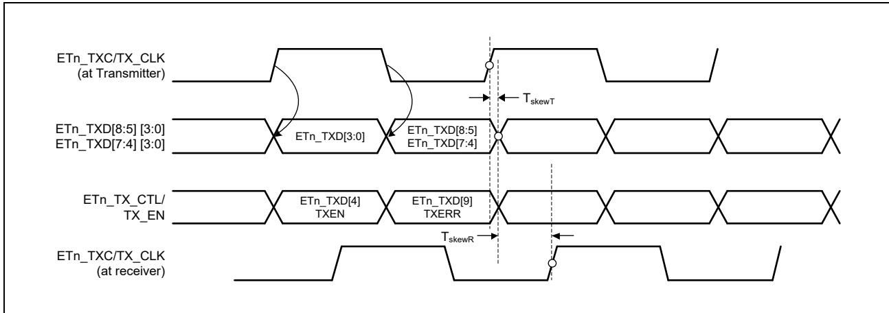
Figure 3.19 Multiplexing &amp; Timing Diagram — RGMII (Transmitter)
