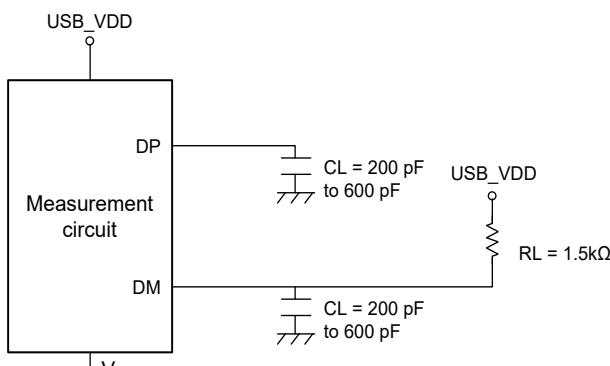
Figure 3.12 Measurement Circuit (Low-Speed)
