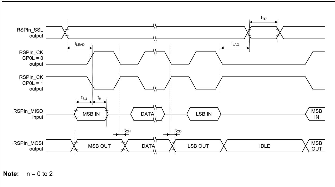
Figure 3.45 Transmission and Reception Timing (Master, CPHA = 0)
