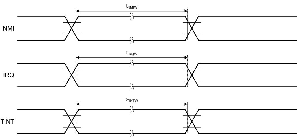
**Note:** This specification “(Min. 20  $t_{cycle}$ )” is the min. pulse width the case that the digital noise filter is off. For details on digital noise filter settings, refer to *Section 41, General Purpose Input Output Port (GPIO)*, in the *User's Manual: Hardware*.
