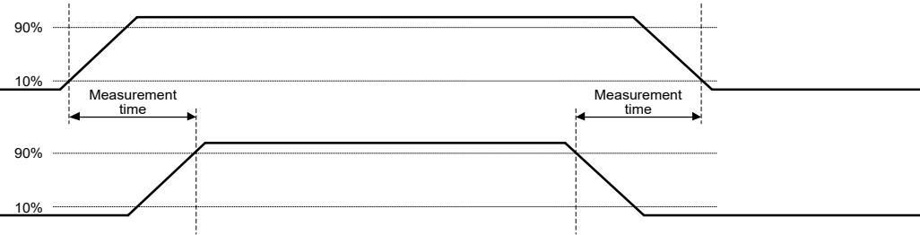
**Note:** In case of there is restriction of sequence between different power supply, measurement time is starting point that is 10% of earlier rising power voltage level to end point that is 90% of later rising power voltage level, and starting point that is 90% of earlier falling power voltage level to end point that is 10% of later falling power voltage level.
