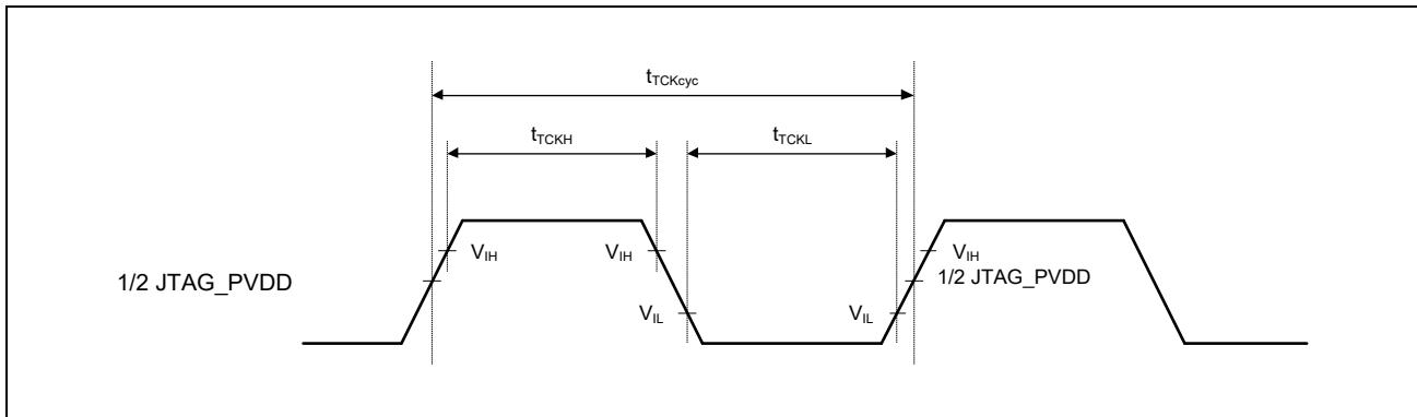
Figure 3.21 TCK\_SWDCLK Input Timing
