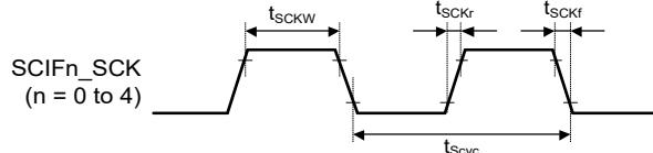
Figure 3.40 SCK Input Clock Timing
