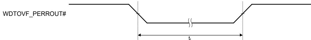
Figure 3.50 Watchdog Timer Output Timing
