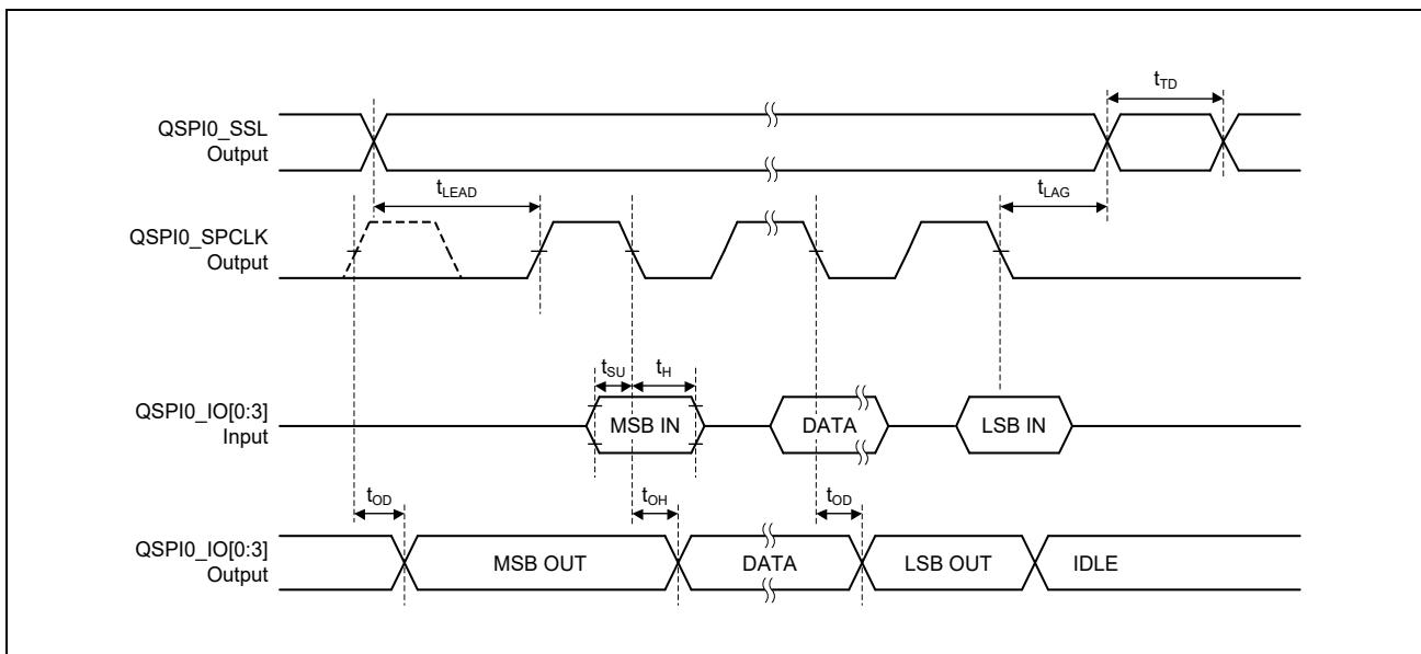
Figure 3.25 SDR Transfer Format Transmission and Reception Timing
