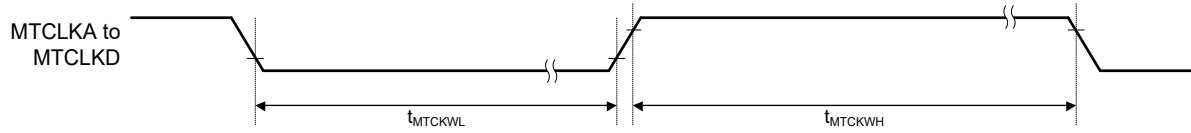
Figure 3.37 MTU3a Clock Input Timing
