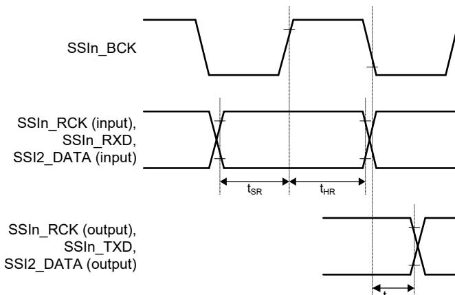
Figure 3.32 Transmission and Reception Timing (SSIBCK Falling Output)
