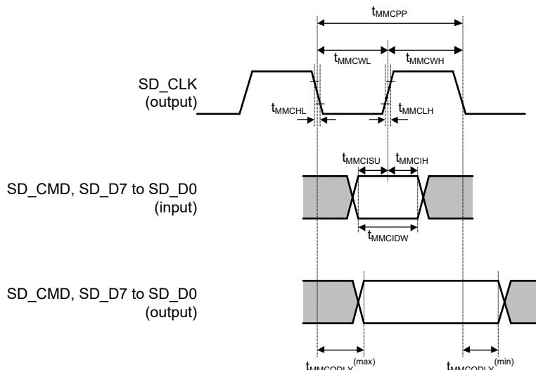
Figure 3.10 eMMC Host Interface (MMC Interface HS200 Mode 1.8-V Power Supply Selection)
