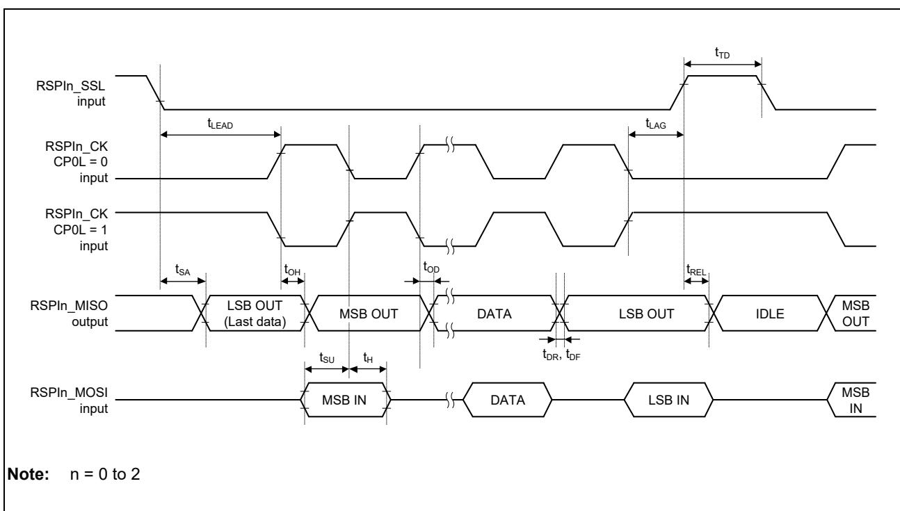
Figure 3.48 Transmission and Reception Timing (Slave, CPHA = 1)
