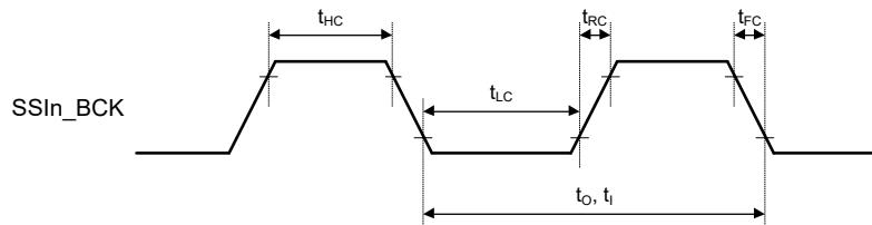
Figure 3.31 Bit Clock Input/Output Timing
