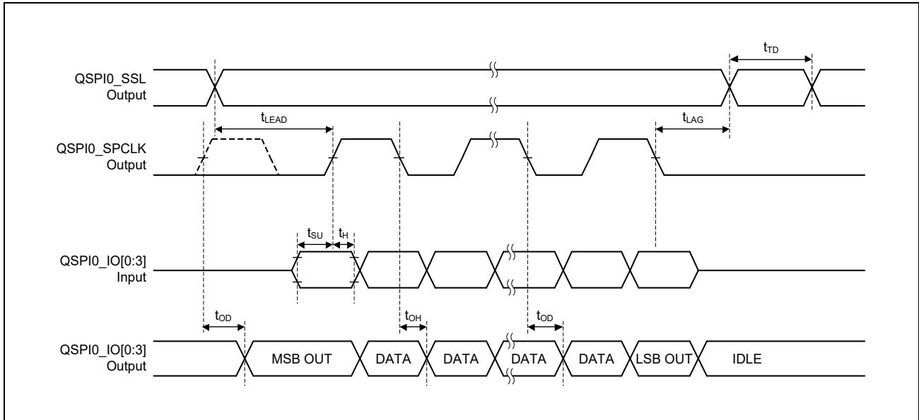
Figure 3.26 DDR Transfer Format Transmission and Reception Timing
