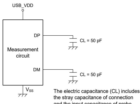
Figure 3.14 Measurement Circuit (Full-Speed)
