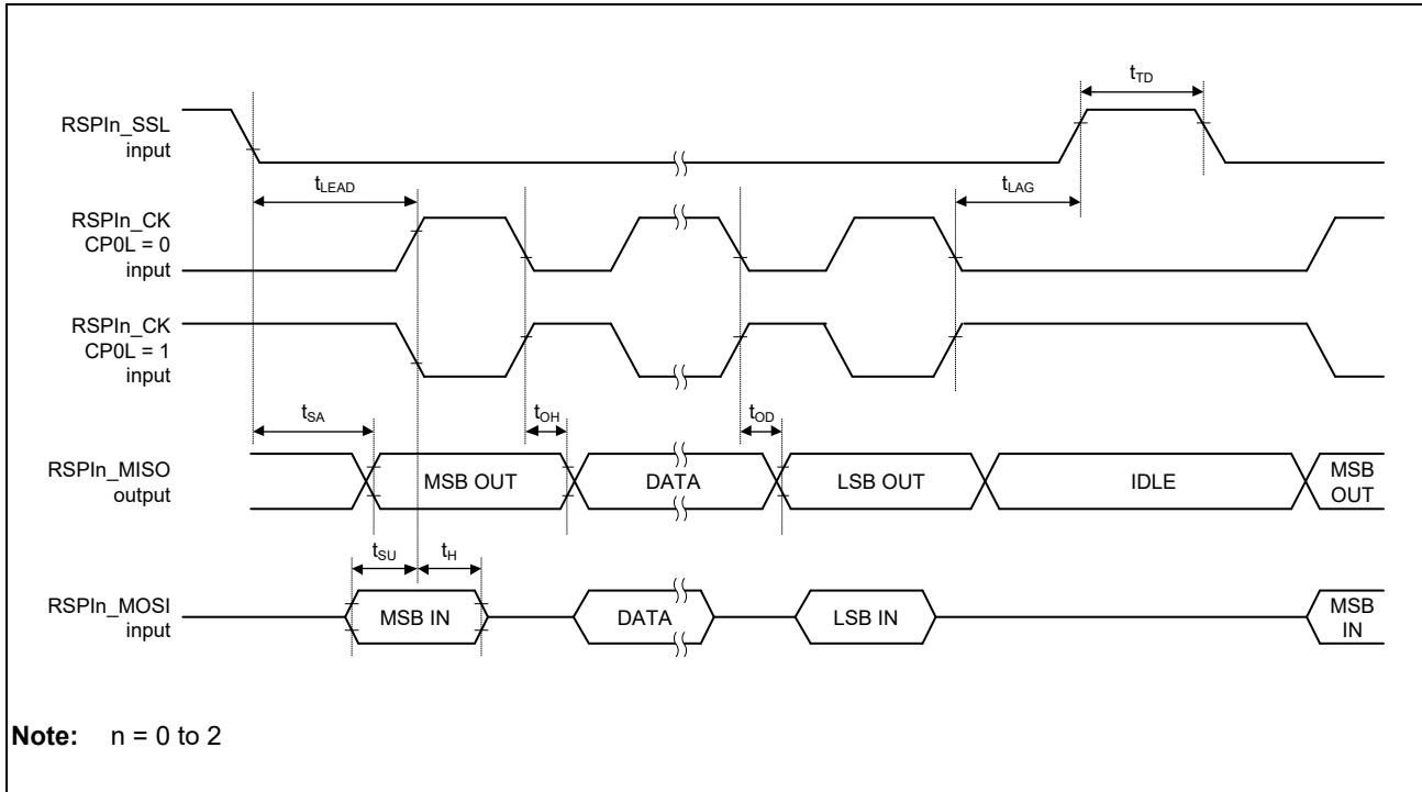
Figure 3.47 Transmission and Reception Timing (Slave, CPHA = 0)
