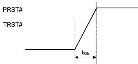
Figure 3.29 Reset Input Timing 2
