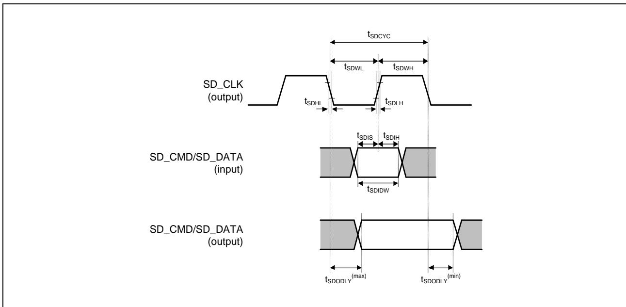
Figure 3.8 SDHC Interface Timing (SDR 3.3-V Power Supply)
