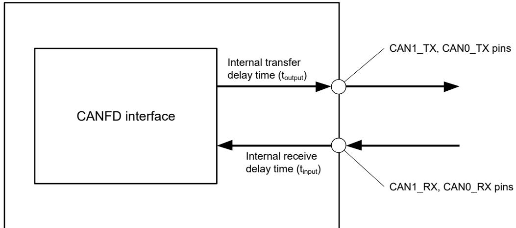
Figure 3.35 CAN-FD Interface Condition
