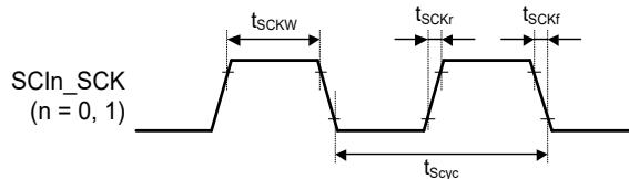
Figure 3.42 SCK Input Clock Timing
