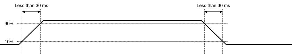
**Note:** The rise/fall time of each power supply should be within 30 msec.
