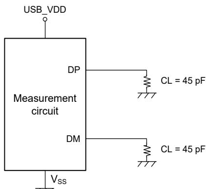
Figure 3.16 Measurement Circuit (Hi-Speed)
