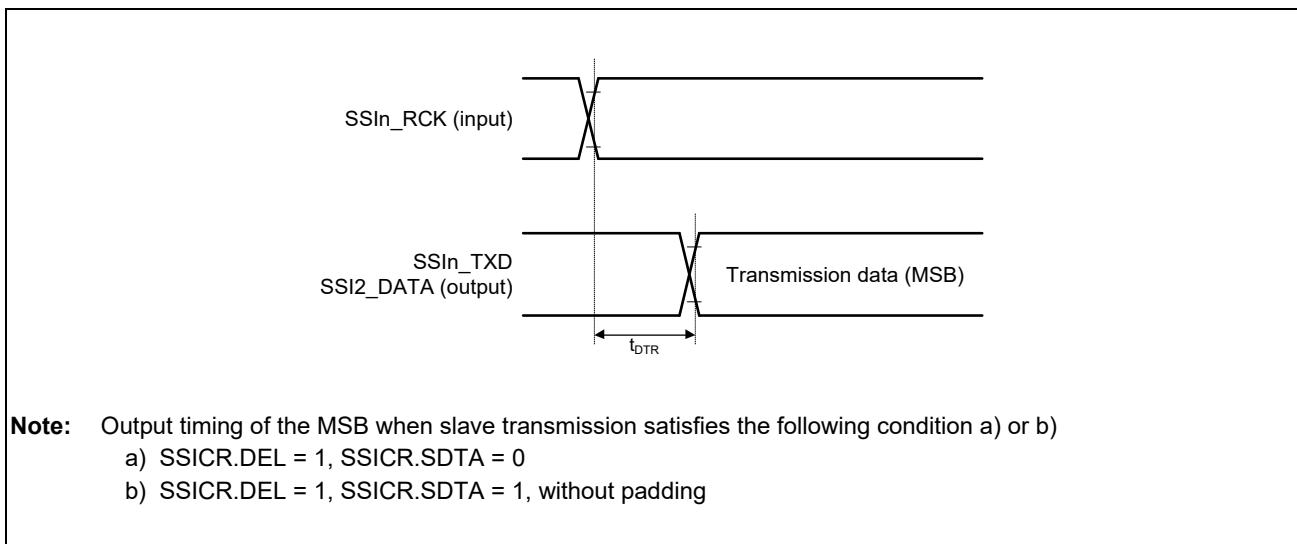
Figure 3.34 Transmission Timing (Slave, in Synchronization with SSILRCK)
