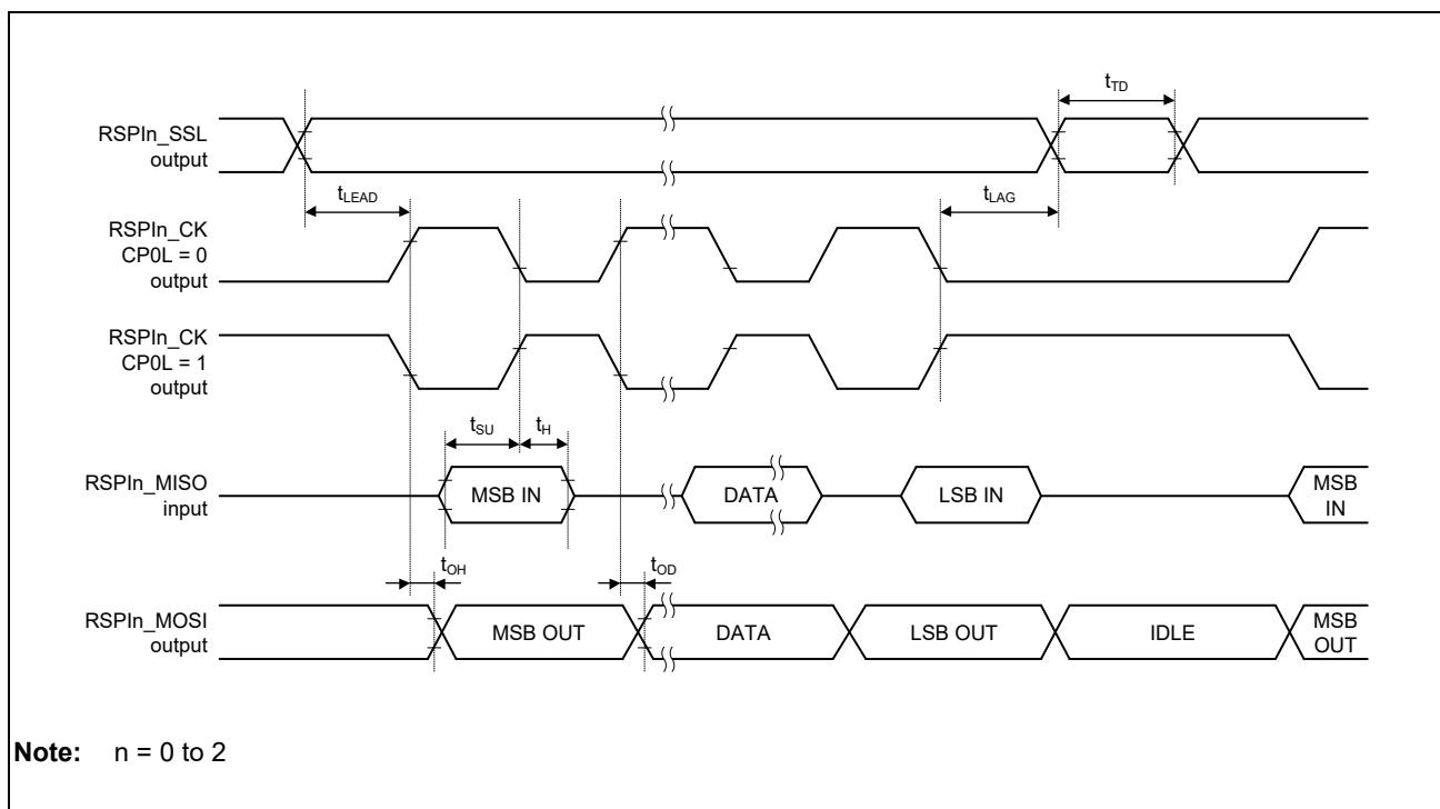
Figure 3.46 Transmission and Reception Timing (Master, CPHA = 1)
