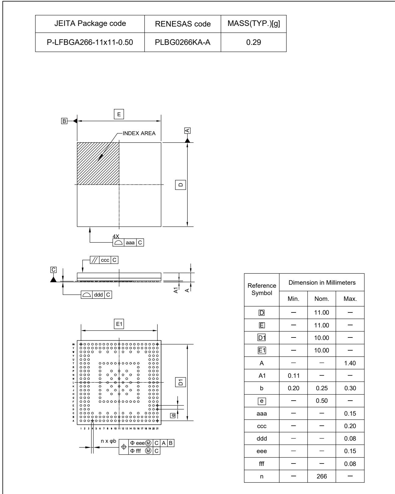
Figure 4.2 Package Dimensions for LFBGA 11 mm□/0.5 mm pitch/266 pin
