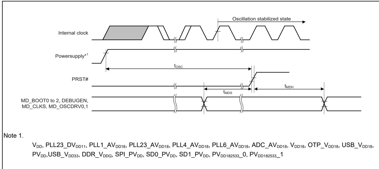
Figure 3.6 Power-On Oscillation Settling Time
