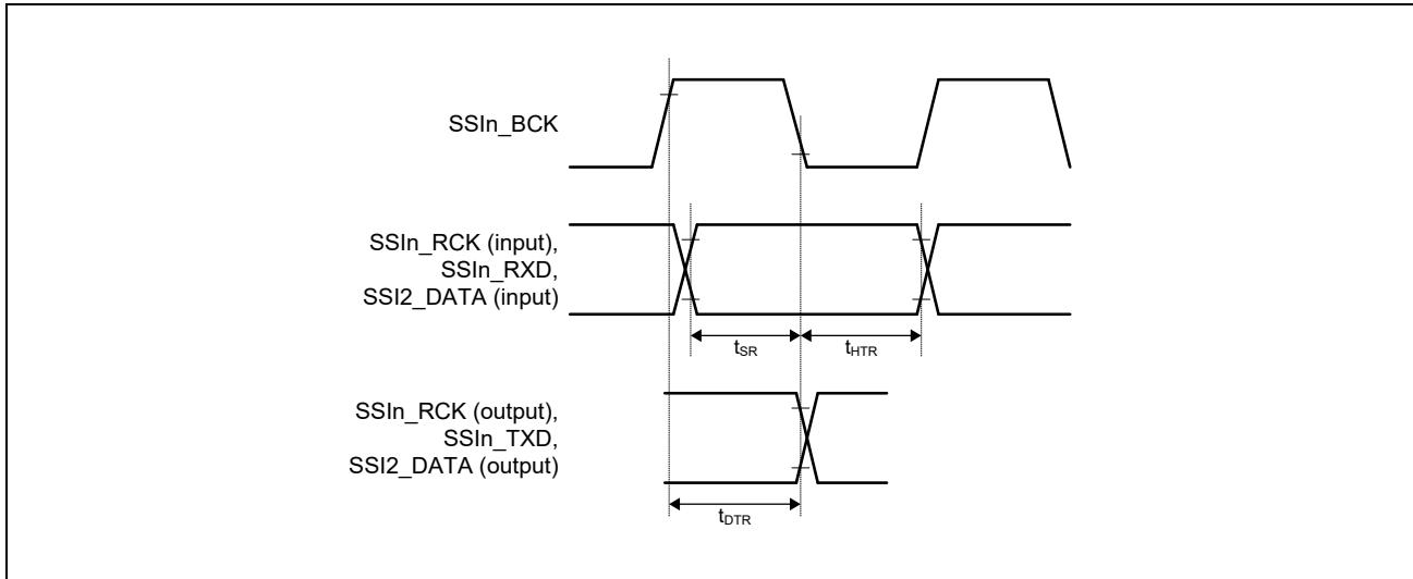
Figure 3.33 Transmission and Reception Timing (SSIBCK Rising Output)
