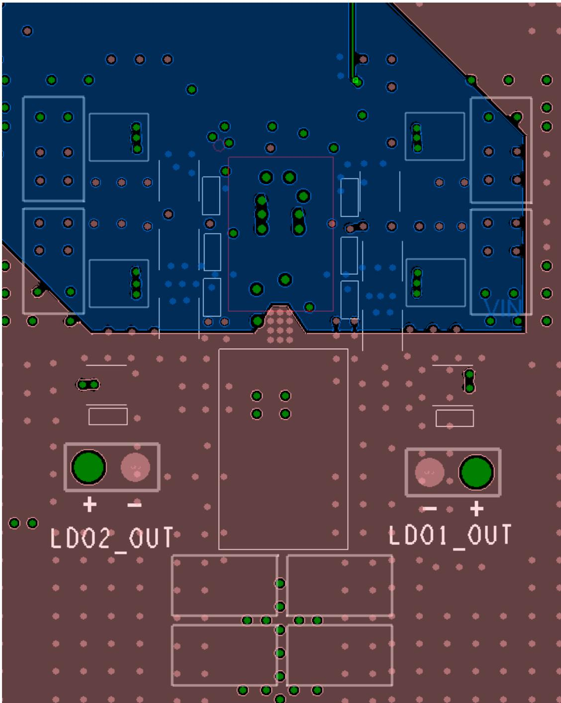
Figure 36. PCB Example 2, Inner Layer VIN and GND Copper
