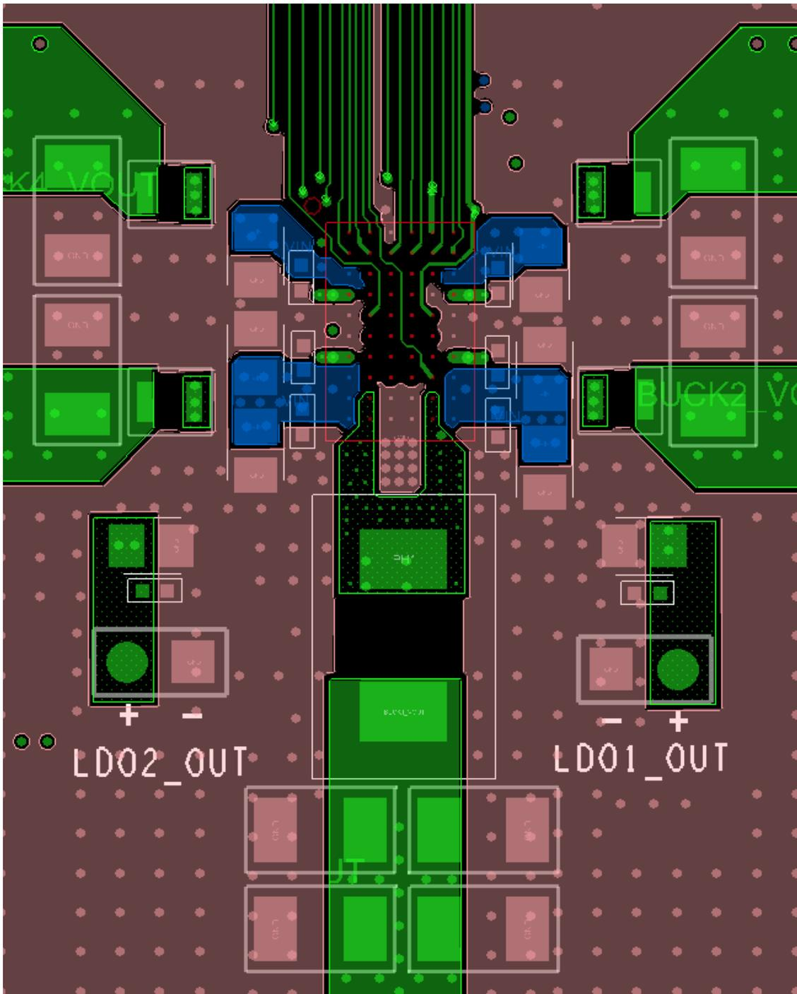
Figure 34. PCB Example 2, Top Layer with Staggered Vias
