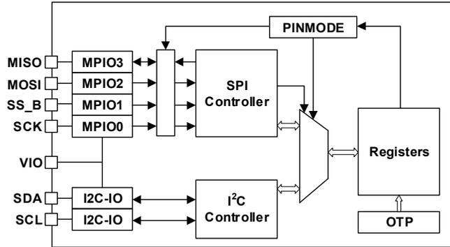
Figure 12. SPI and I<sup>2</sup>C Interface Block Diagram
