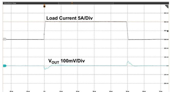
Figure 7. Load Transient of Buck1 at  $V_{IN} = 5V$
