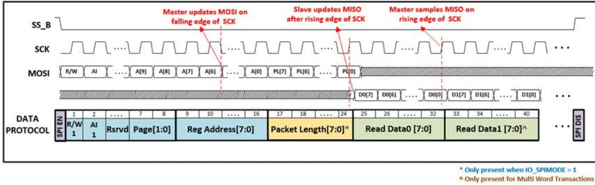
Figure 14. SPI Read Transaction with IO\_SPIMODE = 1; IO\_SPICPOL = 0; IO\_SPICPHA = 0
