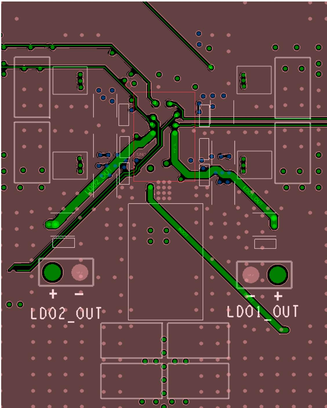
Figure 37. PCB Example 2, Inner Layer Showing LDO1-2 and  $V_{OUT}$  Sensing Traces
