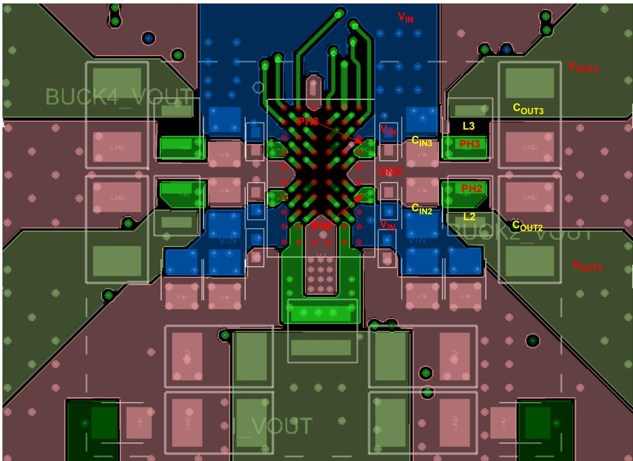
Figure 27. PCB Top Layer Buck Component Placement
