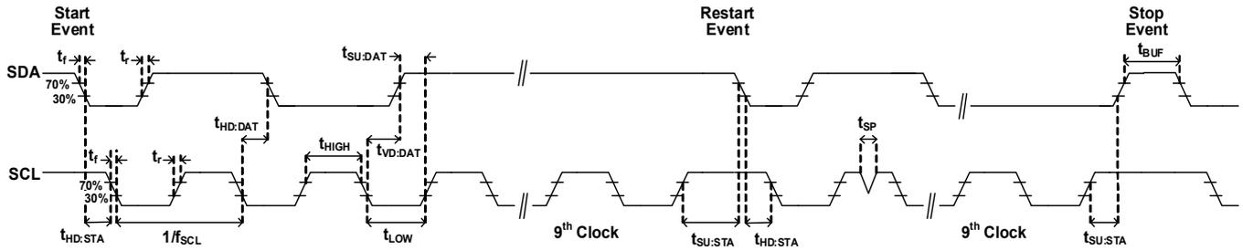
Figure 19. I<sup>2</sup>C Timing
