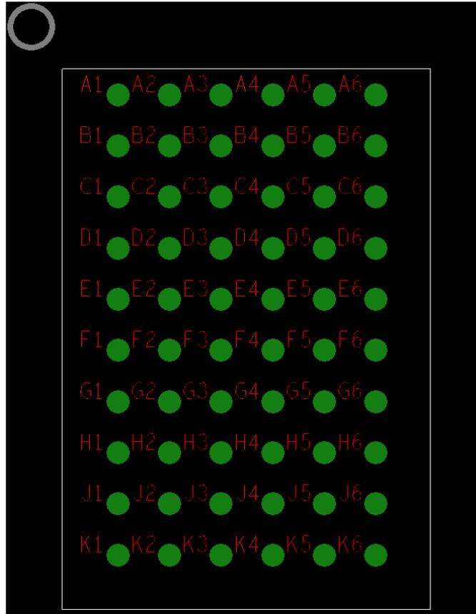
Figure 23. RAA271000 PCB Footprint (Top View)
