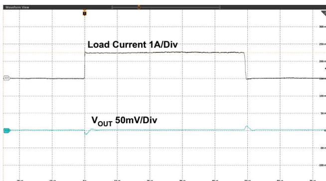
Figure 8. Load Transient of Buck2 at  $V_{IN} = 5V$
