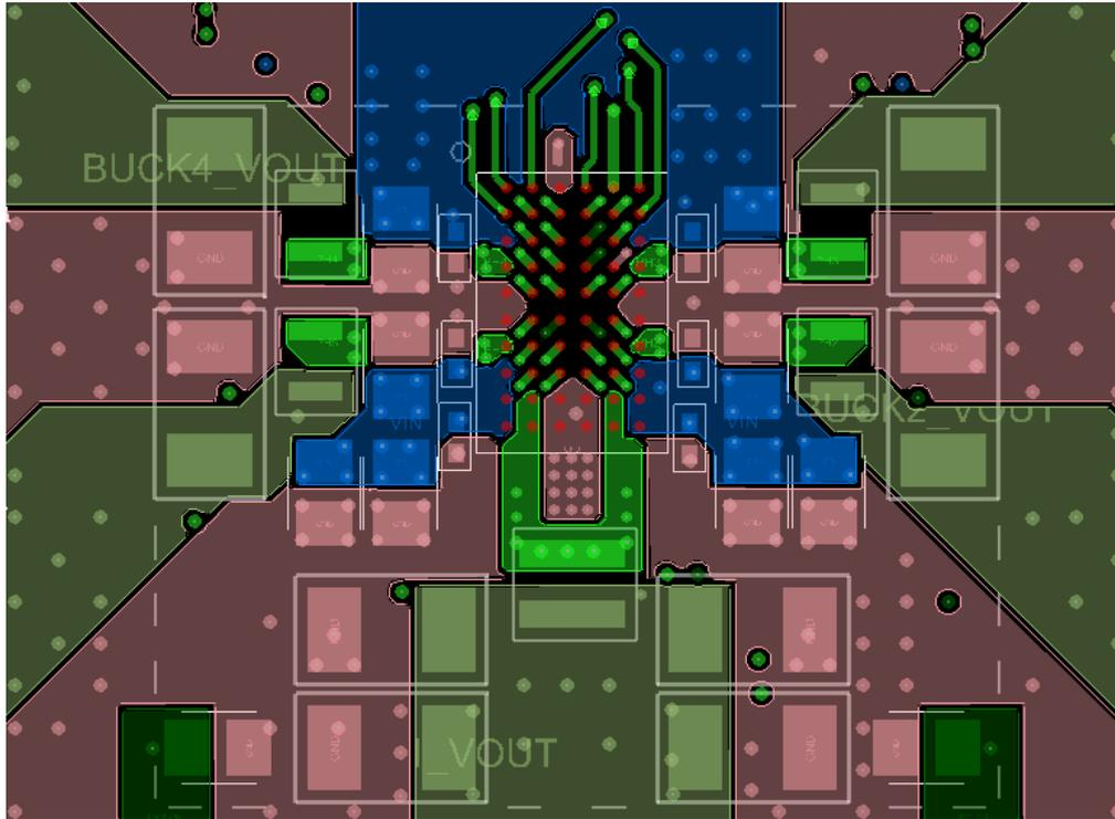
Figure 30. PCB Top Layer with All Components
