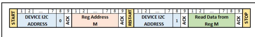
Figure 18. 1-Byte Data Read from Register M
