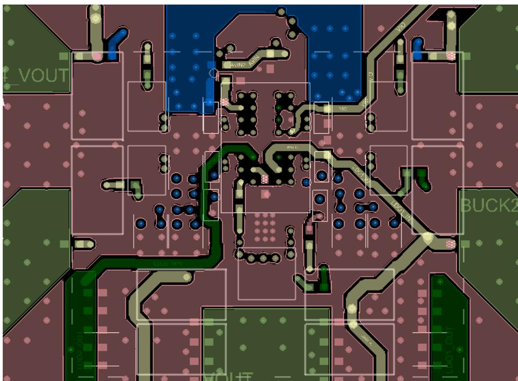
Figure 33. PCB Bottom Layer and Bootstrap Capacitor Connection
