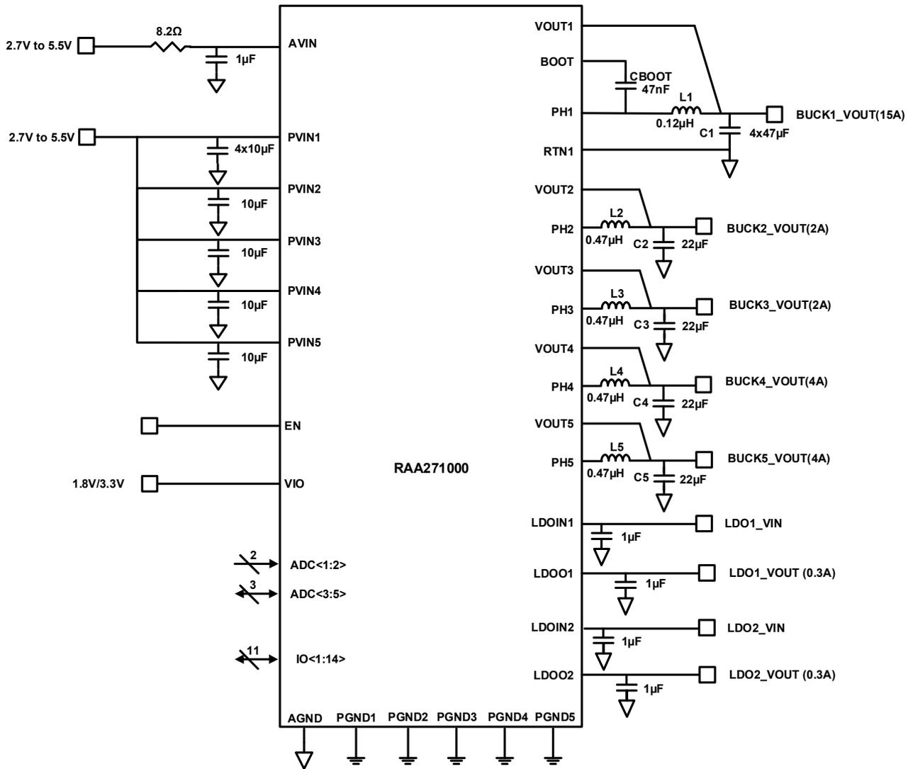
Figure 2. Typical Application Diagram
