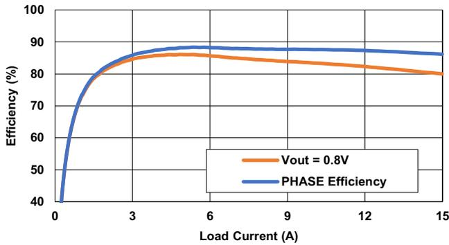
Figure 4. Efficiency of Buck1 at  $V_{IN} = 5V$
