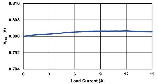
Figure 5. Load Regulation of Buck1 at  $V_{IN} = 5V$
