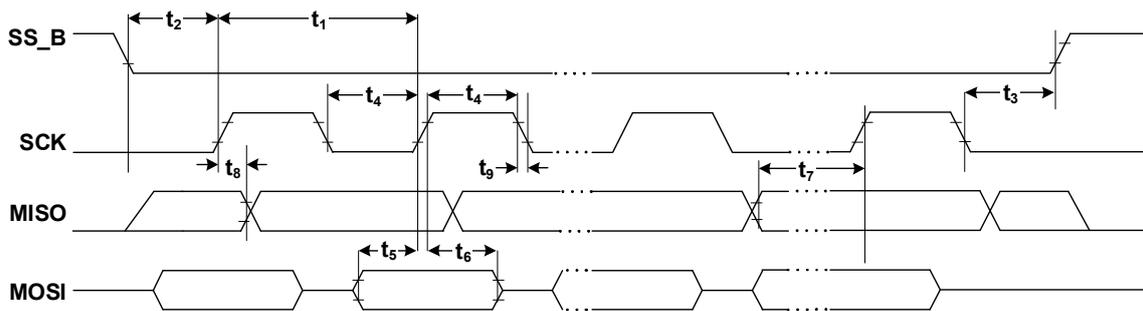
Figure 16. SPI Timing for IO\_SPICPHA = 0, IO\_SPICPOL = 0
