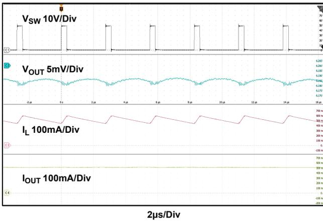
Figure 5. Buck Output Ripple at Full Load
