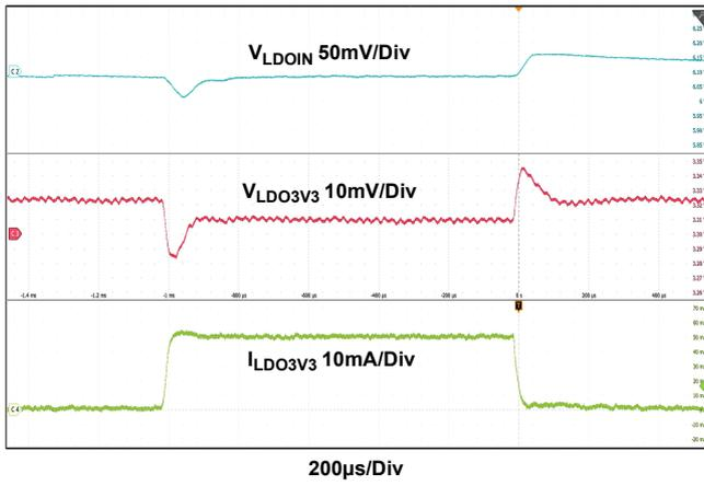
Figure 21. VLDO3V3 Load Transient between 0A to 0.05A
