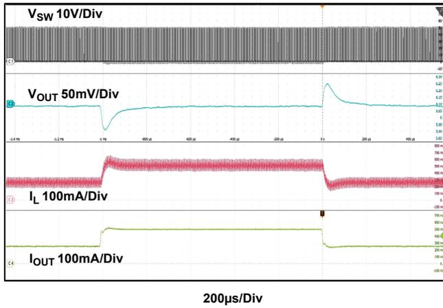
Figure 9. Load Transient between 0.25A to 0.5A
