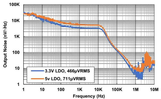
**Figure 28. Output Noise vs Frequency**
