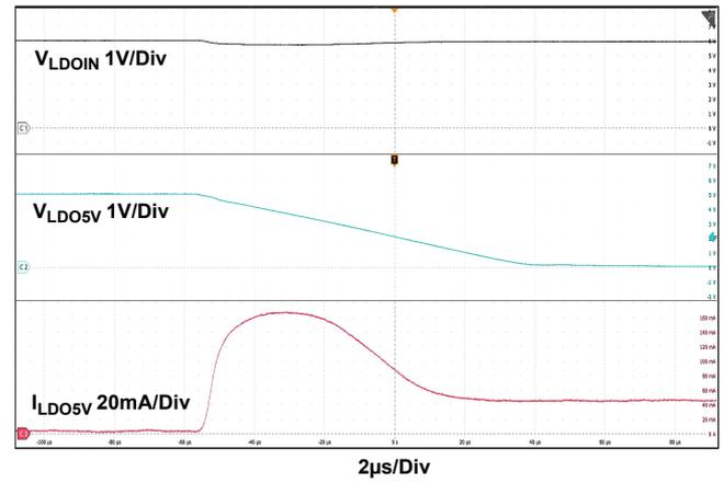
Figure 24. VLDO5V OCP Fault with Current Foldback
