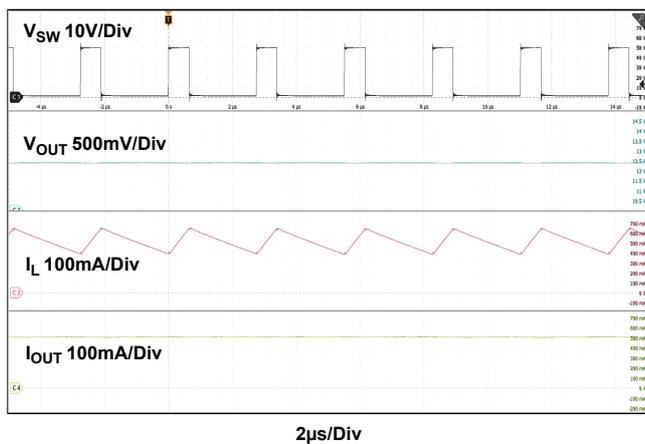
Figure 13. Buck Output Ripple at Full Load
