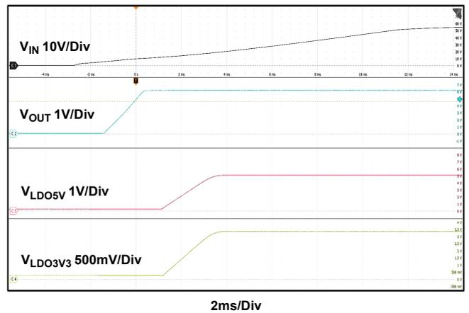
Figure 8. Power-On at Full Load with LDO Channels
