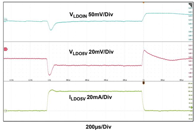
Figure 22. VLDO5V Load Transient between 0A to 0.1A
