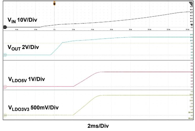
Figure 16. Power-On at Full Load with LDO Channels
