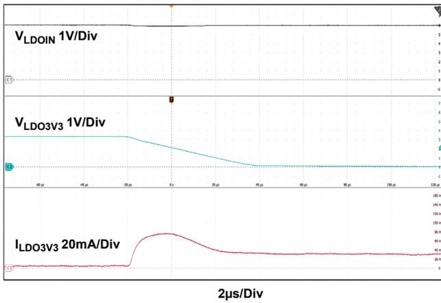
Figure 23. VLDO3V3 OCP Fault with Current Foldback
