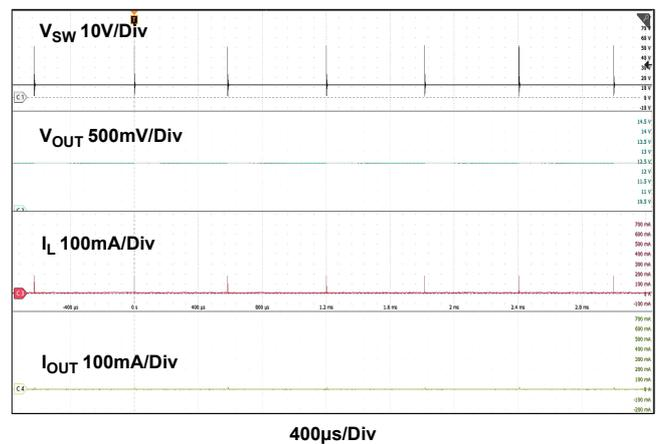
Figure 14. Buck Output Ripple at No Load
