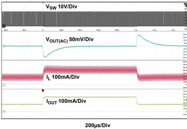
Figure 17. Load Transient between 0.25A to 0.5A
