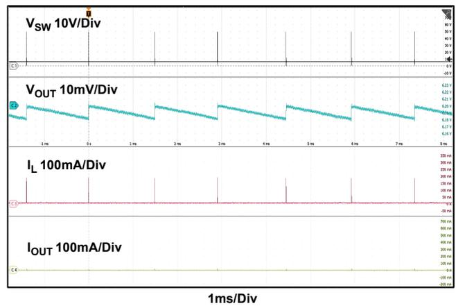
Figure 6. Buck Output Ripple at No Load
