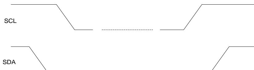
**Figure 36: Timing of the START and STOP Conditions**
