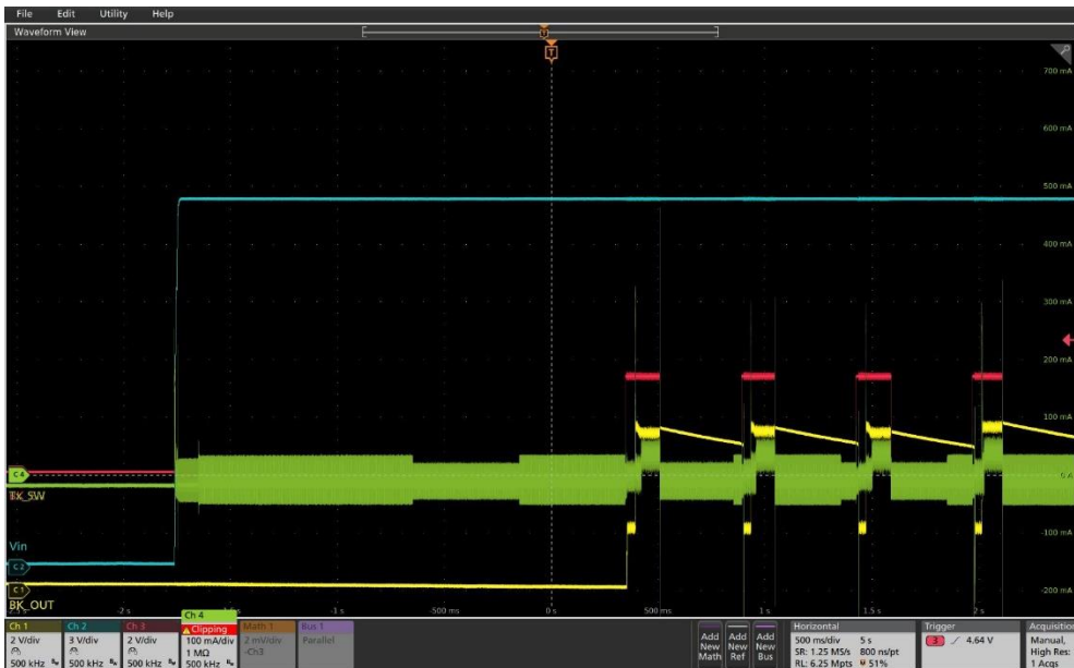
Figure 9. 19V Fixed Voltage Adaptor Start-up: Ch1 = VBRIDGE, Ch2 = Vin, Ch3 = GPIO_B4, Ch4 = I IN
