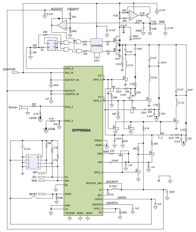
Figure 1. IDTP9036A Simplified Application Schematic
