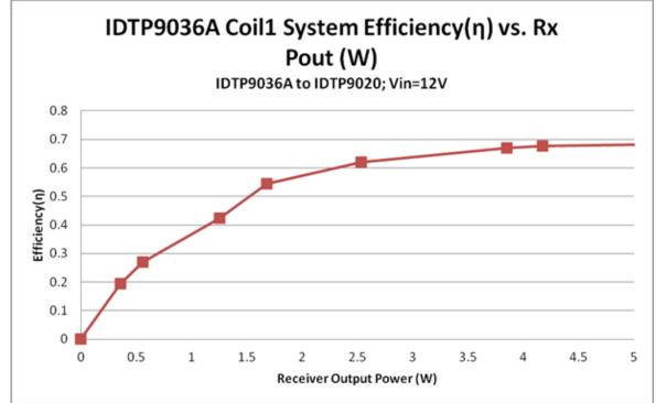
Figure 3. Efficiency vs. RX Output Power with Left Coil #1
