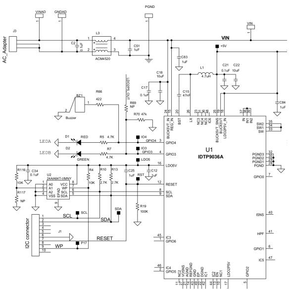
Figure 11a. Input power, LDO5V, LEDs, buzzer, and I<sup>2</sup>C
