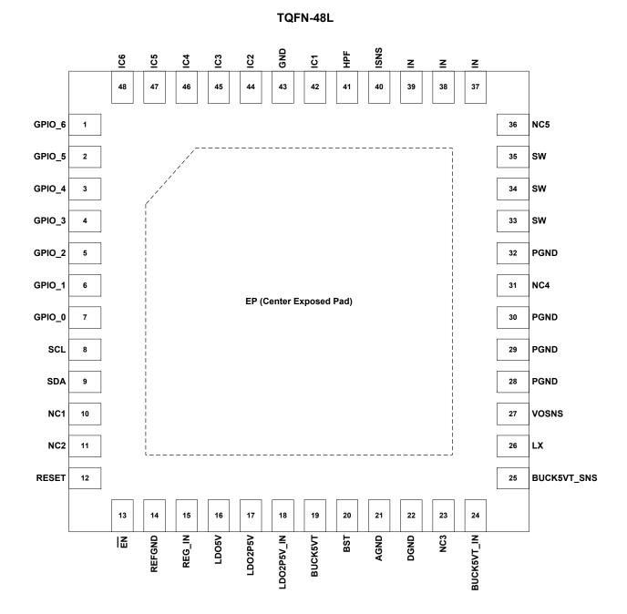
Figure 2. IDTP9036A Pin Configuration (NTG48 TQFN-48L 6.0 mm x 6.0 mm x 0.75 mm, 0.4mm pitch)
