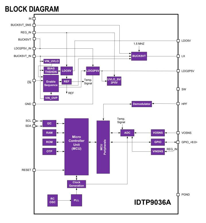
Figure 7. IDTP9036A Internal Functional Block Diagram
