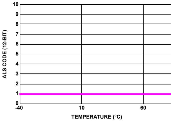
FIGURE 14. STABILITY OF ALS COUNT OVER-TEMPERATURE (AT 0.00 LUX)
