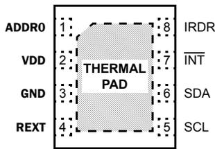
\*THERMAL PAD CAN BE CONNECTED TO GND OR ELECTRICALLY ISOLATED
