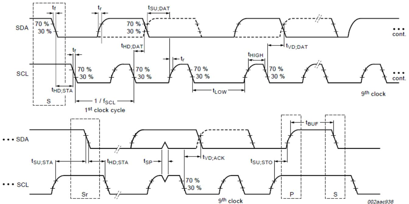
FIGURE 1. I<sup>2</sup>C TIMING DIAGRAM
