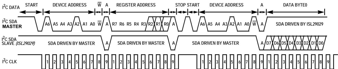
**FIGURE 2. I<sup>2</sup>C DRIVER TIMING DIAGRAM FOR MASTER AND SLAVE CONNECTED TO COMMON BUS**
