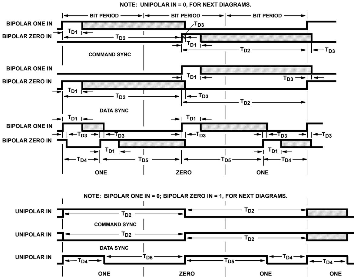
FIGURE 12. DECODER TIMING
