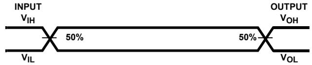
AC Testing: All input signals must switch between  $V_{IL}$  and  $V_{IH}$ . Input rise and fall times are driven at 1ns per volt.
