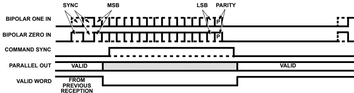
FIGURE 5. DECODER TIMING
