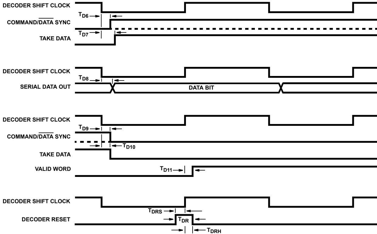
FIGURE 11. DECODER TIMING
