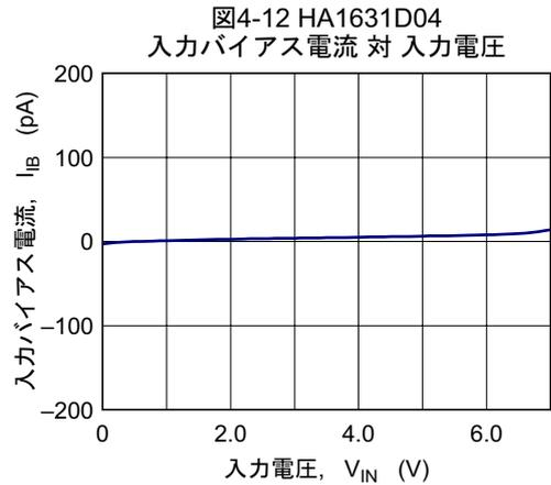
(特記なき場合,  $V_{DD} = 3V, V_{SS} = 0V, T_a = 25^\circ C$ )
