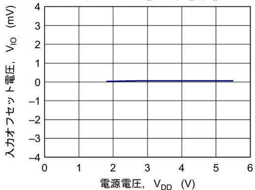
(特記なき場合,  $V_{DD} = 3V, V_{SS} = 0V, T_a = 25^\circ C$ )
