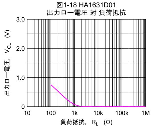
(特記なき場合,  $V_{DD} = 3V, V_{SS} = 0V, T_a = 25^\circ C$ )
