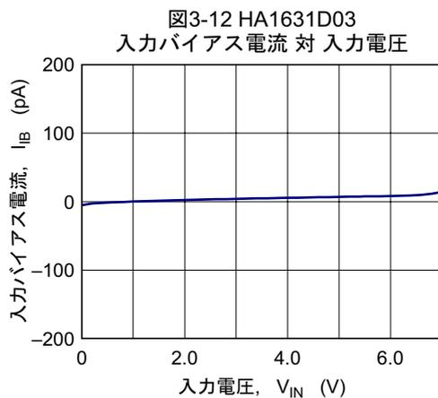
(特記なき場合,  $V_{DD} = 3V, V_{SS} = 0V, T_a = 25^\circ C$ )
