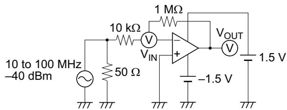
$$A_V = \left| 20 \log_{10} \frac{101 \times |V_{OUT}|}{|V_{IN}|} \right|$$
