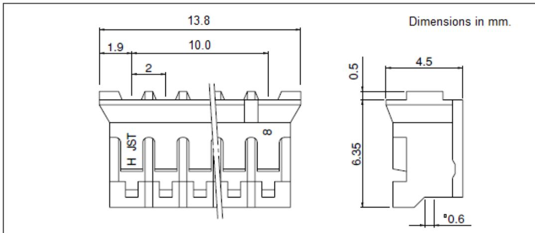
Figure 8. Receptacle Drawing
