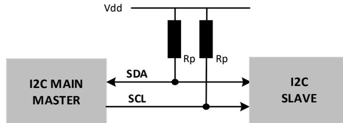
Figure 3. I<sup>2</sup>C Master-Slave Configuration
