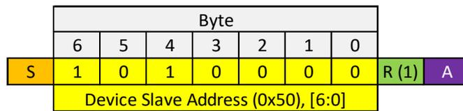
Figure 5. Flow Data Read Command
