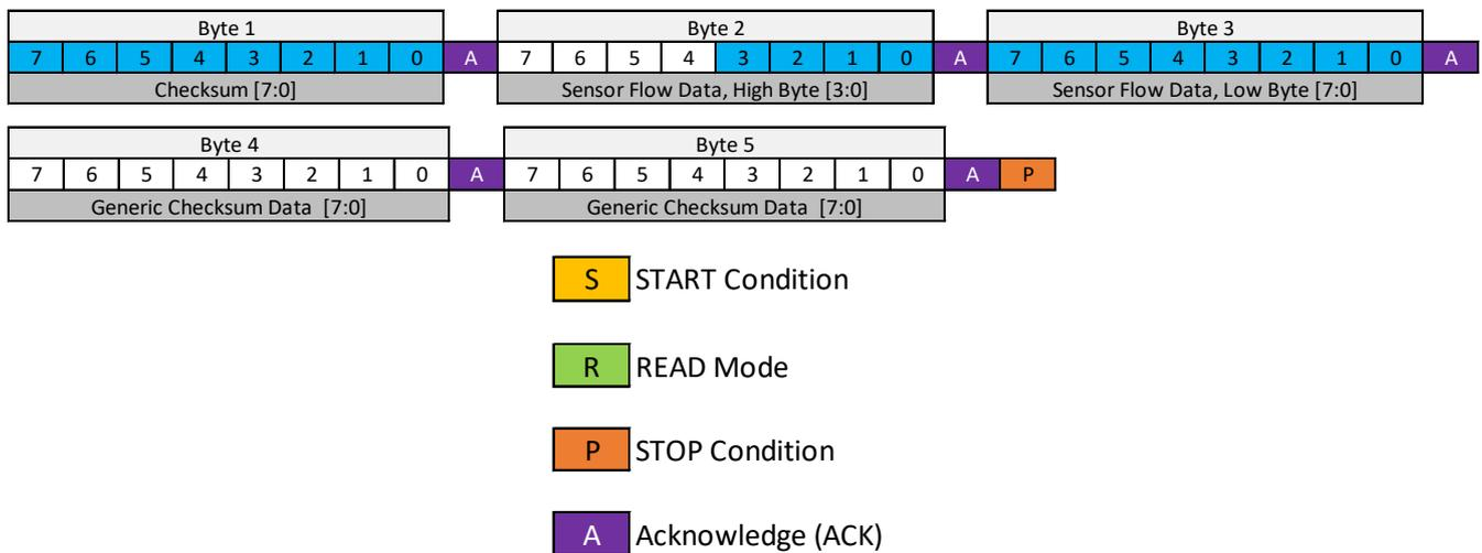
Figure 7. Flow Data from FS1023-DG
