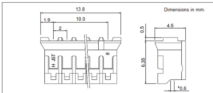
Figure 8. Receptacle Drawing
