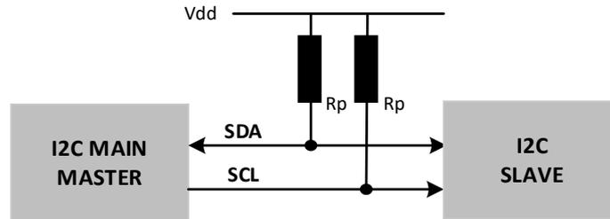
Figure 4. I<sup>2</sup>C Master-Slave Configuration
