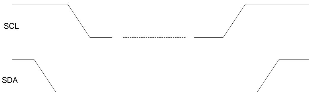
Figure 21: I 2 C START and STOP Condition Timing
